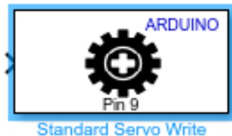
Figure 9.3 – Servo write block used to control motors.
