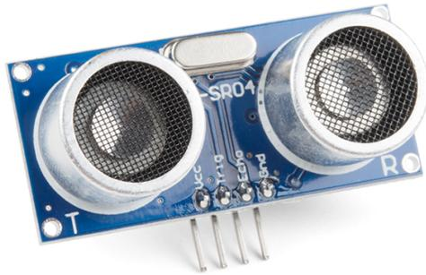
Figure 8.6 – HC-SR04 ultrasonic sensor which is used to provide altitude readings to the flight controller.
