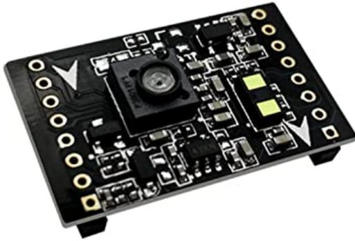
Figure 8.7 – PMW3901 Optical Flow Sensor.
