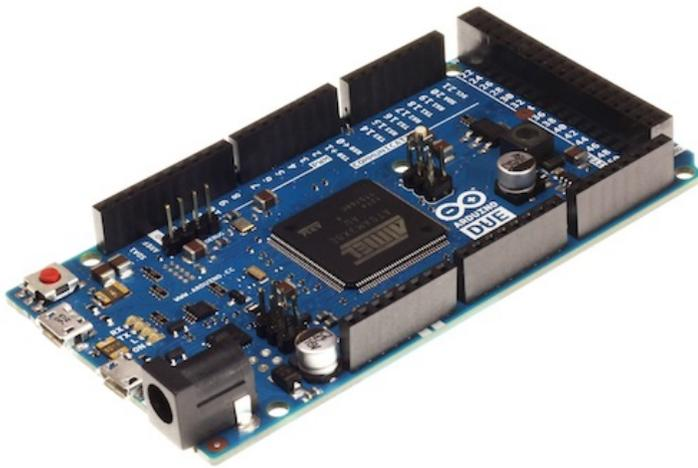
Figure 8.1 – Arduino Due used as the flight controller for this project.
