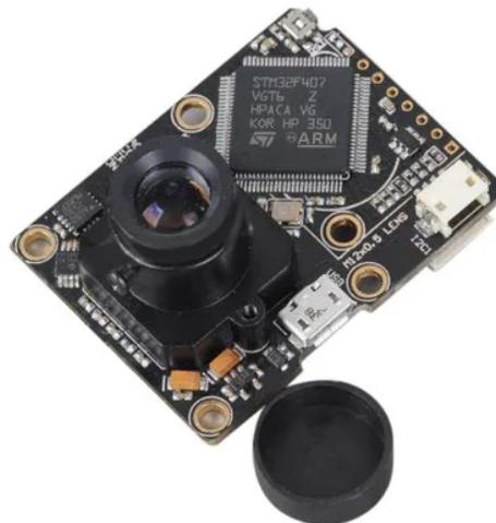
**Figure 16. PX4FLOW module**
