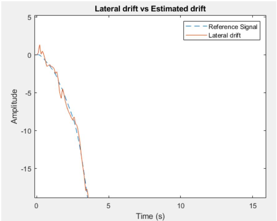
Figure 23: KF true vs estimated lateral drift (m)
