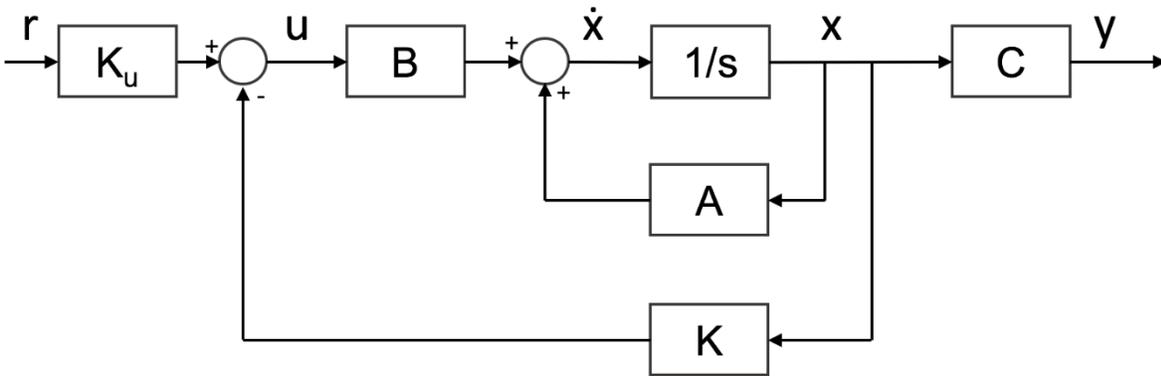
Figure 13: LQR block diagram [7]
