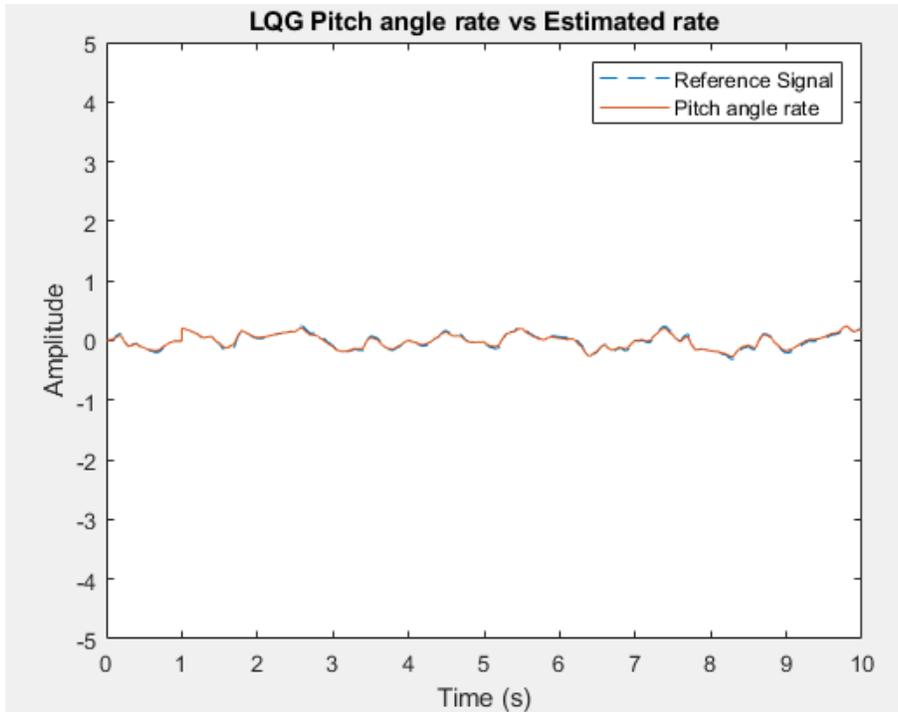
Figure 28: LQG estimate vs true angle rate (deg)
