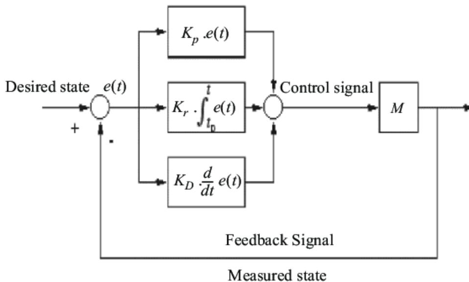
Figure 10: PID block diagram [6]
