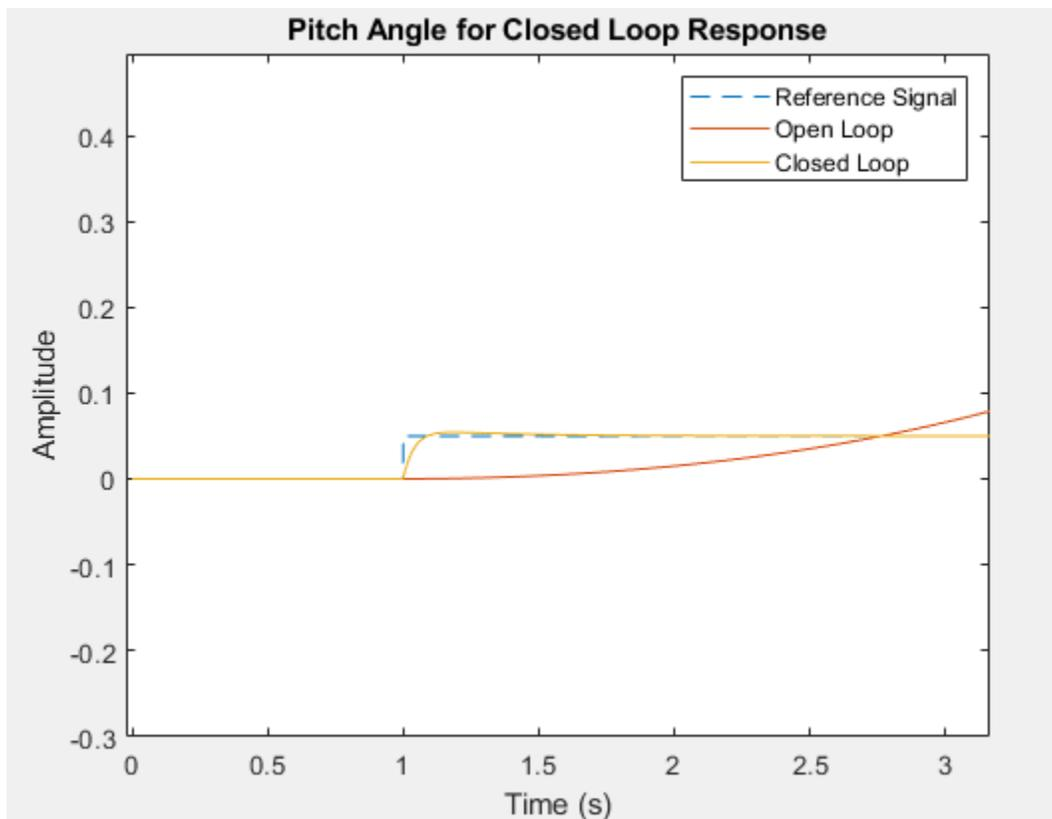
Figure 12: Closed loop PID controlled response
