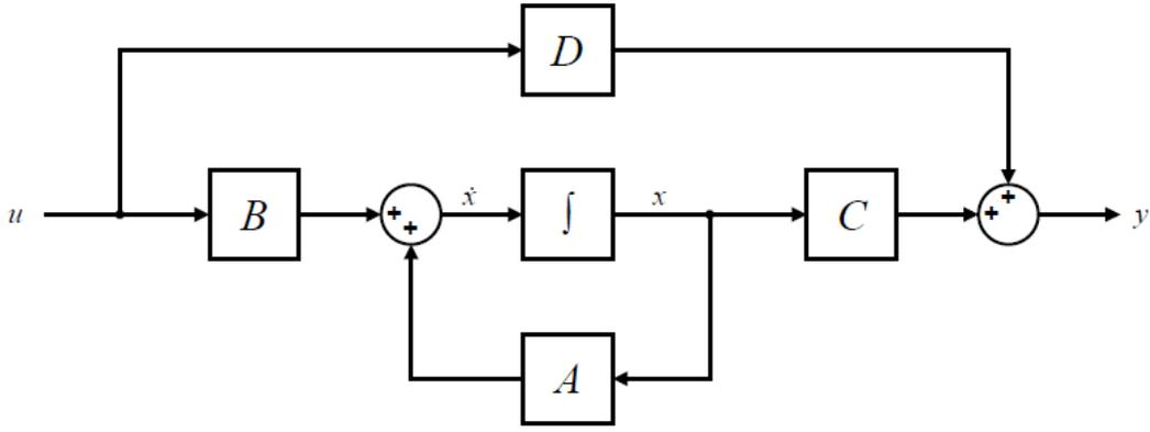
Figure 6: State space block diagram [20]
