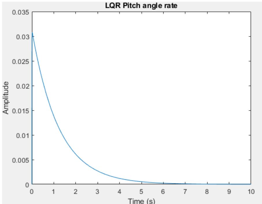
Figure 15: LQR pitch angle rate (deg/s)
