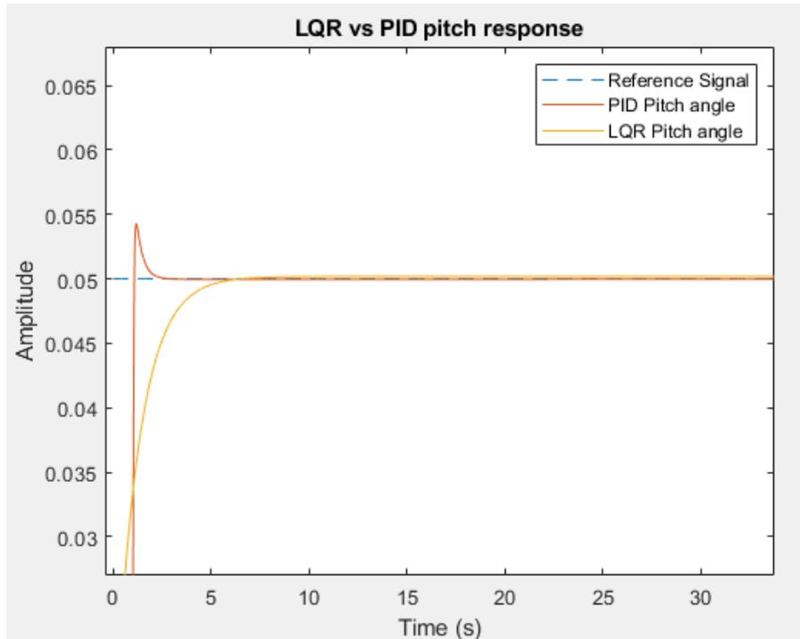
Figure 18: LQR vs PID controller pitch response comparison (deg)
