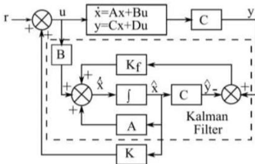
Figure 25: LQG detailed block diagram [11]
