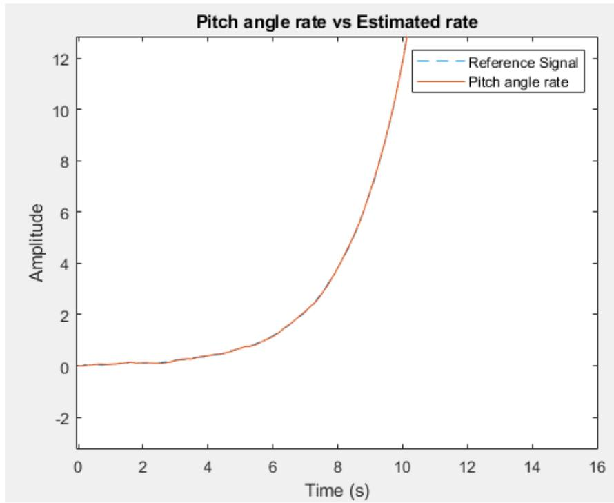
Figure 22: KF true vs estimated angle rate (deg/s)
