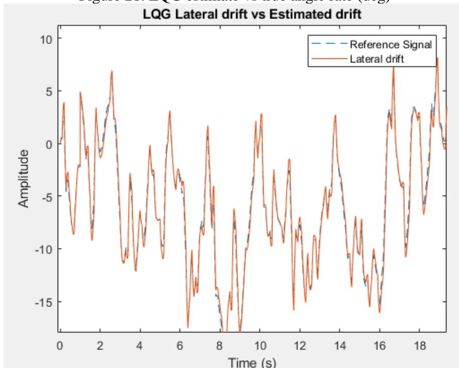
Figure 29: LQG estimated vs true lateral drift (m)
