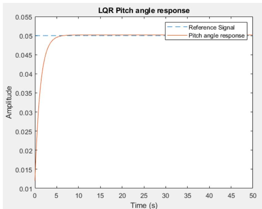
Figure 16: LQR pitch angle response (deg)
