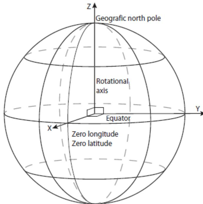
Figure 3: Earth centered inertial reference frame [1]
