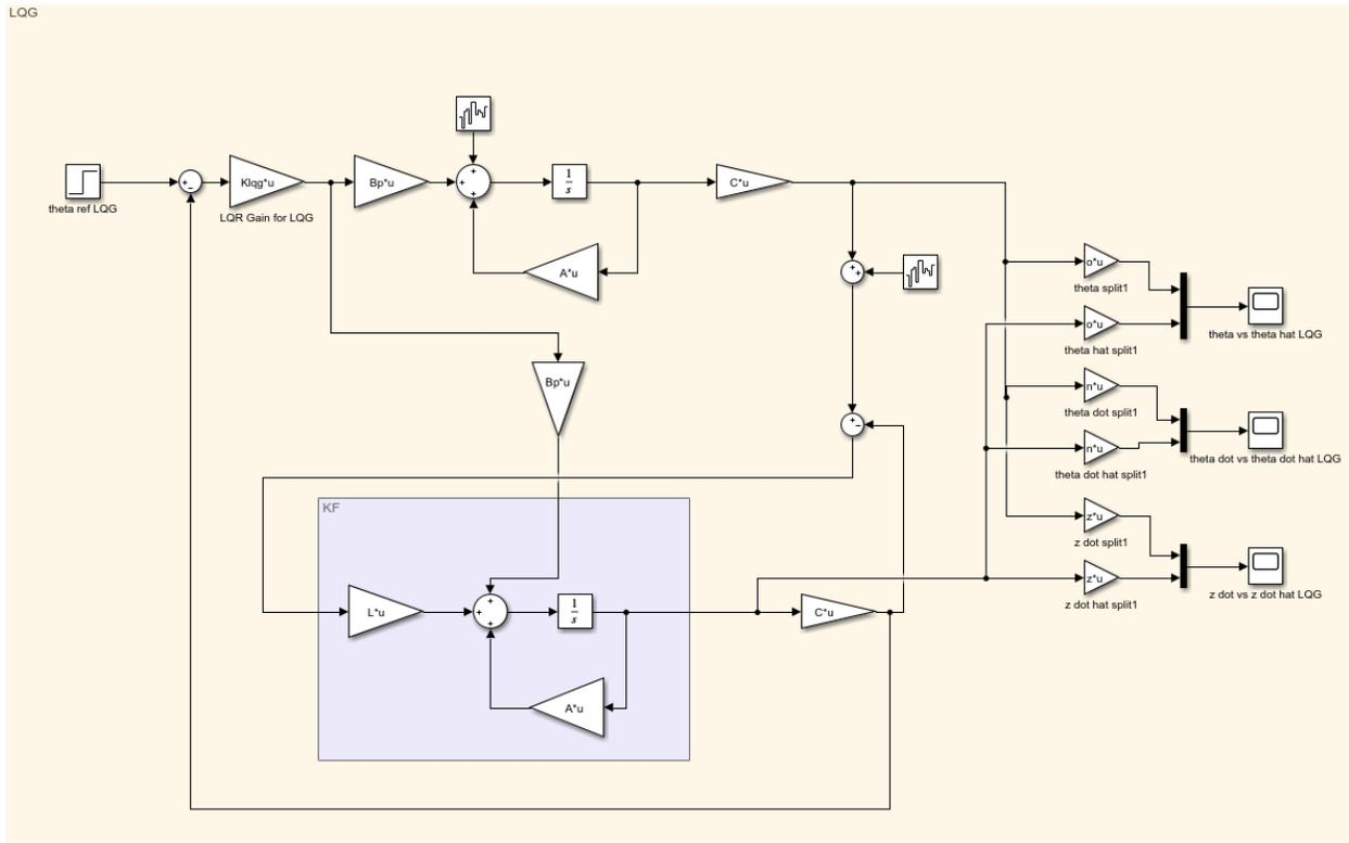
Figure 26: LQG Simulink block diagram
