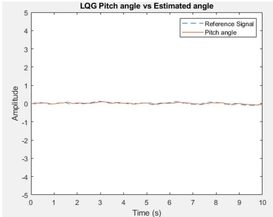
Figure 27: LQG estimated vs true angle (deg)
