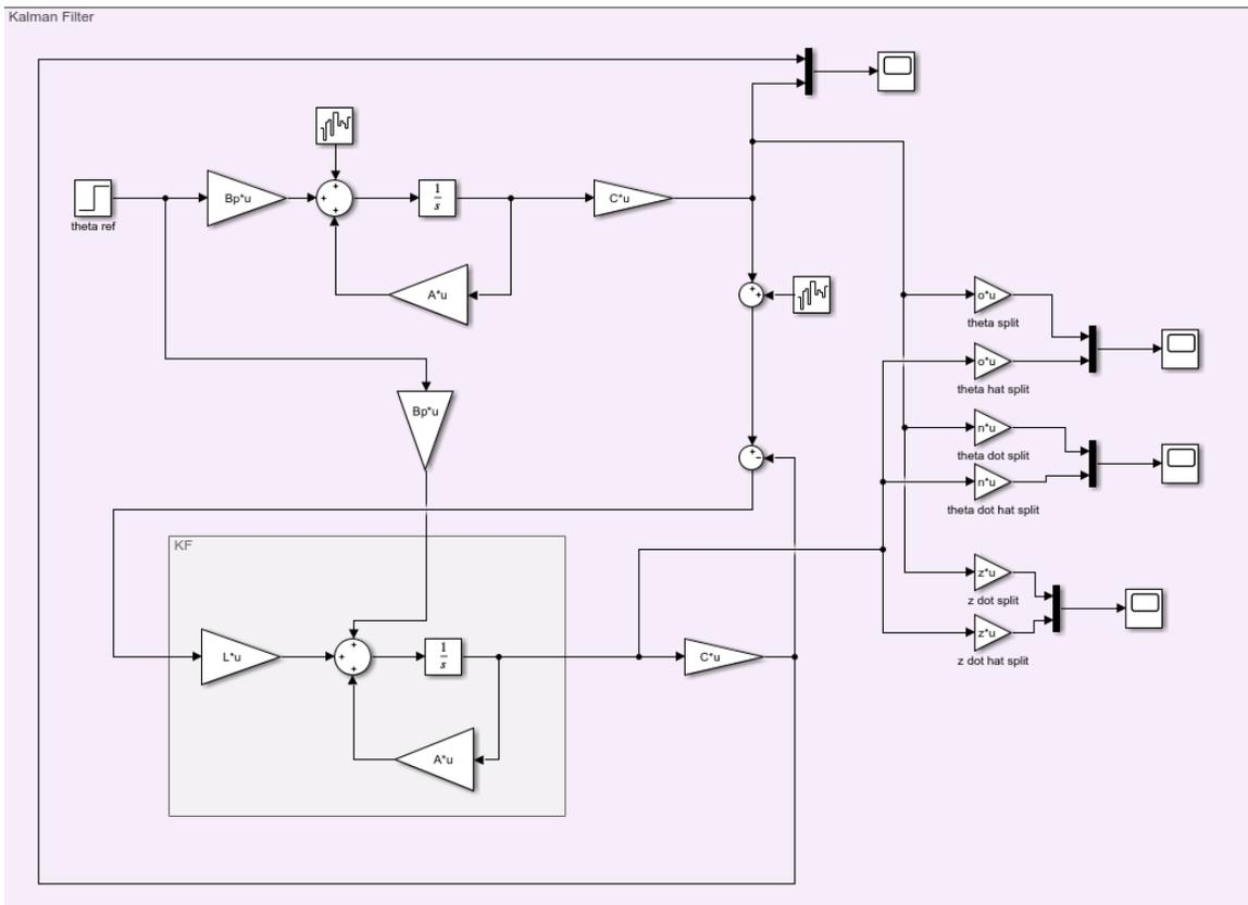
Figure 20: Simulink kalman filter diagram
