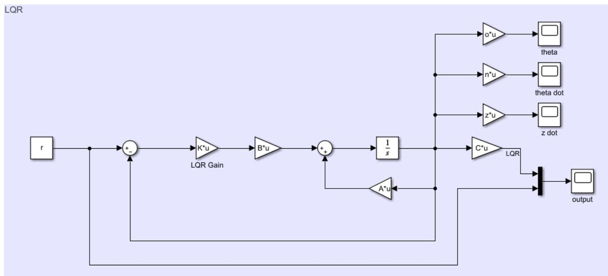
Figure 14: LQR SIMULINK block diagram
