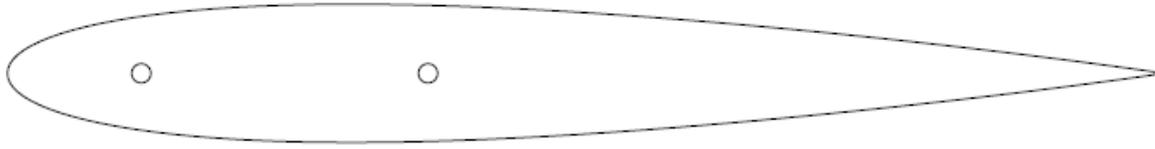
Figure 9.2 – NACA 0012 airfoil
