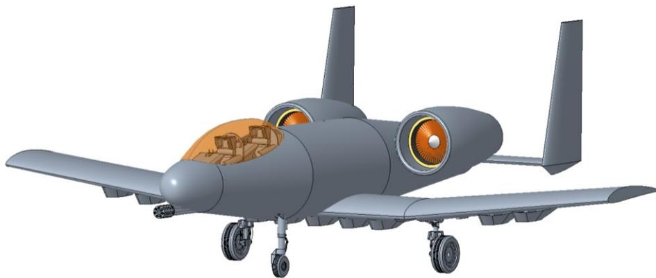
Figure 10.10 – YA-94 with landing gear fully integrated (deployed)
