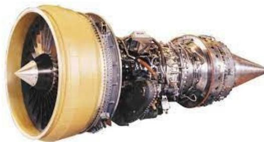
Figure 6.2 – General Electric CF34-8C5B1 turbofan engine
