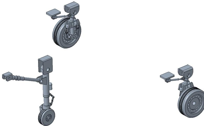
Figure 10.1 – Landing gear design layout
