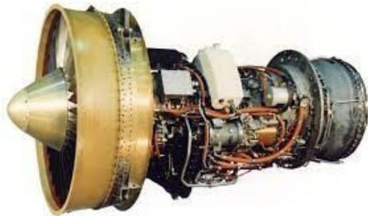
Figure 6.1 – General Electric TF34-GE-100A turbofan engine
