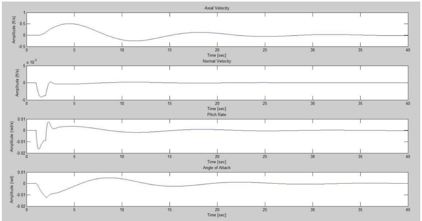
Figure 5: Response to +1 deg. step elevator input
