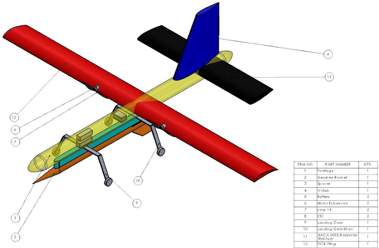
Figure 14: Preliminary layout of the Airplane
