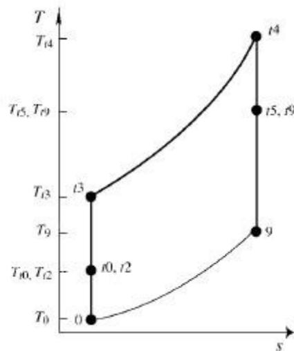
**Figure 4. T-s diagram for an ideal turbojet**
