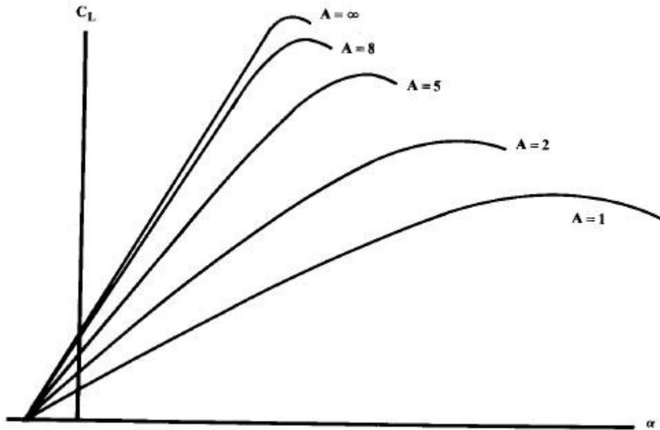
Figure 2. Effect of aspect ratio on lift
