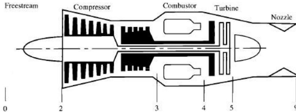
**Figure 3. Station numbering for an ideal turbojet**
