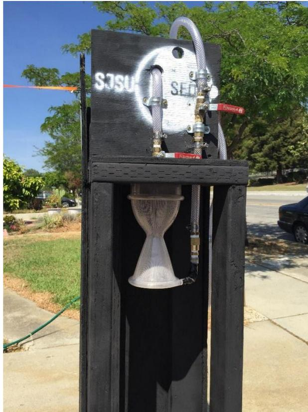
**Figure 33a: SEDS SJSU Hydro Flow Test Stand**
