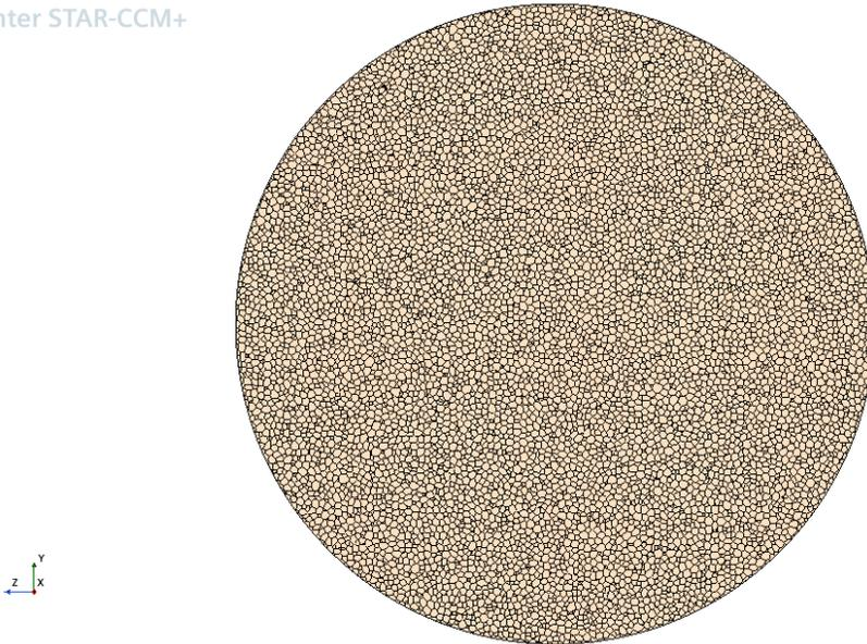
Figure 3.9 – Cross section of the thruster mesh in the y-z plane.
