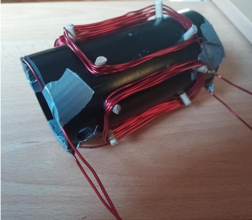
Figure 4.7 – Perspective view of the RMF coil array.
