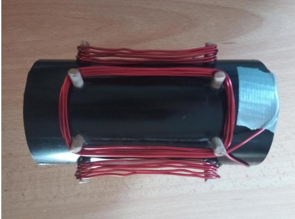
Figure 4.5 – Top view of the RMF coil array.
