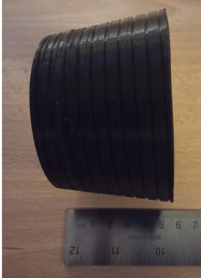
Figure 5.2 – 3D printed axial coil scaffold.
