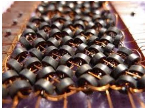
**Figure 1. Iron core rope memory**
