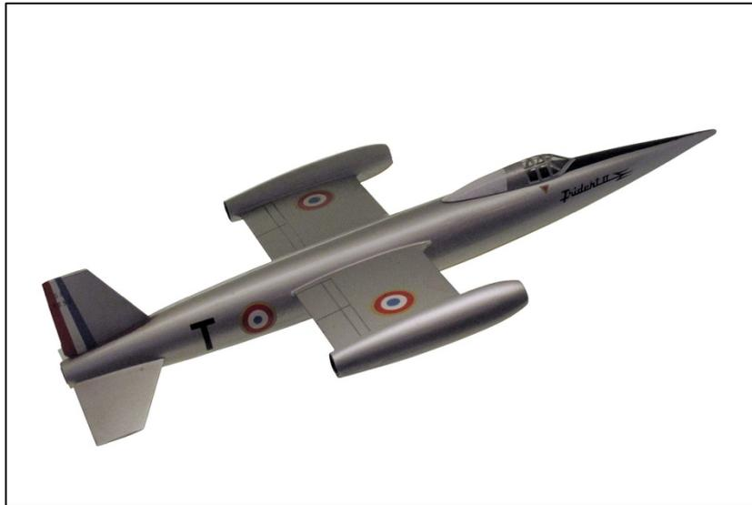
Figure 2.0.8 – Trident II with Turbomeca Gabizo and SEPR 631 engine
