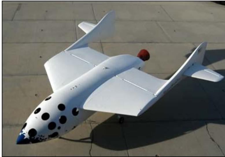
Figure 2.0.6 – Top view of SpaceShipOne with rocket nozzle
