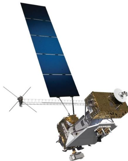
Figure 1.7 - LCRD on the STPSat-6 spacecraft [2]
