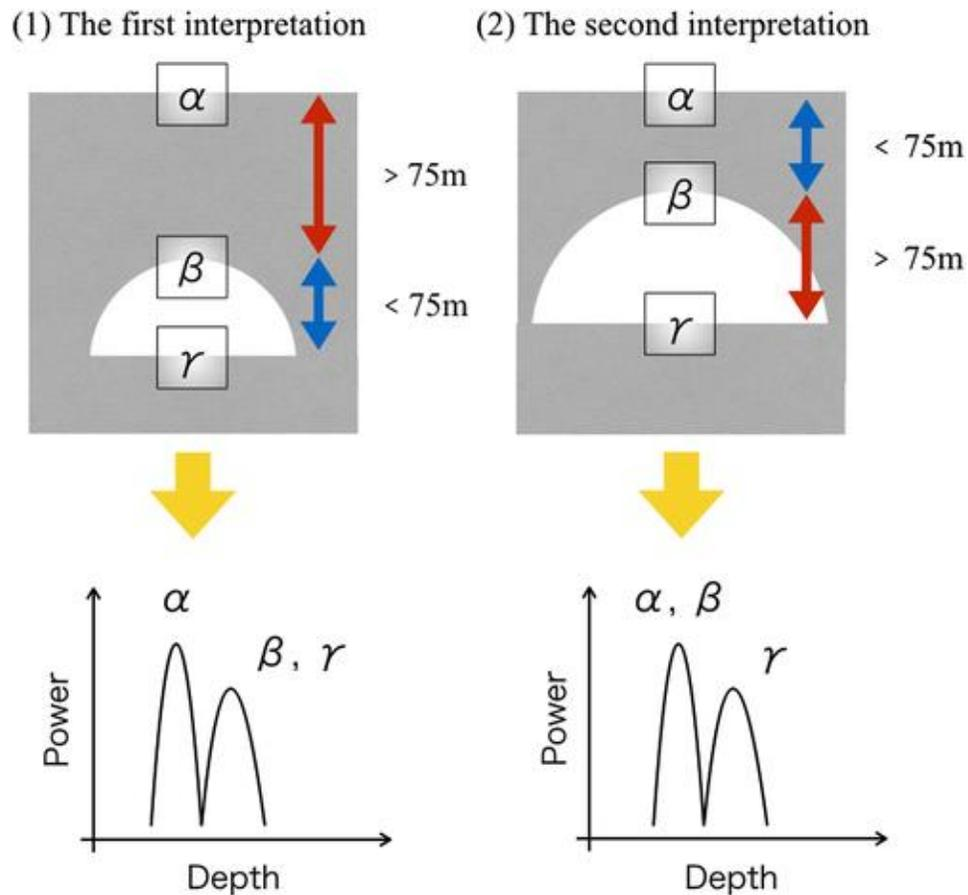
Figure 3.8 - Radar echo data results indicating location and depth of lava tube [50]
