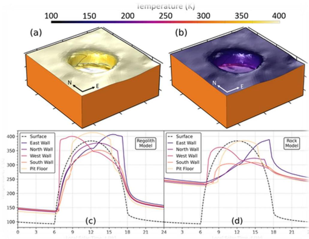
Figure 2.6 - 3D thermal model of a lunar pit made by UCLA researchers [43]
