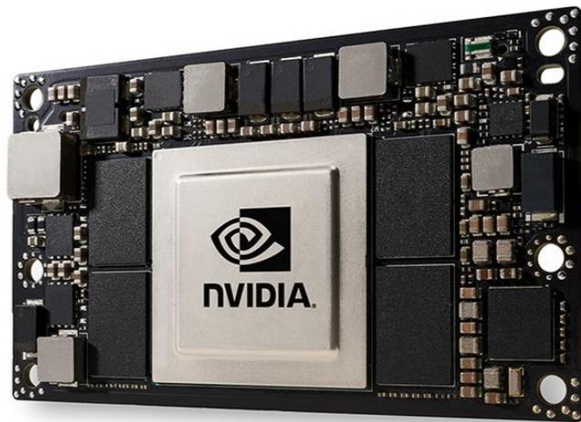
Figure 3.6 – NVIDIA Jetson TX2 module [48]
