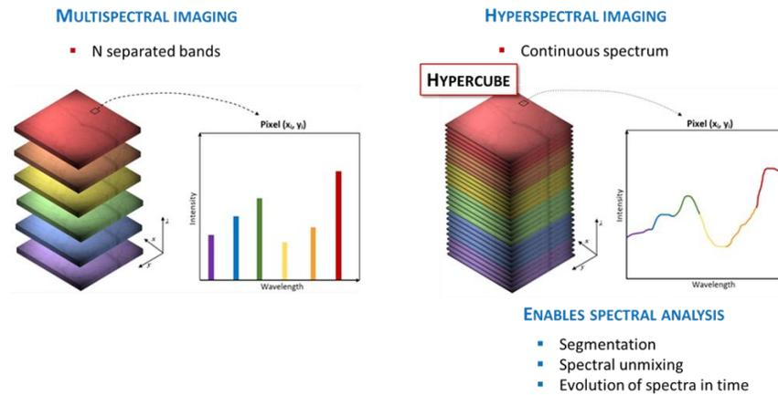
Figure 1.6 - A diagram illustrating how hyperspectral imagery works [20]
