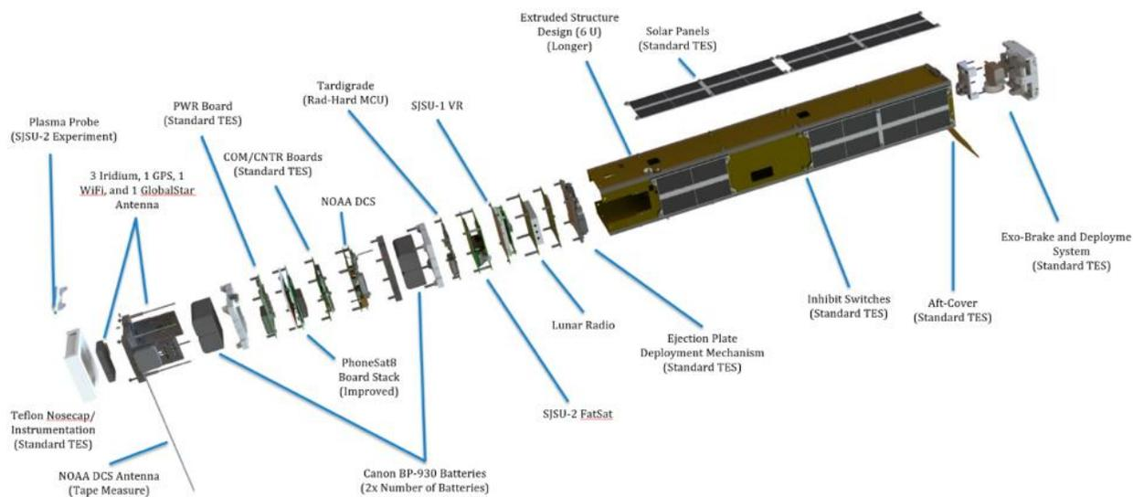
Figure 2.3 - Isometric view of *TechEdSat-8* [16]
