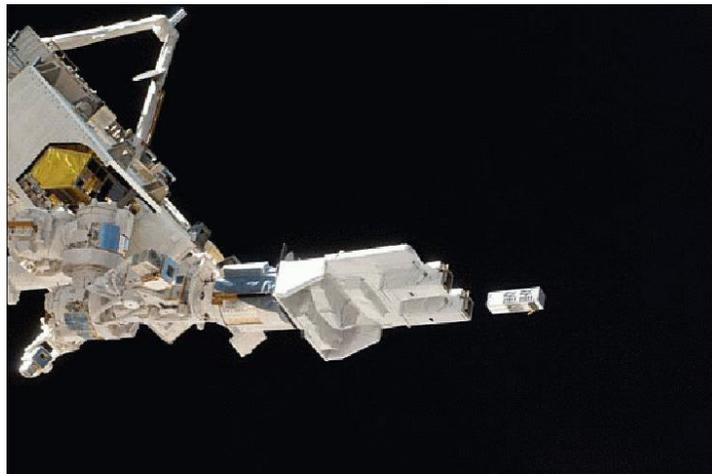
Figure 1.5 - *TechEdSat-1* being deployed from the ISS [16]
