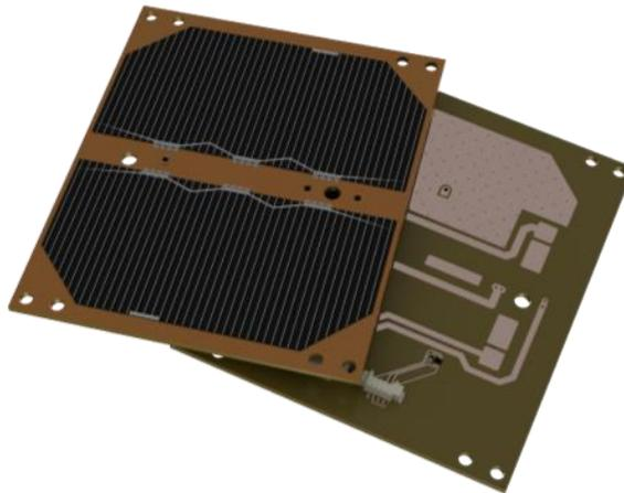
Figure 3.5 – Type of solar panel typically used on CubeSats [47]
