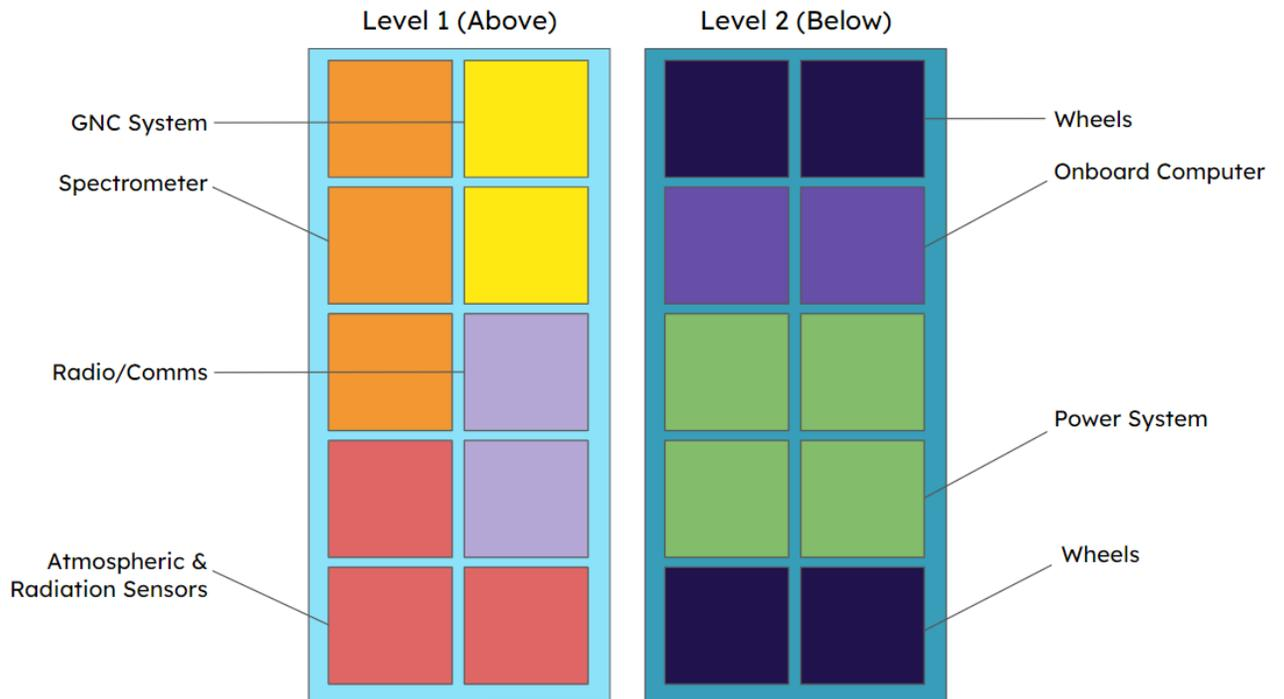
Figure 7.1 - Proposed locations of each subsystem on the CubeSat rover
