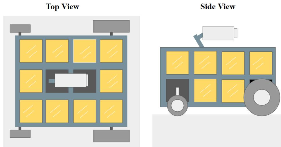
Figure 3.1 - Preliminary mockup of the CubeSat rover with spectrometer
