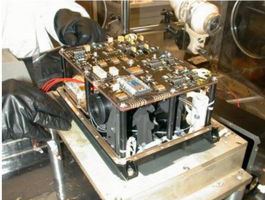
Figure 4.1 - Mini-TES spectrometer in development [51]
