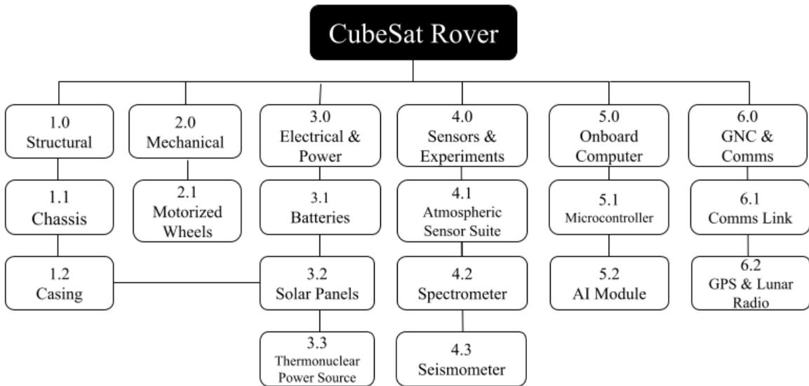
Figure 3.3 – Subsystem breakdown of CubeSat rover
