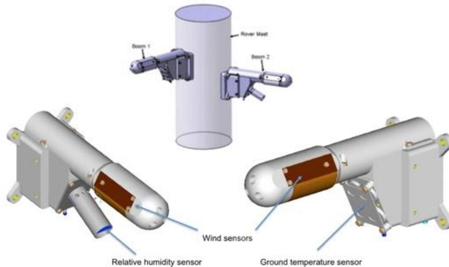
Figure 4.3 - REMS sensor suite for Mars rovers [54]
