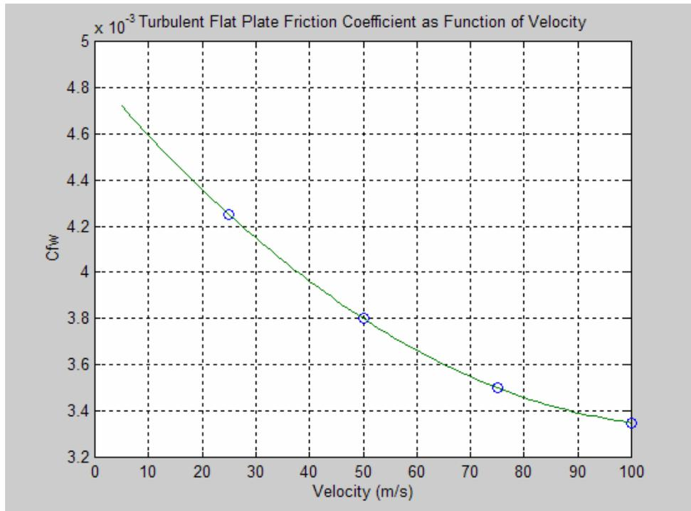
**Figure 18: Turbulent Flat Plate Friction Coefficient as Function of Velocity (Nordin, 2006)**
