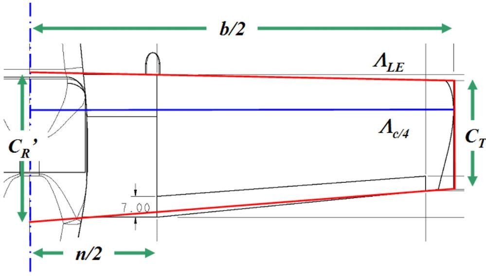
**Figure 40: Equivalent wing planform (Nordin, 2006)**
