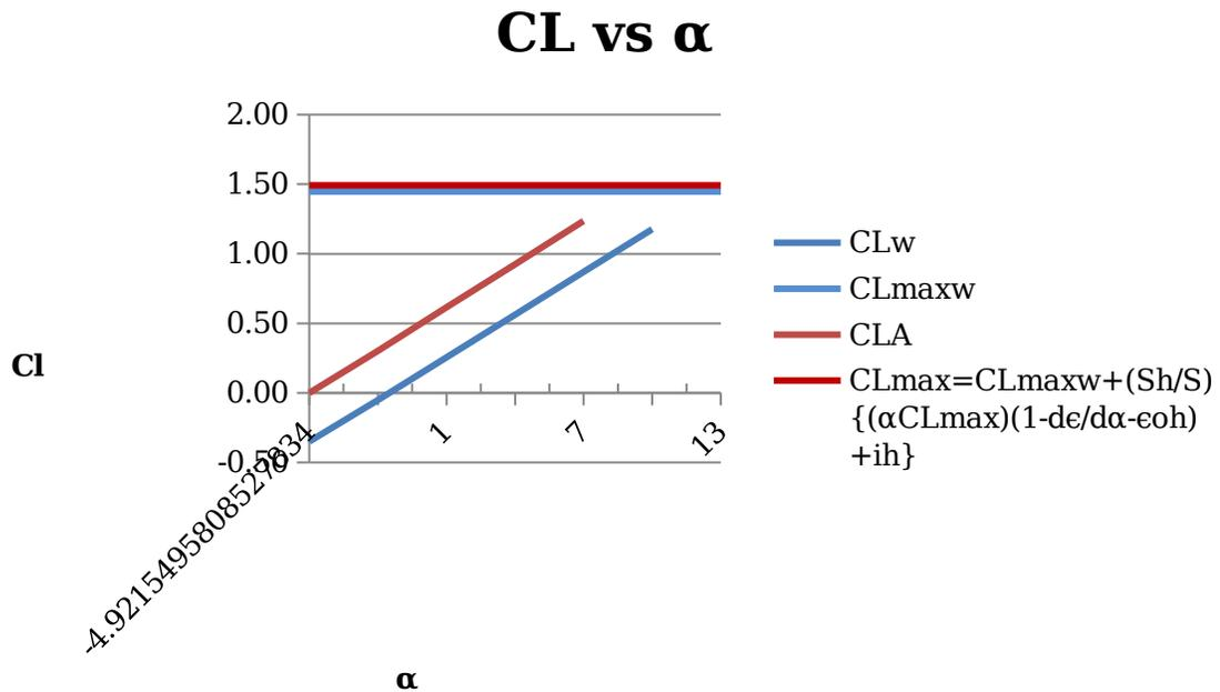
**Figure 17: Airplane and wing lift vs. alpha curves**
