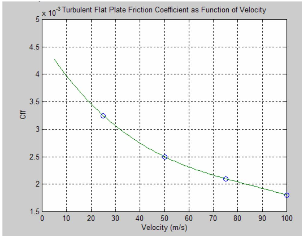
**Figure 19: Fuselage Turbulent Flat Plate Friction Coefficient as Function of Velocity (Nordin, 2006)**
