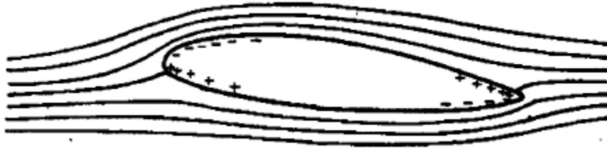
**Figure 9: Fuselage in Ideal Flow (Multhopp, 1942)**
