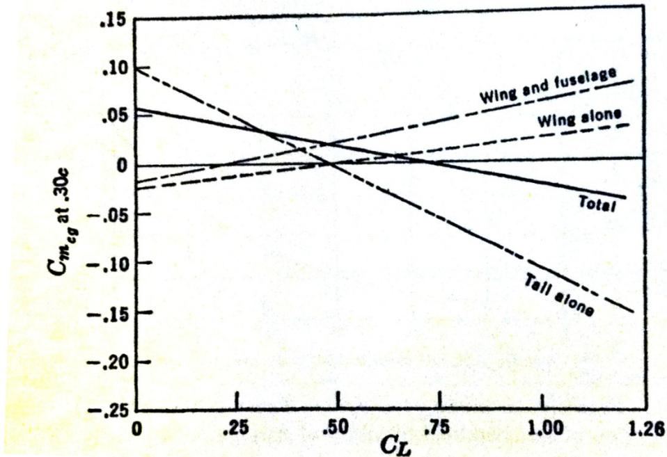
**Figure 10: Typical longitudinal stability breakdown (Perkins & Hage, 1949)**
