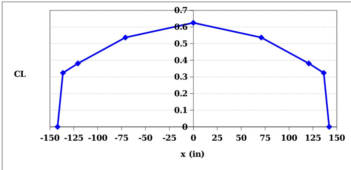
**Figure 14: Lift Coefficient Distribution for Level Flight (Nordin, 2006)**
