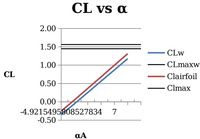
**Figure 16: Wing lift vs. angle of attack**
