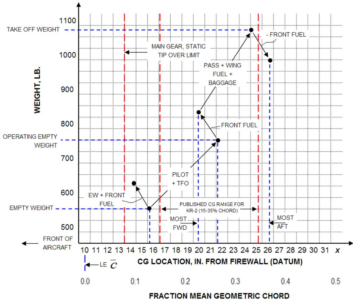
**Figure 24: Airplane center of gravity (c.g.) diagram**
