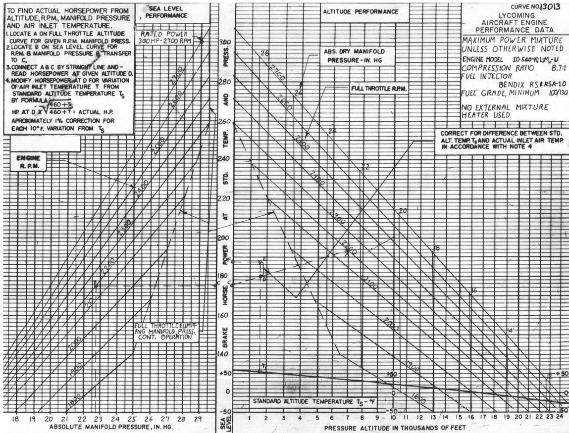
**Figure 2: Sea Level and Altitude Performance Curve - IO-540-K, -L, -M, -S (Lycoming)**
