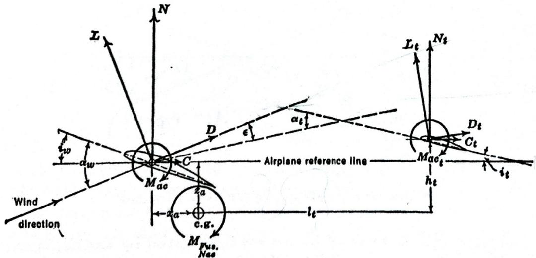
Figure 6: Forces and moments in plane of symmetry (Perkins & Hage, 1949)
