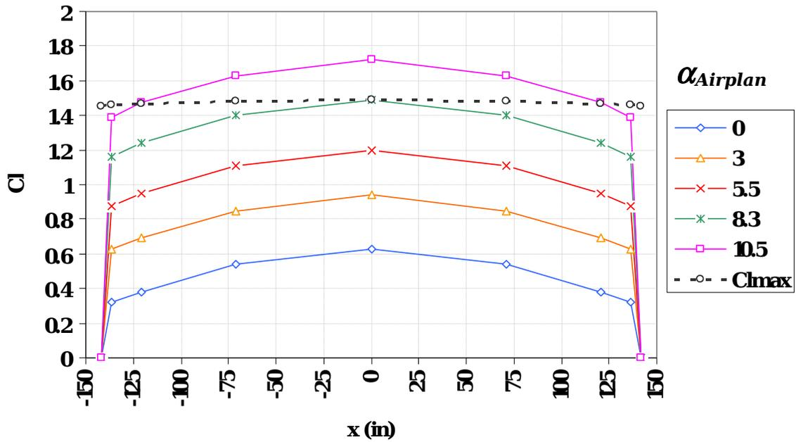
**Figure 15: Local wing lift coefficient distribution for varying angle of attack (Nordin, 2006)**
