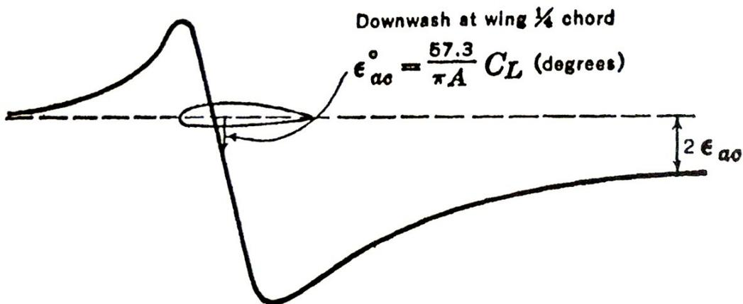
**Figure 8: Downwash distribution in front and behind a finite wing. (Perkins & Hage, 1949)**
