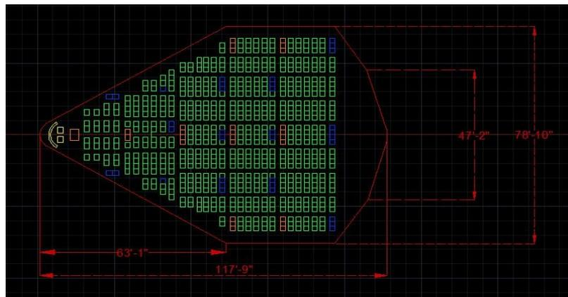
**Figure 22: AutoCAD drawing of Cabin Layout**
