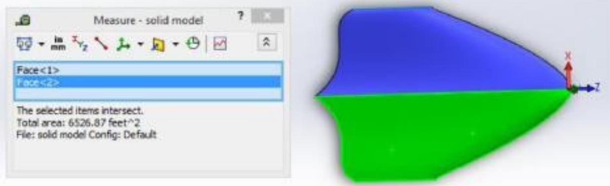
**Figure 43: Measurement of wet area of Center body from solid work model**
