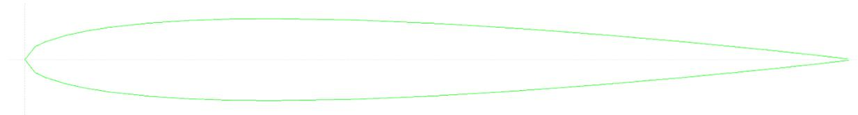
Figure 7.4 - NACA 0010 airfoil.
