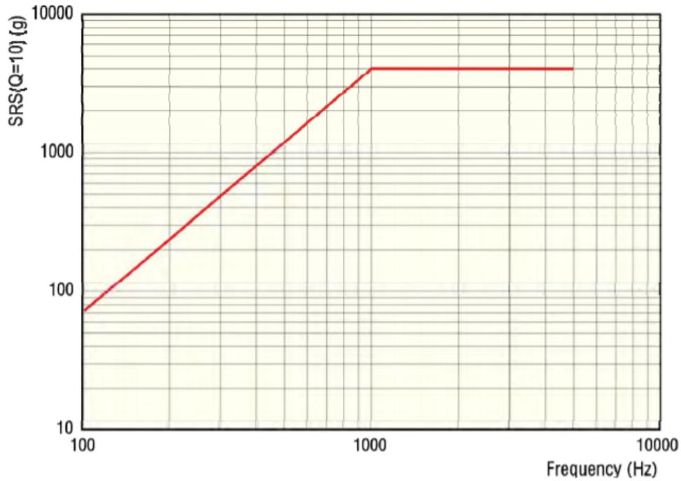
Figure 2.6: Frequency of shock vibration against g-force acceleration [27]
