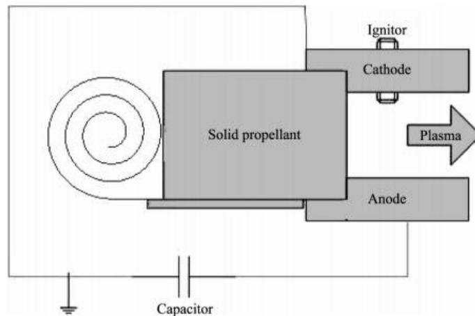
*Figure 1 Pulse Plasma Thruster (PPT) Parts [14]*
