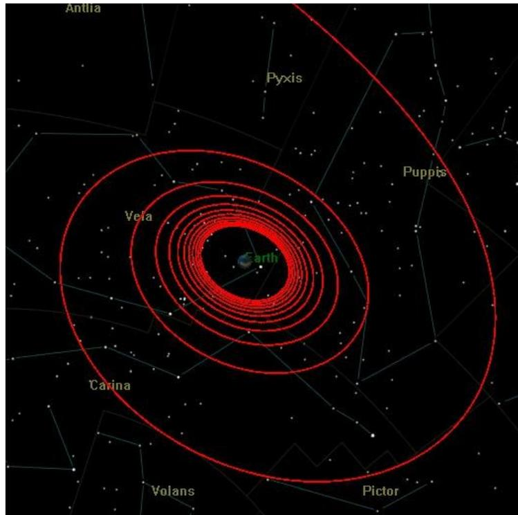
*Figure 17: Orbit Transfer from GEO to MTO Using HET*
