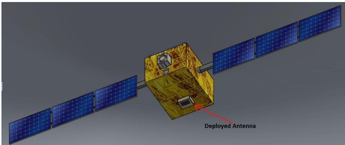
Figure 13: Deployed Antenna
