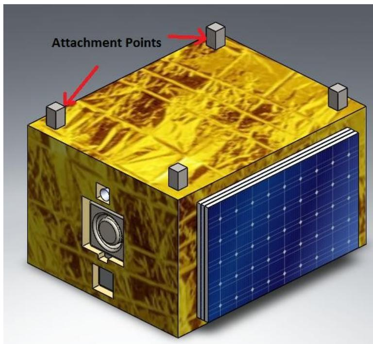
Figure 9: Stored Configuration of MMS [4]
