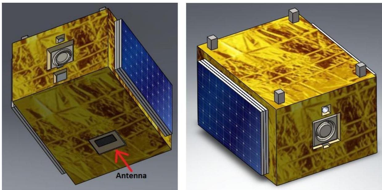
Figure 11: (Left) Bottom View of MMS with Stowed Antenna. (Right) Back View of MMS [4]
