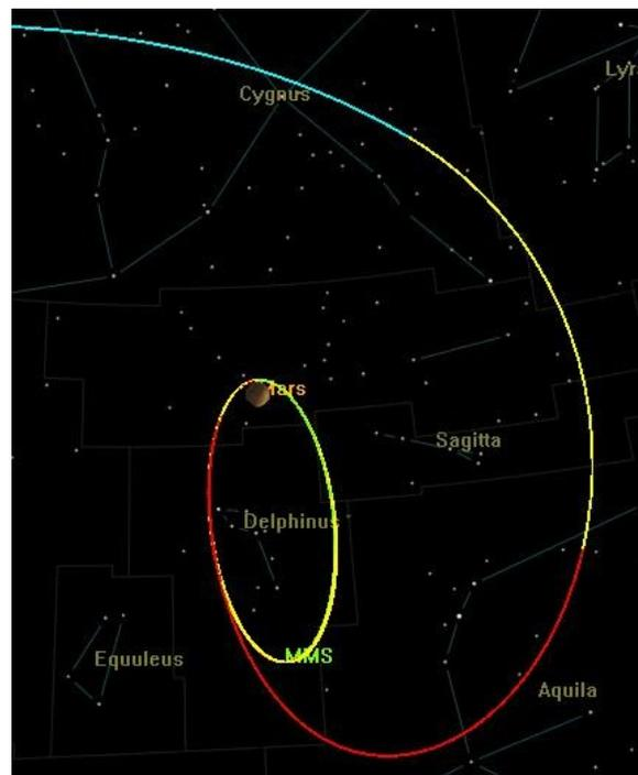
Figure 29: MMS at Mars Apoapsis to Reduce Eccentricity of Orbit, Phase 5.B ADN based Maneuver
