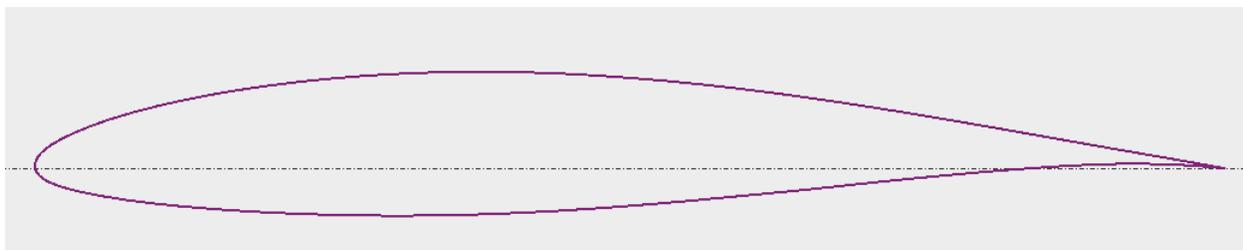
Figure 5.4 Boeing 747 root airfoil shape, generated from XFLR5
