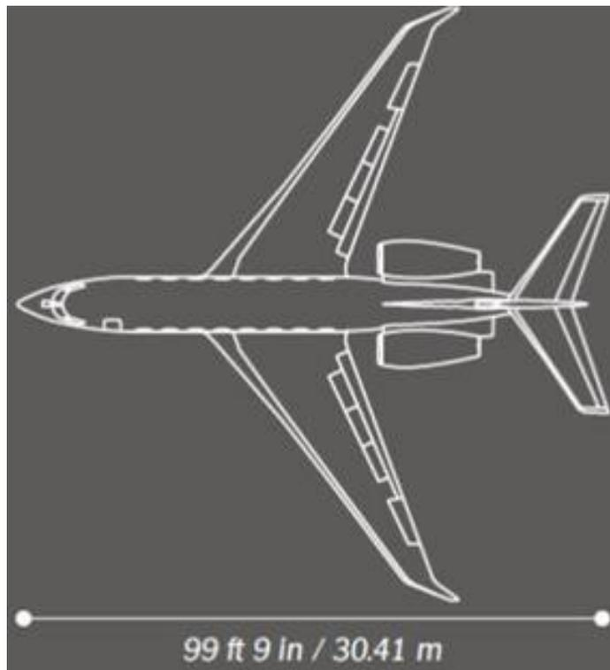
**Figure 1.4: Top view of Gulfstream G650**
