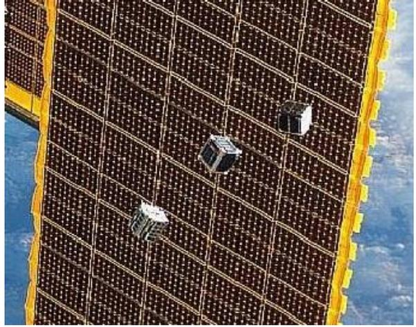
TES-3 was the 1st 3U CubeSat jettisoned from the ISS on November 19, 2013, and utilized an Exo-Brake system that was deployed as planned. TES-4 was jettisoned from the ISS on March 3, 2015 after being dormant on the ISS for almost a year. Building on flight heritage, TES-4 validates passive drag modulation and satellite-to-satellite communication. TES-4 is currently flying and is planned to re-enter atmosphere on April 11 +/- 1, 2015.
