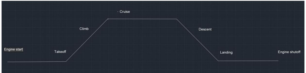
Figure 1.1 Mission Profile of the Hybrid-Electric Aircraft.
