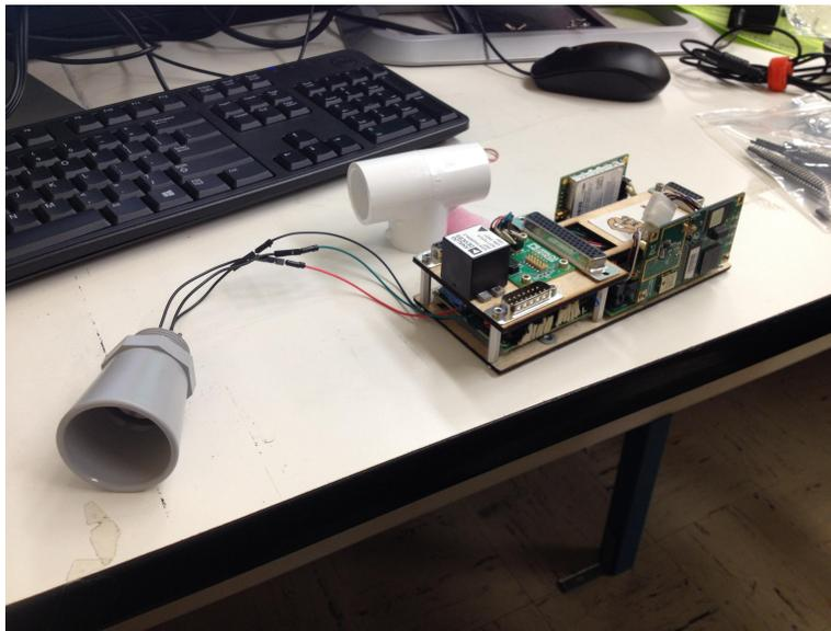
Figure 3. Ultrasonic Range Finder Attached to Flight Computer
