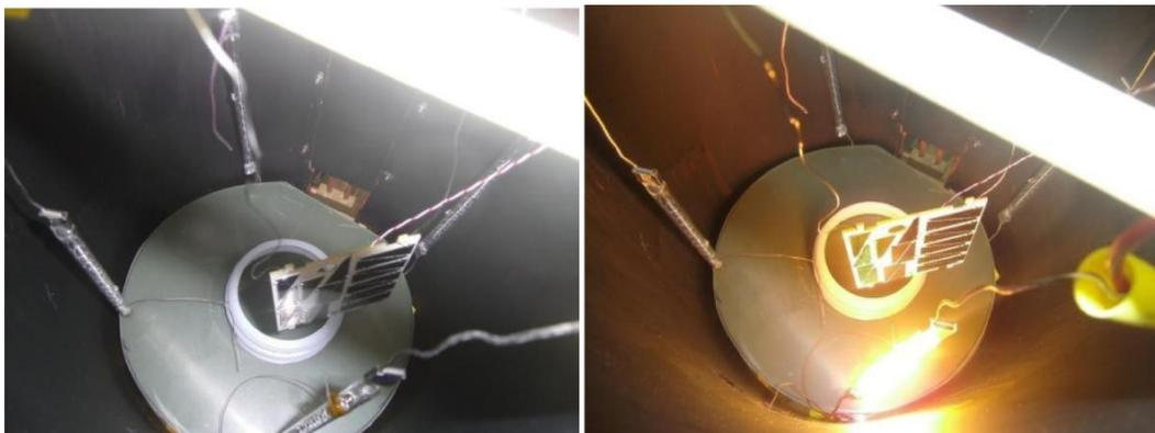
Figure XX-Pictures of solar panel in test chamber (with and without illumination)
