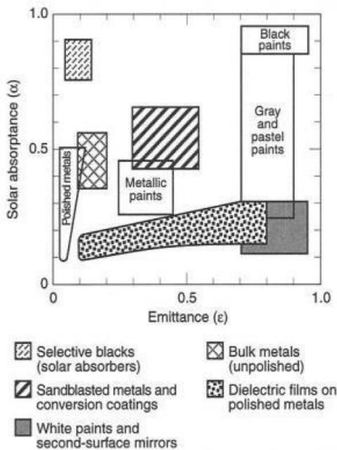
Figure XX-Surface Properties by type of Finish (Spacecraft Thermal Control Handbook, Gilmore, pg. 141)
