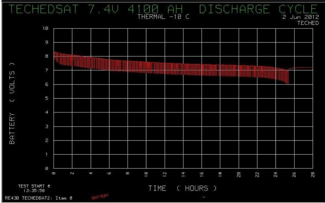
Figure XX-4100AH Test Battery Discharge Cycle at -10C
