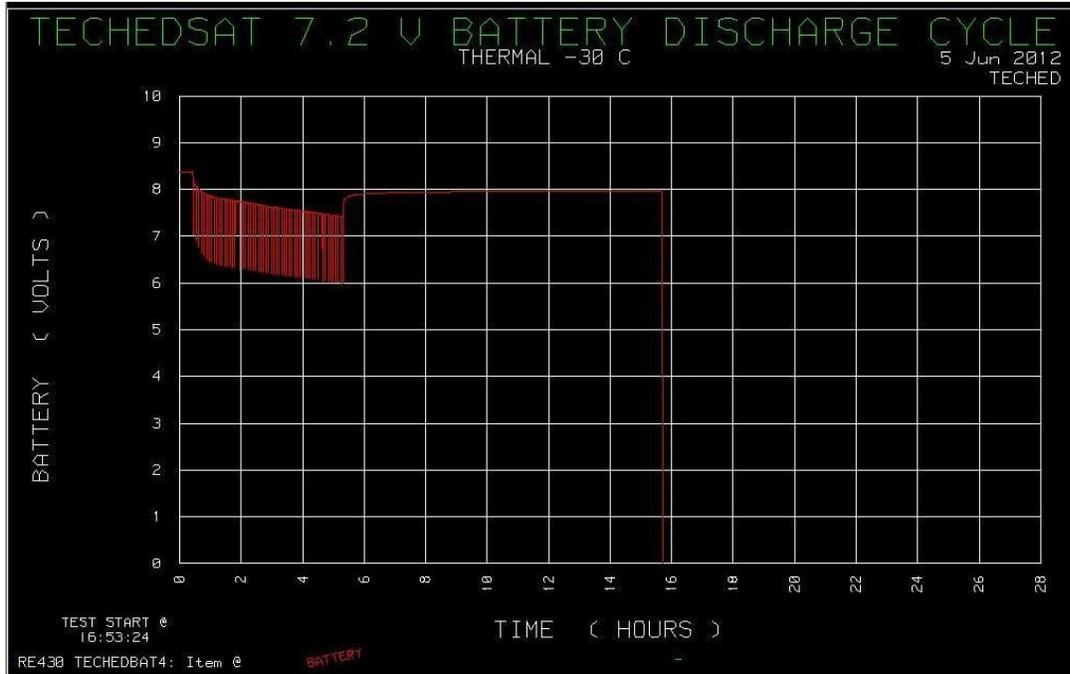
Figure XX-Test Battery Discharge Cycle at -30C
