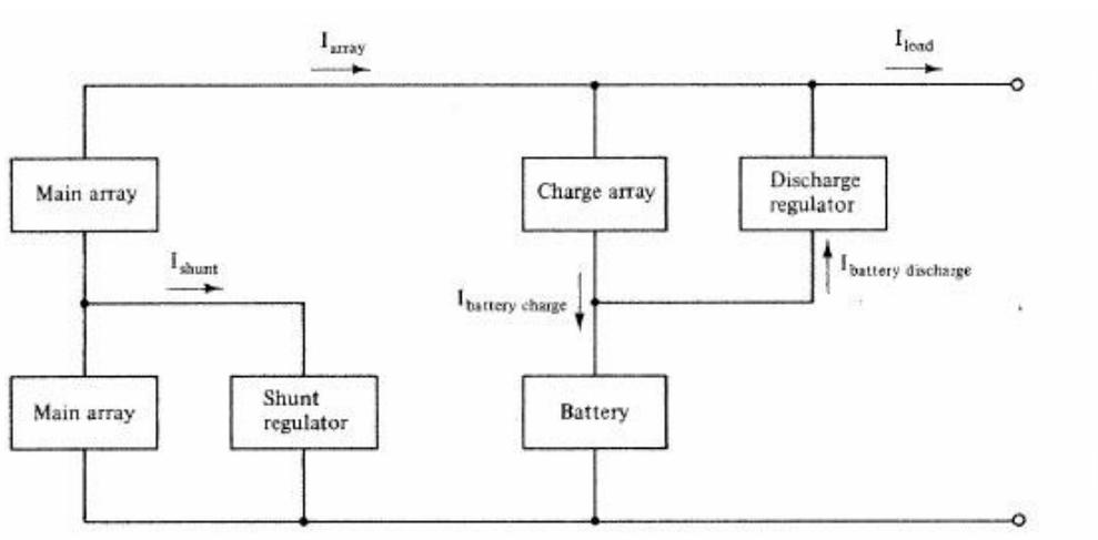
Figure 1-Block Diagram of Electrical Power Subsystem (Agarwal, 1986)
