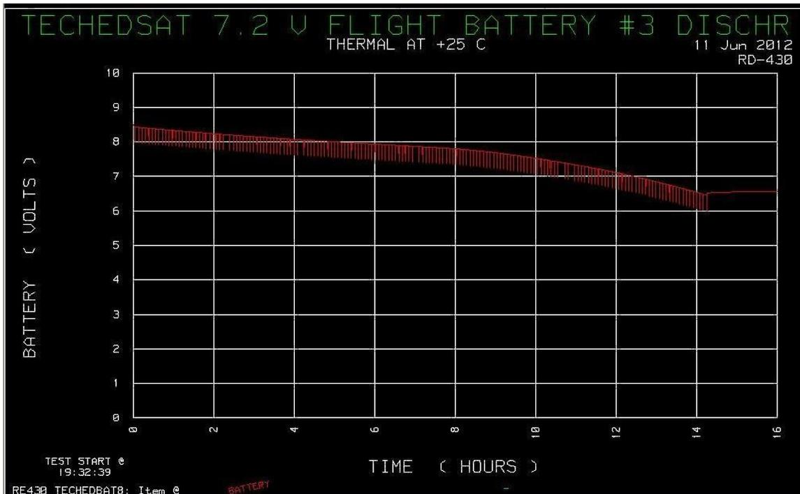
Figure XX-Spare Flight Battery Discharge Cycle at 25°C
