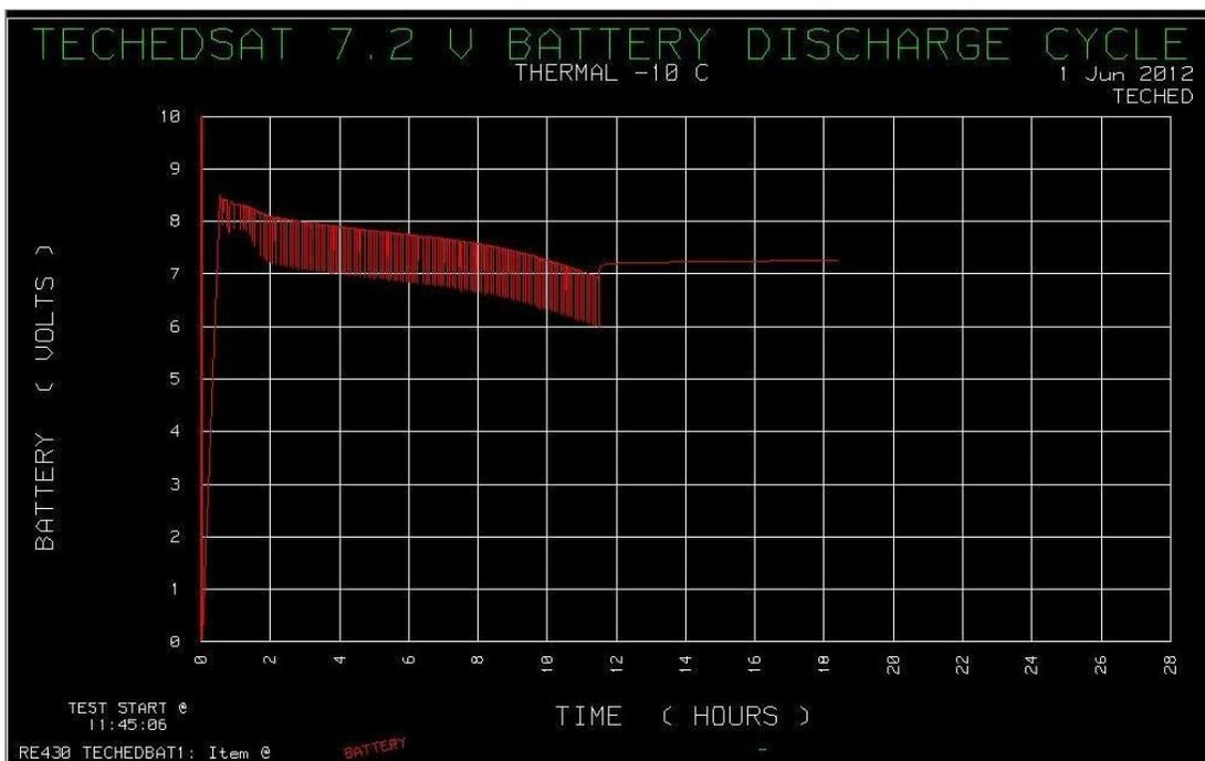
Figure XX-Spare Flight Battery Discharge Cycle at -10°C
