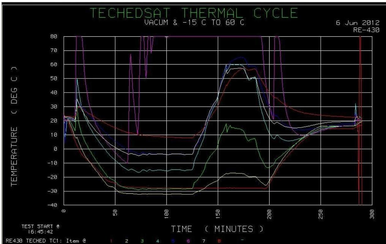
Figure XX-Thermal Cycle testing from -15 to 60°C
