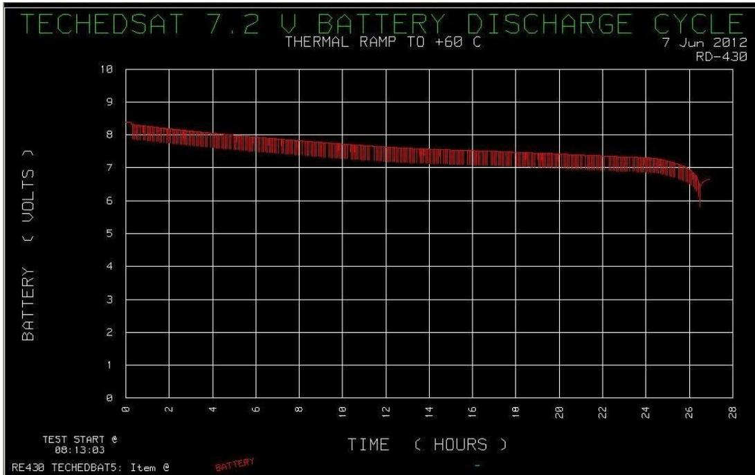
Figure XX-Test Battery Discharge Cycle ramped to 60C
