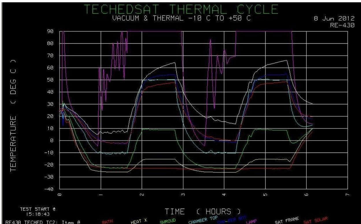
Figure XX-Thermal Cycle Testing from -10 to 50C
