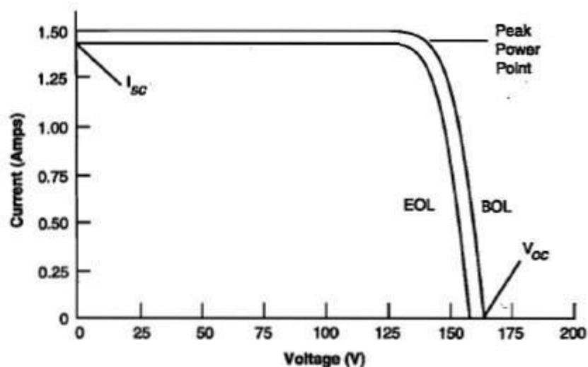
Figure 3-Current-Voltage Plot for a Planar Array
