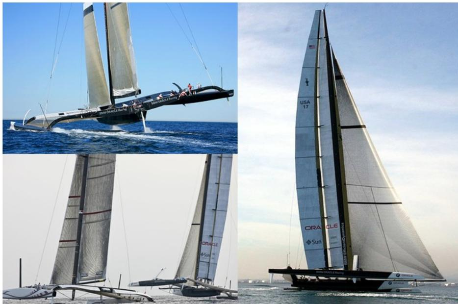
Figure 2: (Clockwise from top left): USA 17 with its traditional soft sail <sup>B</sup>, USA 17 with the wing mast and sail <sup>C</sup>, USA 17 and Alinghi 5 racing in the 2010 America's Cup <sup>D</sup>
