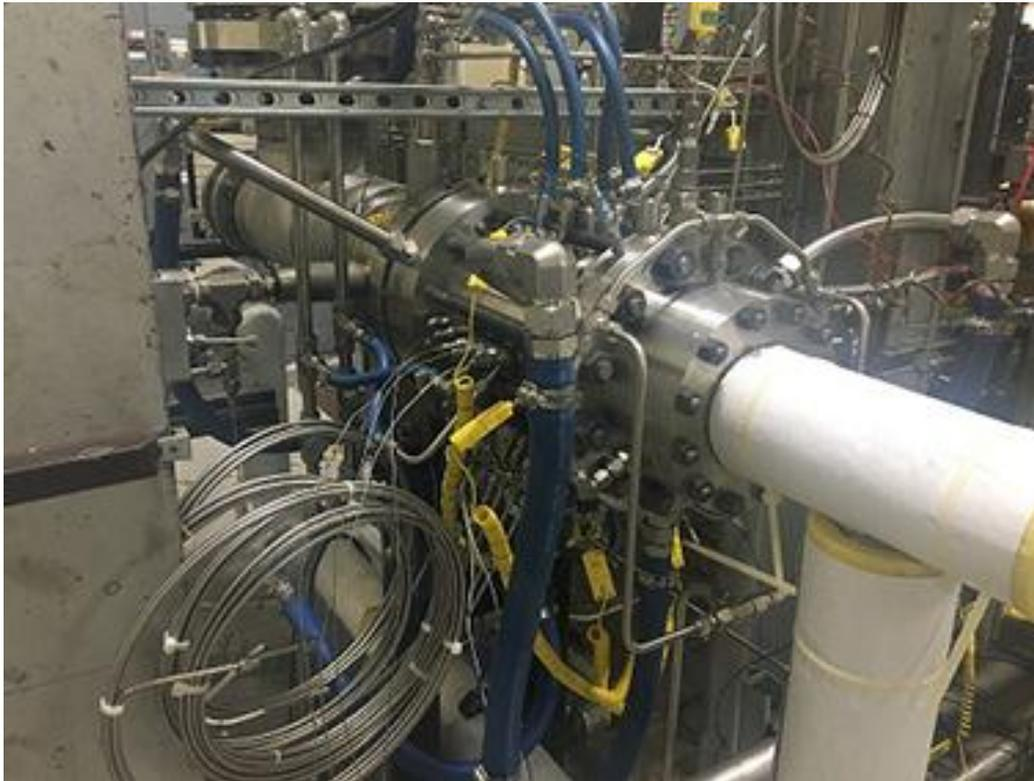
**Figure 13 NETL'S water-cooled rotating detonation engine [25].**
