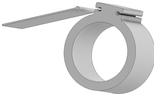
Figure 4.3: An example of how skin and frame can be joined together.
