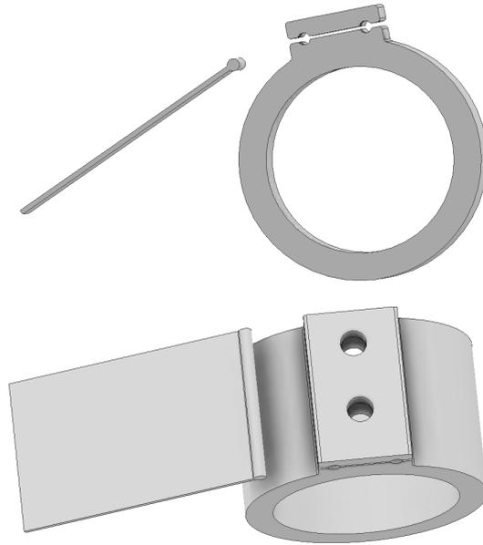
Figure 4.4: Two views of the cross section of an example of fastening the skin to the ribs.
