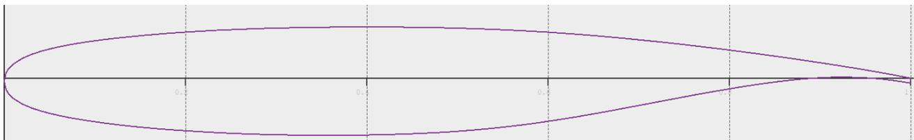
Figure 6.5. NASA SC (2) 0412 airfoil profile
