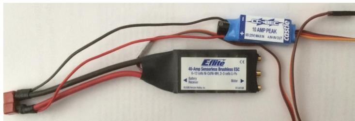
Figure 6. ESC and BEC
