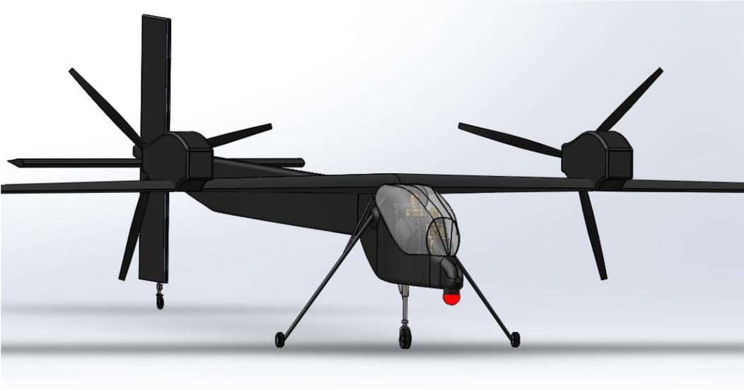
CAD drawing 14. Landing gear arrangement
