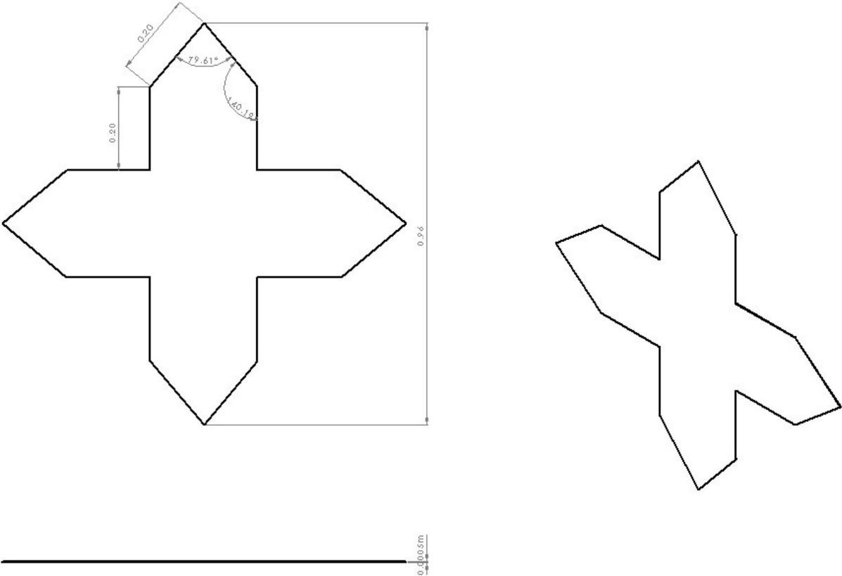
Figure 3: Flat Cross-Parachute Geometry
