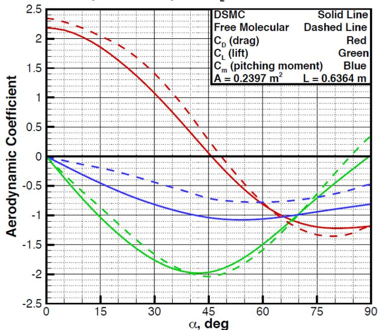
Figure 26 DAC & DACFREE Solution at 166 km
