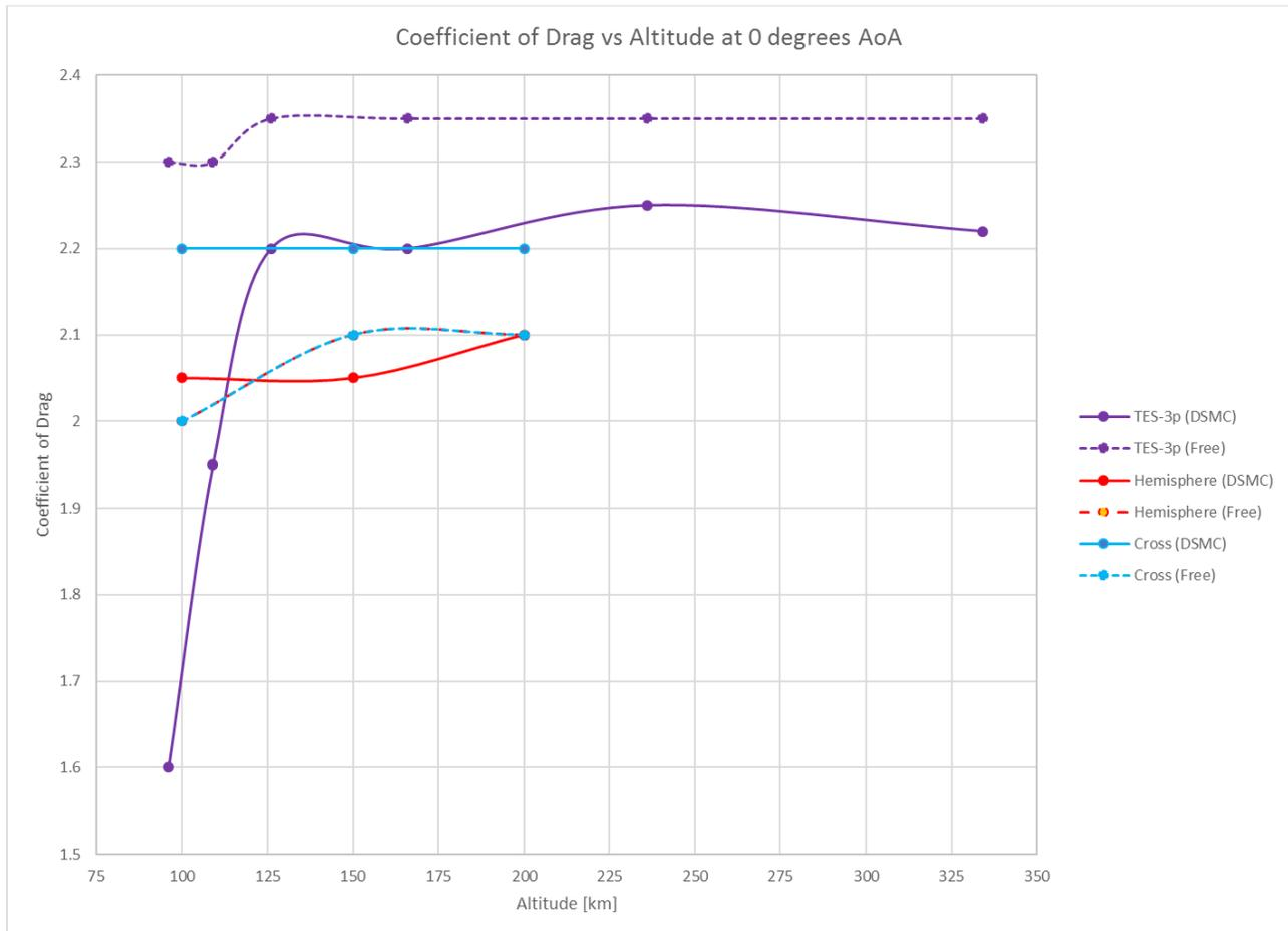
Figure 30 Coefficient of Drag versus Altitude at 0 Degrees Angle of Attack
