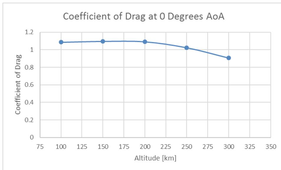
Figure 37 Coefficient of Drag versus Altitude at 0 Degrees Angle of Attack
