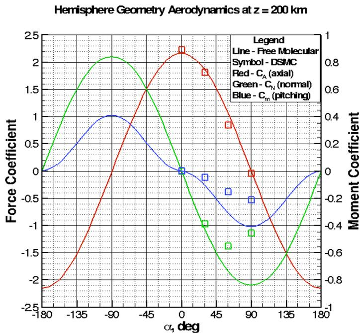
Figure 17 Dome Aerodynamics at 200km
