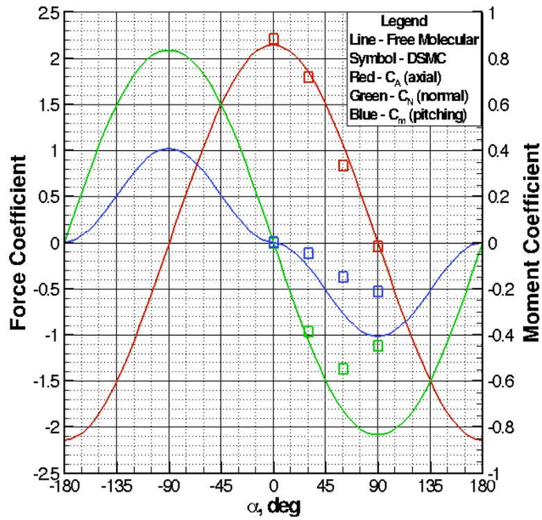
Figure 18 Dome Aerodynamics at 150km
