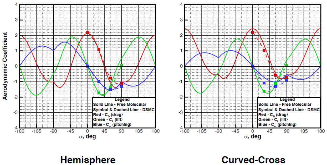
Figure 20 Aerodynamics at 150 km
