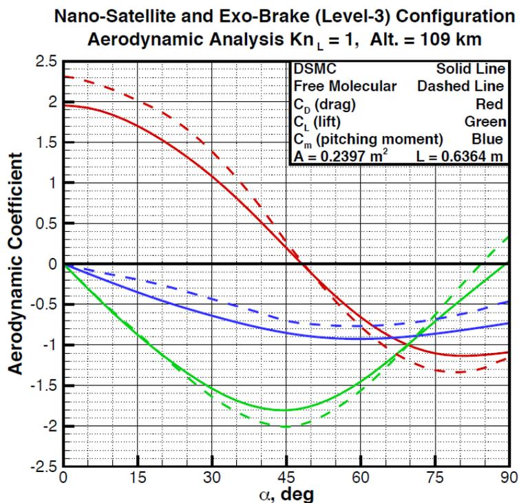
Figure 28 DAC & DACFREE Solution at 109 km
