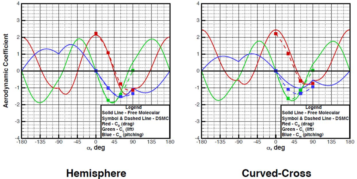
Figure 19 Aerodynamics at 200 km
