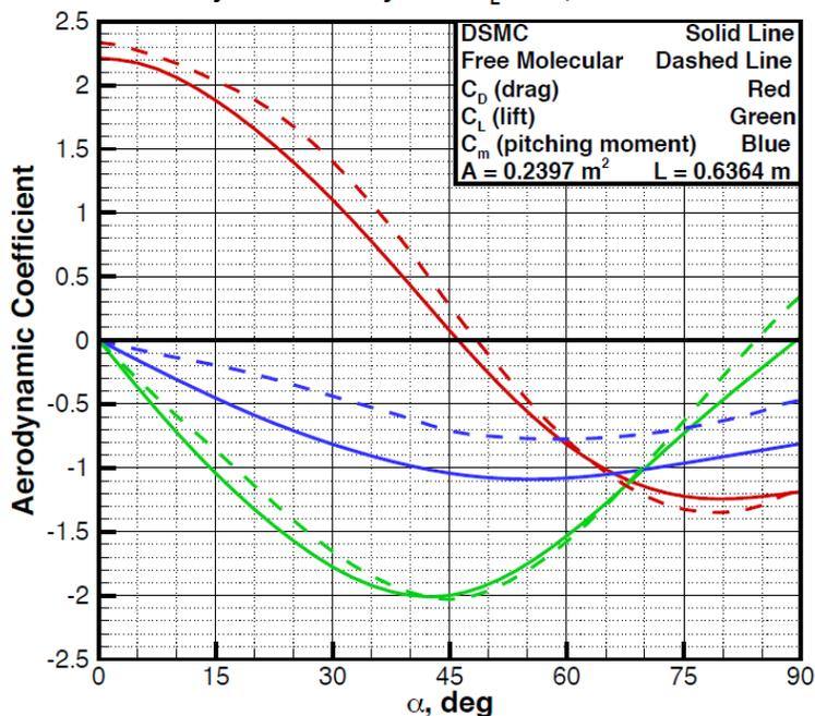
Figure 27 DAC & DACFREE Solution at 126 km
