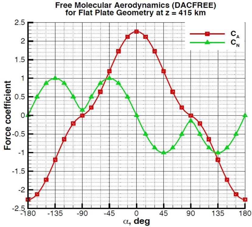
Figure 13 DACFREE for Flat Plate
