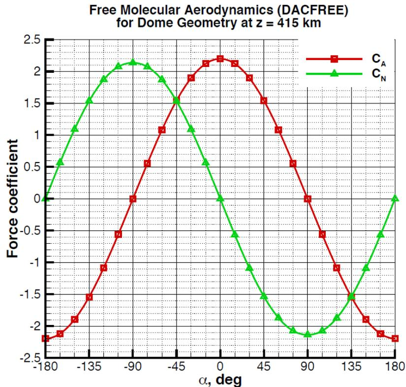
*Figure 15 DACFREE for Dome*
