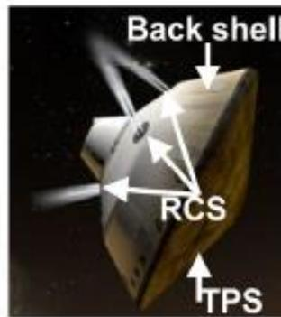
Figure 1 – Traditional aeroshell entry vehicle RCS design [3]
