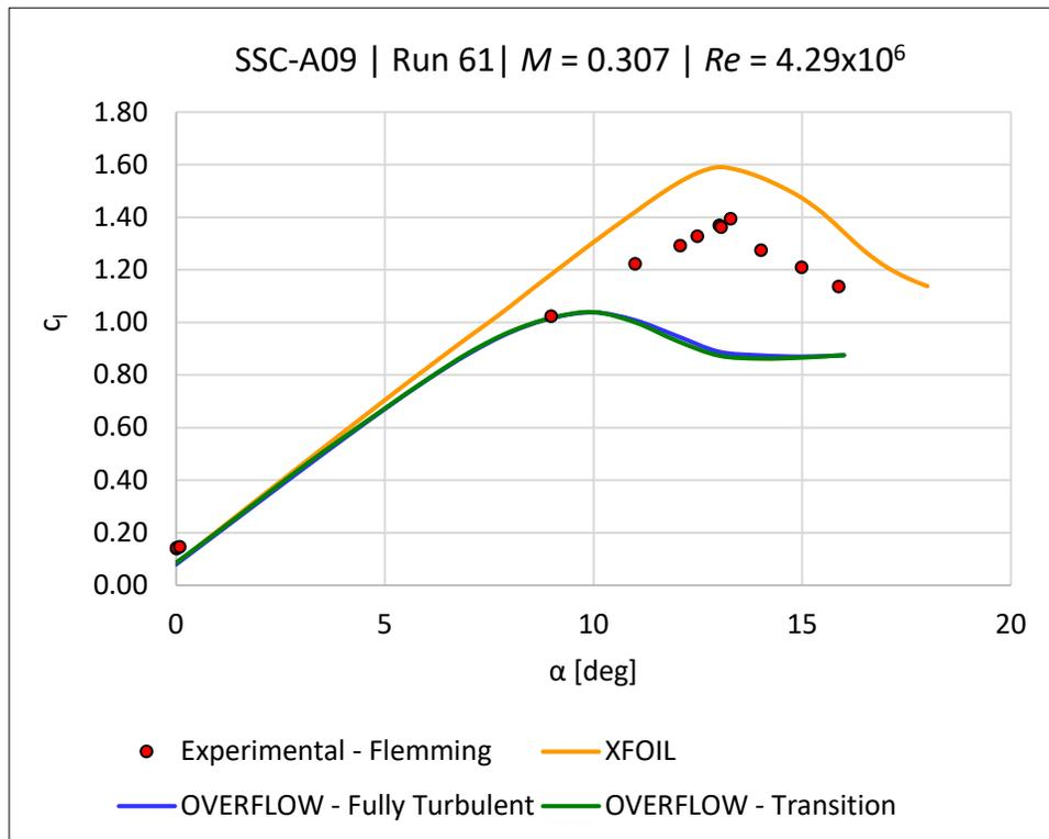
Figure D.2 SSC-A09, Run 61, Mach 0.307,  $Re\ 4.29 \times 10^6$ : lift coefficient versus  $\alpha$ .
