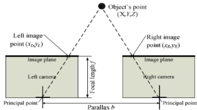
Figure 2.3: Stereo geometry illustration [62]
