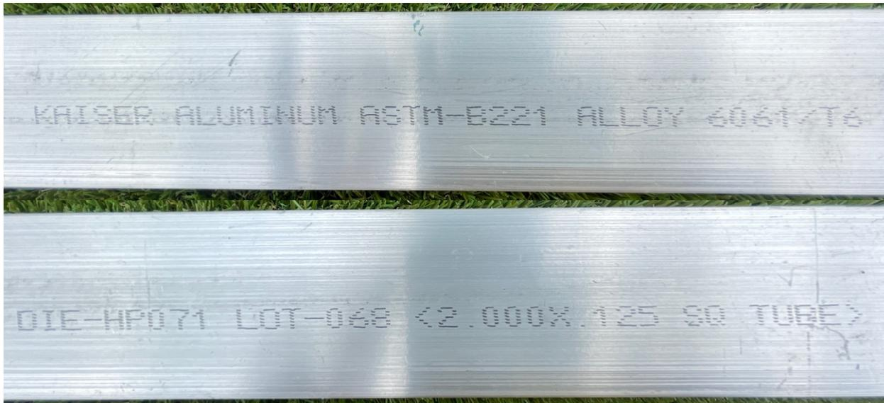
Figure 3.1: Manufacturer markings on square aluminum alloy tube.
