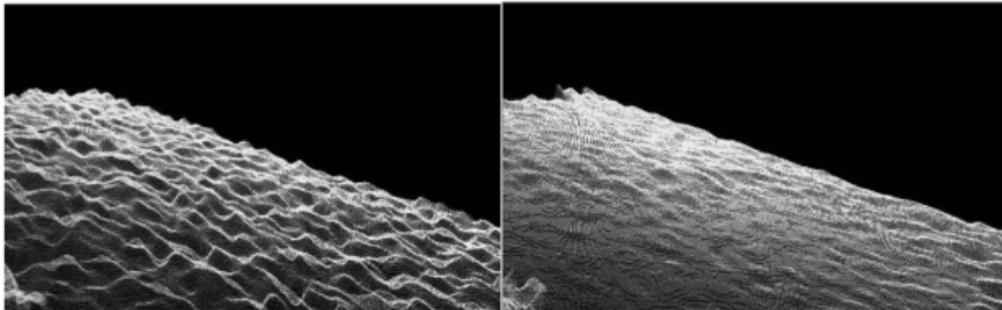
Figure 2.2: (Left) Depth noise from point cloud measured from a flat wall. (Right) Depth noise from the same surface, captured at a 3x lower NRMSE value.
