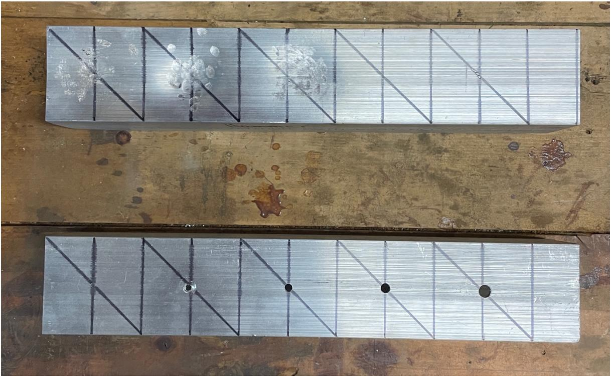
Figure 3.4: (Top) Object with damage from different hammers. (Bottom) Object with various size drill holes
