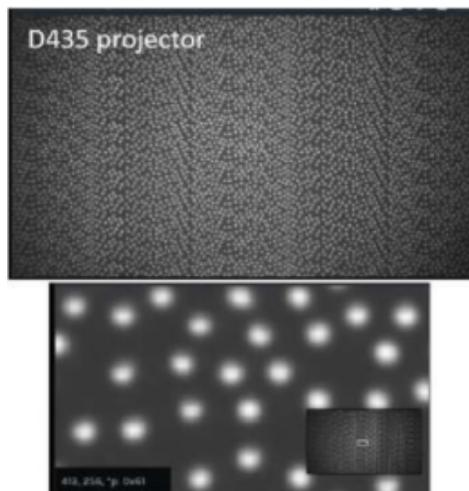
Figure 2.1: Intel RealSense D435 depth camera IR dot pattern [57]
