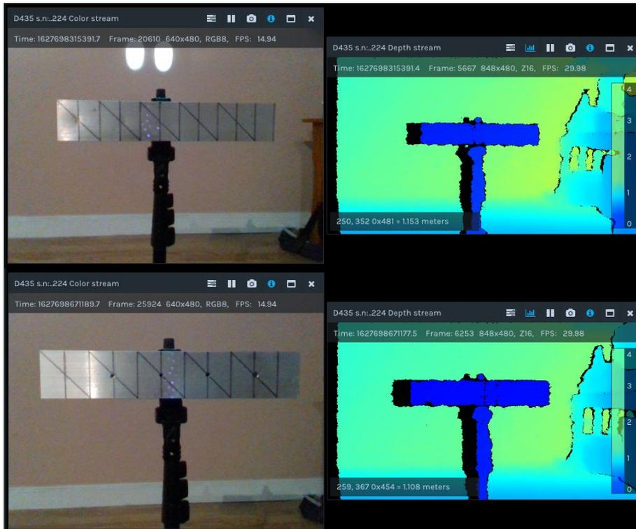
Figure 3.6: Images captured with D435 and displayed using Intel RealSense Viewer (Top) Object damaged with hammers (Bottom) Object damaged with drill holes
