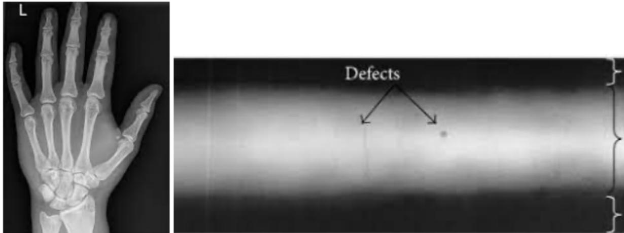
Figure 1.2: (Left) Hand X-ray [21] (Right) Shadowgraph of welded seam with defects [22]
