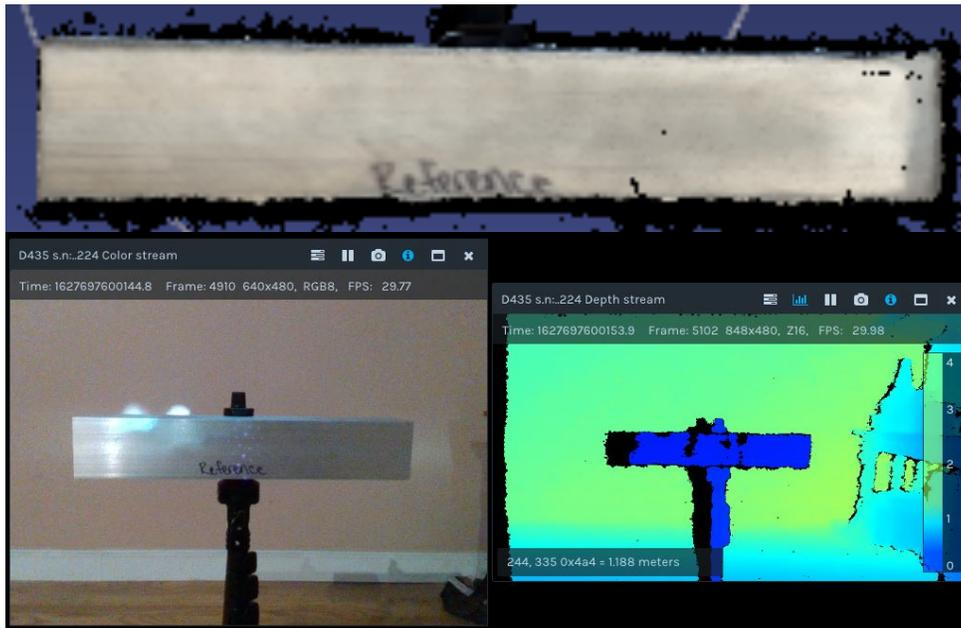
Figure 3.2 (Top) Object captured with iPhone displayed in MeshLab (Bottom) Object captured with D435 displayed in RealSense Viewer
