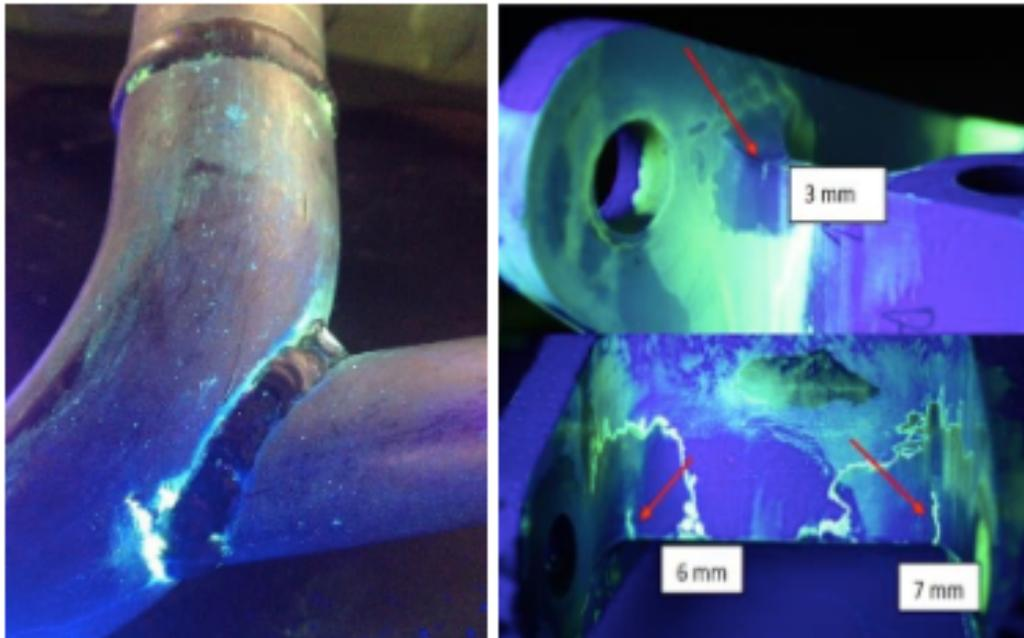
Figure 1.4: (Left) Welded exhaust pipe [31] (Right) Cracked landing gear fork [32]
