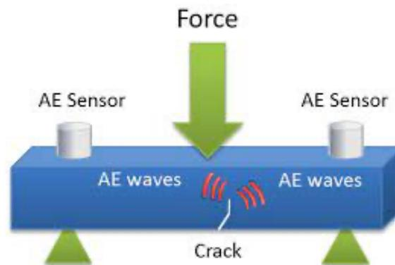
Figure 1.3: Diagram of acoustic emission method [29]
