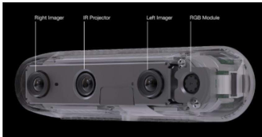
Figure 1.6: Intel RealSense D435 depth camera [48]
