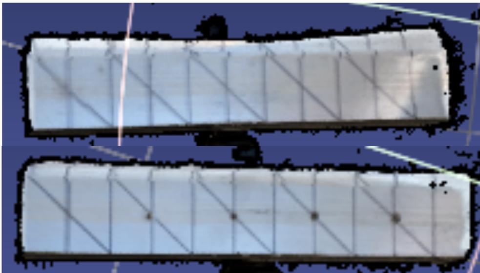
Figure 3.5: MeshLab view (Top) Object with damage from different hammers (Bottom) Object with various size drill holes
