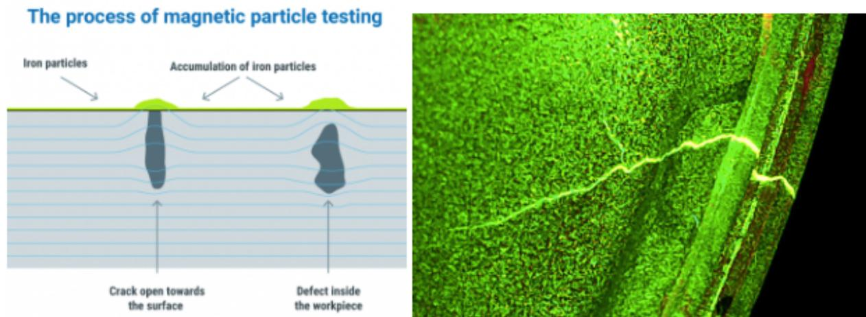
Figure 1.1: (Left) Magnetic particle testing diagram [19] (Right) Crack detected using fluorescent magnetic particle testing [20]
