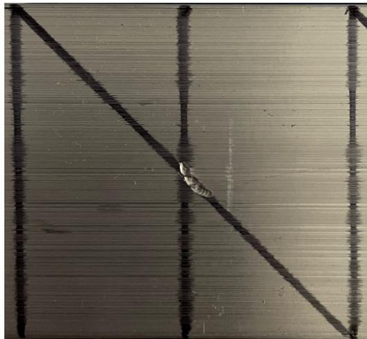
Figure 6.3: Damage created by screwdriver and hammer
