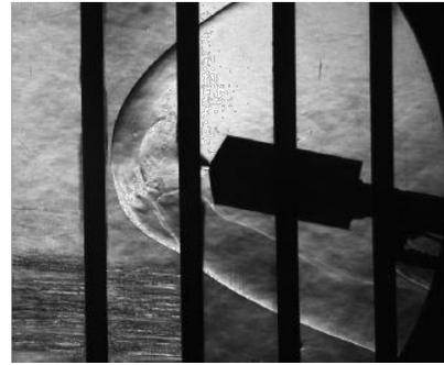
**Fig. 9** Single nozzle,  $\alpha = 12$ -deg,  $C_t = 4$ , Mach 4.6. [2]
