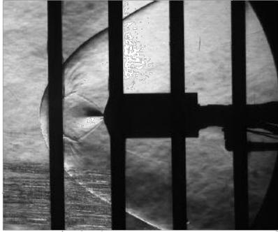
**Fig. 8** Single nozzle,  $\alpha = 0$ -deg,  $C_t = 4$ , Mach 4.6. [2]
