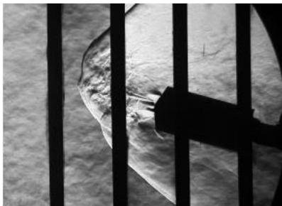
**Fig. 18** Quad-Nozzle,  $\alpha = 16$  Ct =2,  $\phi = 0$  Mach 2.4.[2]
