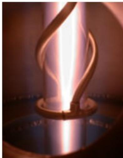
Figure 16 Steady-state helicon discharge Source: Blackwell, 1997
