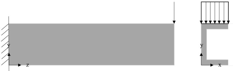
Figure 4.2 – Case 1: 100 N point load in the -y direction at free end, constant along x axis.
