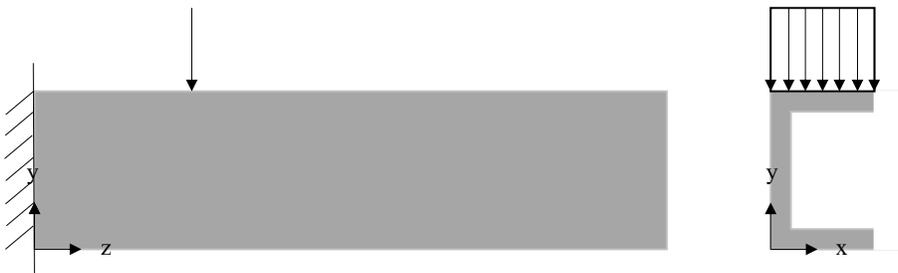
Figure 4.5 – Case 4: 100 N point load in the -y direction at quarter length, constant along x axis.
