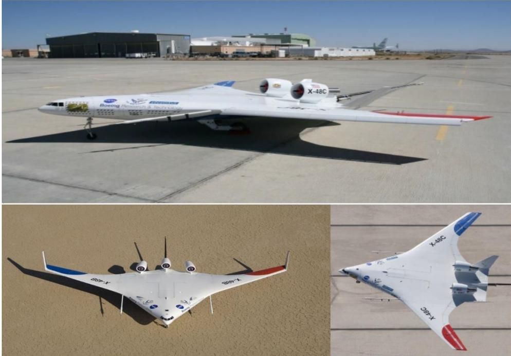
Figure 3 Boeing X-48B (8.5% Scaled for Conceptual HWB Commercial Aircraft)
