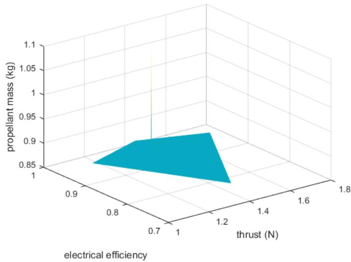
Figure 11: The figure shows the response surface of the interaction between the electrical efficiency and the thrust and their implication on the propellant mass.
