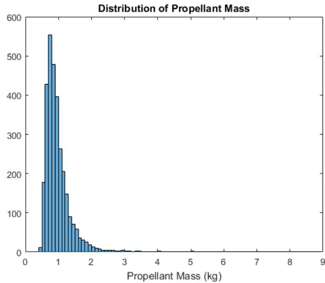
Figure 9: The figure shows the distribution of initial propellant masses fulfilling the requirements.
