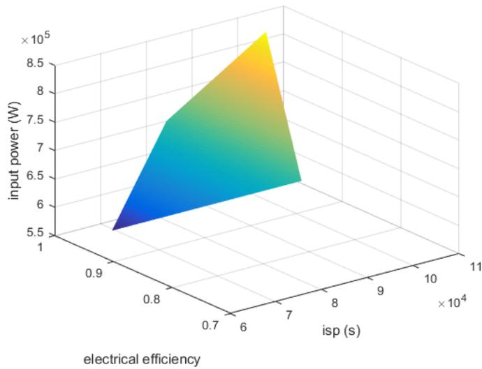
Figure 13: The figure shows the response surface of the interaction between the  $I_{sp}$  and the electrical efficiency and their implication on the input power.
