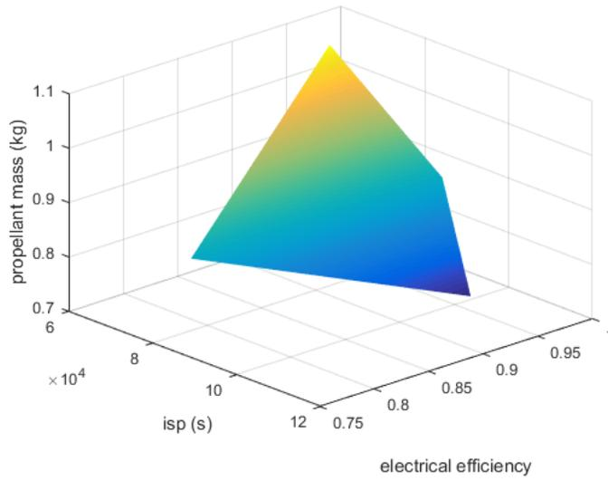
Figure 10: The figure shows the response surface of the interaction between the electrical efficiency and the  $I_{sp}$  and their implication on the propellant mass.
