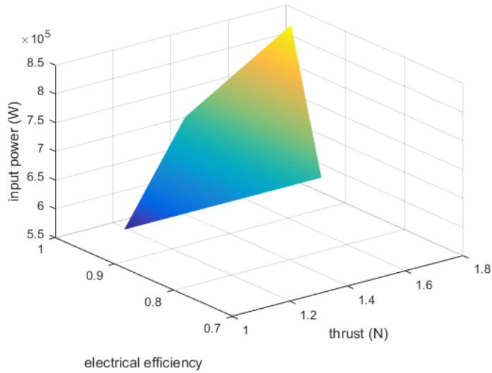
Figure 14: The figure shows the response surface of the interaction between the thrust and the electrical efficiency and their implication on the input power.
