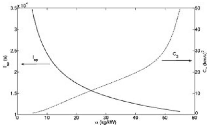
Figure 2: The figure shows variation of  $I_{sp}$  and launch energy with the power systems specific mass. The plot is taken from "Maximizing Payload Mass Fractions of Spacecraft for Interplanetary Electric Propulsion Missions [10]."
