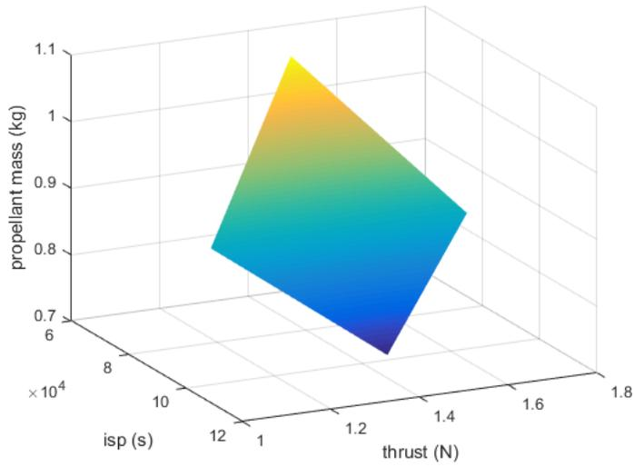
Figure 12: The figure shows the response surface of the interaction between the  $I_{sp}$  and the thrust and their implication on the propellant mass.
