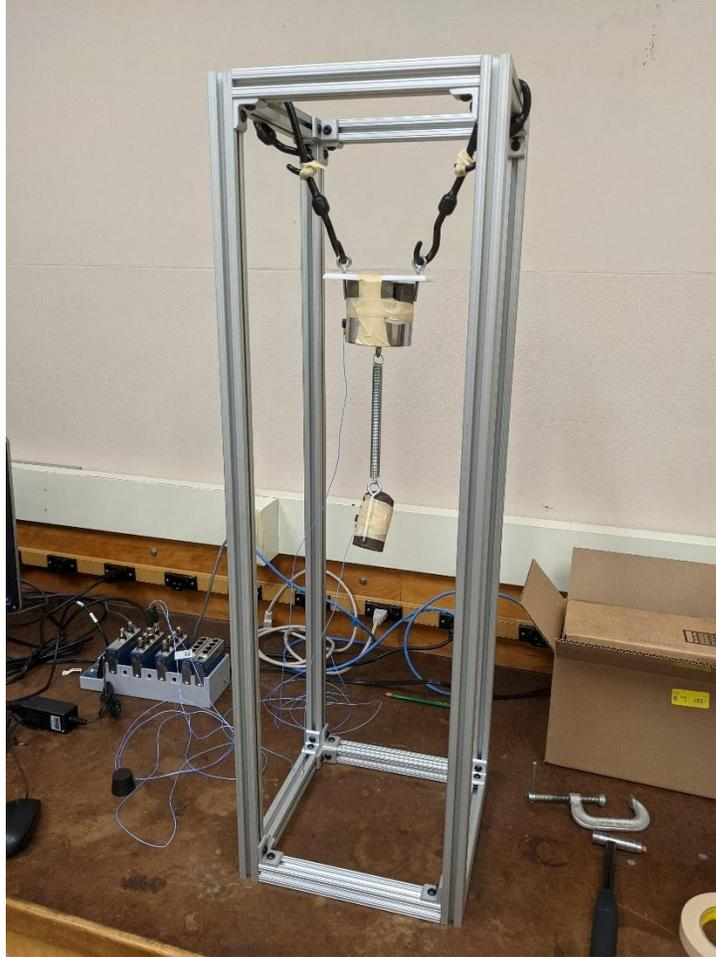
**Figure 5.6: Vibration absorber experiment final setup**
