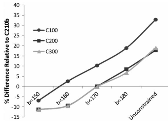
Fig. 12 Comparison of total wing truss system weights.
