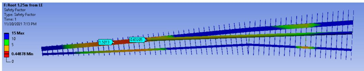
Figure 37- Stress FOS fails to meet 1.5 design specification between strut connection and 2m outboard
