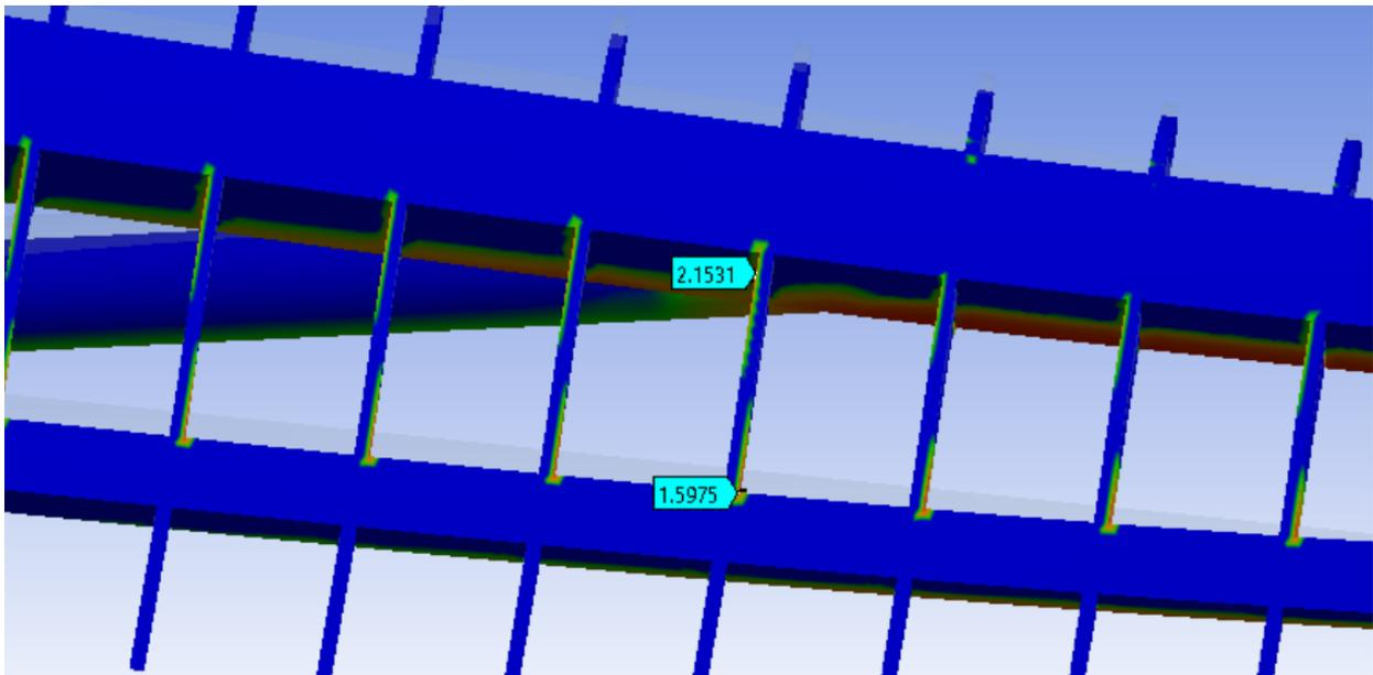
Figure 35 - Design change improves shearing force on ribs increasing stress FOS from 0.74 to 2.1
