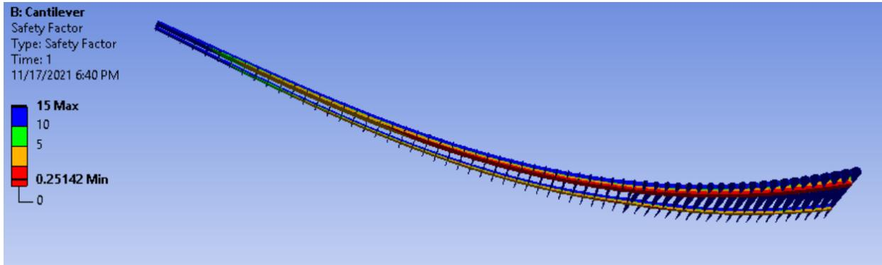
Figure 28 - Based on this study of stress, the wing has a minimum 0.251 FOS and would yield to failure
