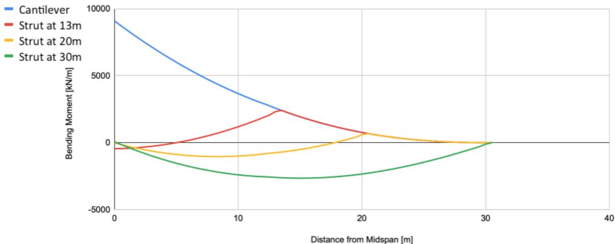
Figure 15 - Bending moment results from strut position sweep
