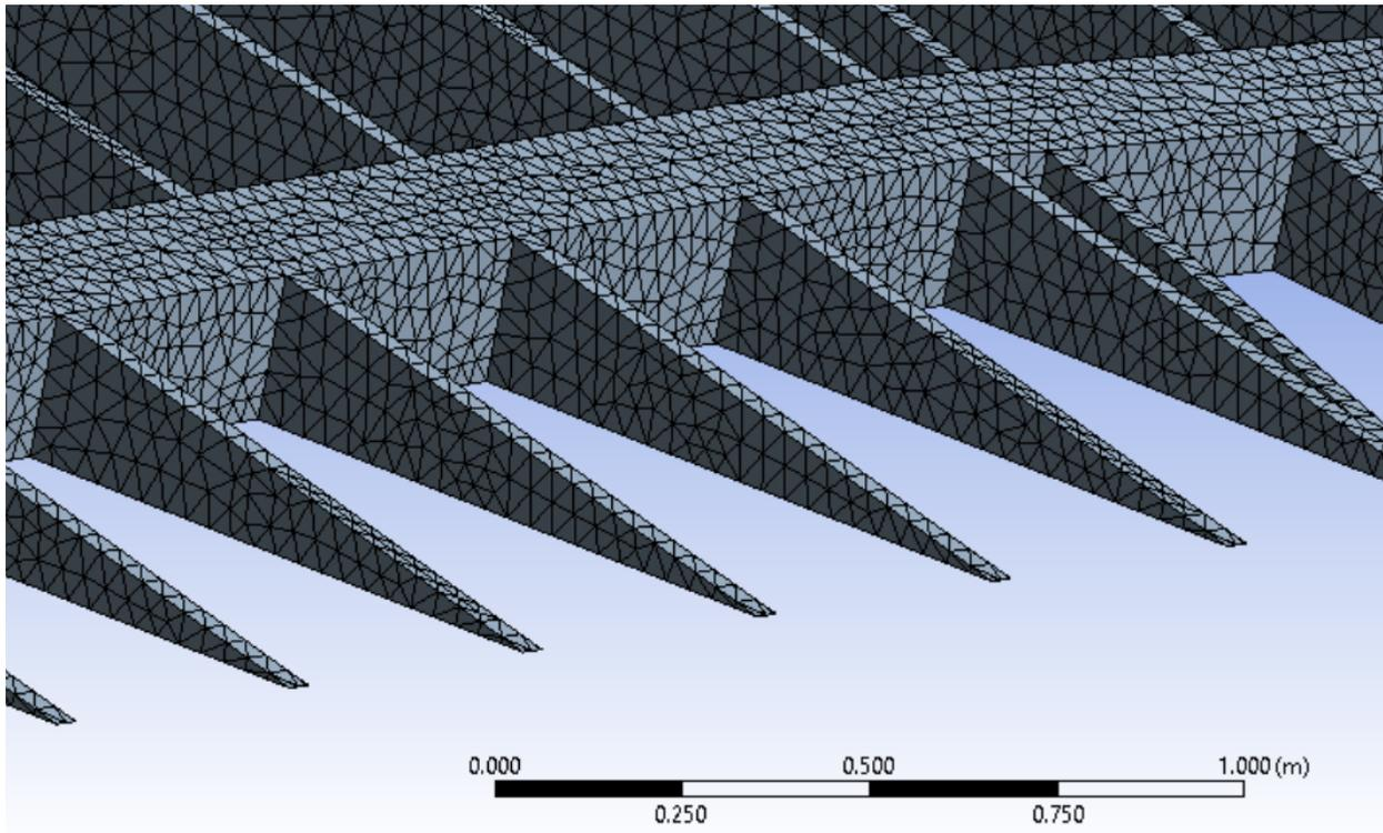
Figure 23 - Main wing mesh at 0.05m tetrahedron
