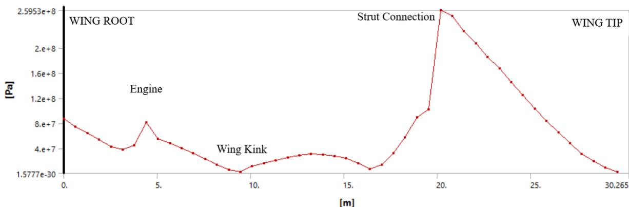
Figure 36 - Maximum principal stress along main spar of strut supported wing
