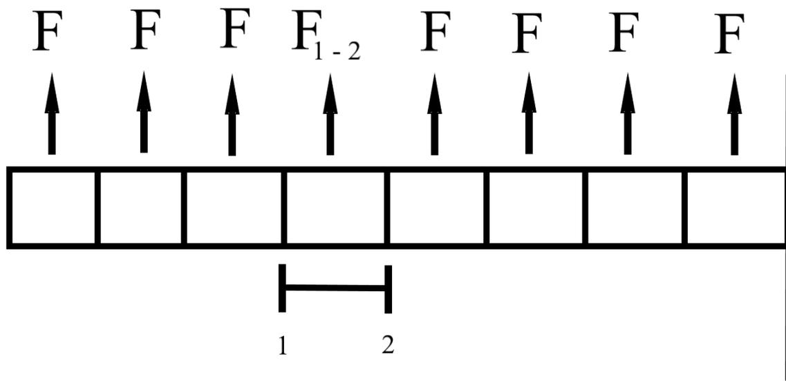
Figure 12 - Beam cut into sections for distributed load calculations
