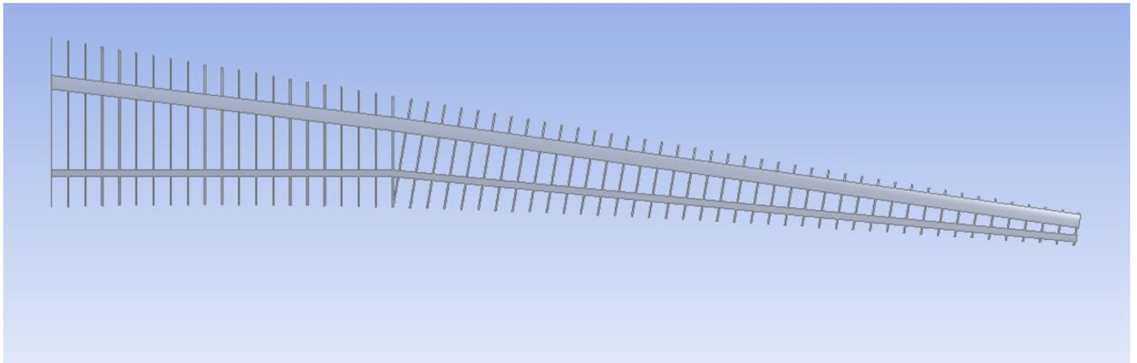
Figure 18 - SUGAR Wing internal frame structure based on F11 Megaliner frame
