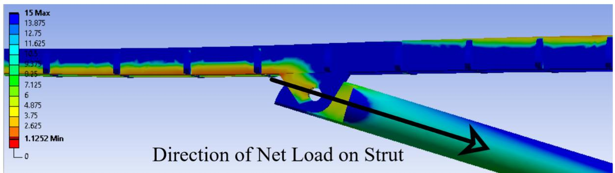
Figure 43 - FOS stress propagation on bracket follows direction of load from strut
