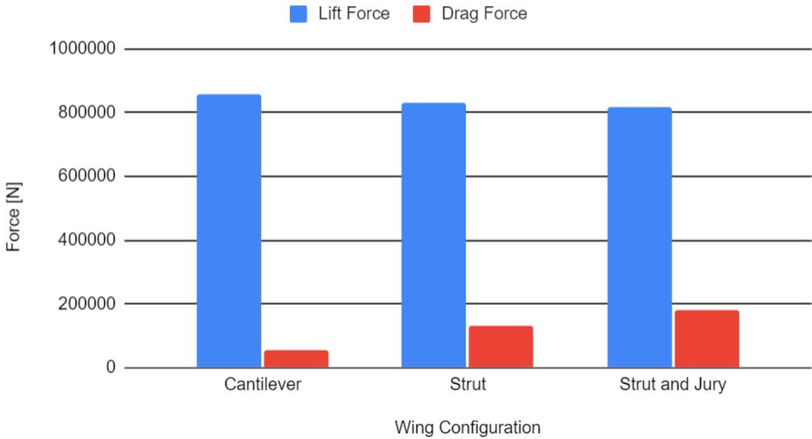
Figure 61 - Lift and drag value plot for each bracing configuration
