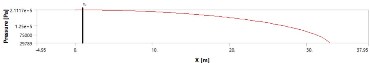
Figure 24 - Elliptical Loading result for baseline pressure loading across half span length
