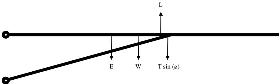
Figure 11 - Reduced loads on wing
