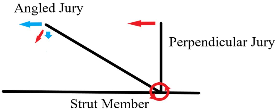
Figure 55 - A jury angles, the component contributing to moment about the joint decreases
