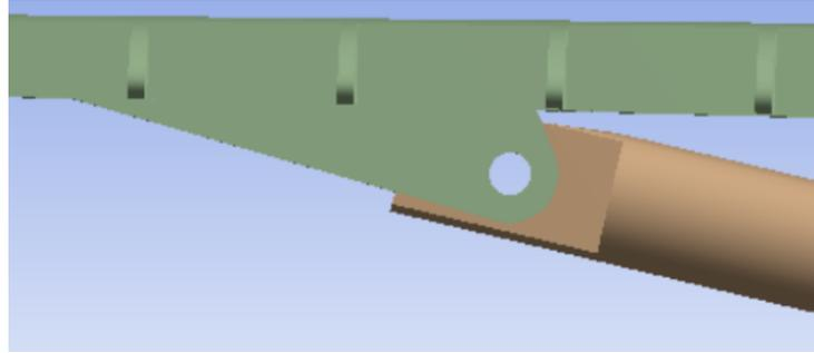
Figure 46 - Iteration 4 modified strut connection bracket
