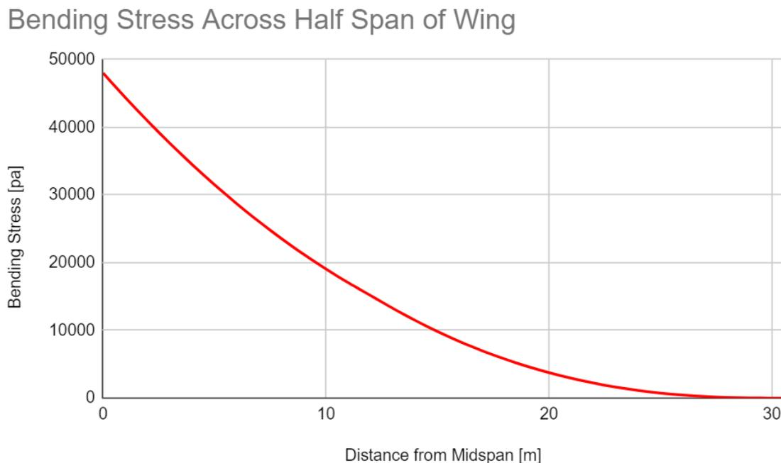
Figure 25 - Bending stress of classical calculation
