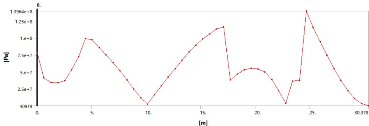
Figure 51 - Stress intensity along the main spar in with a single strut and vertical jury at 17 meters from wing root to tip
