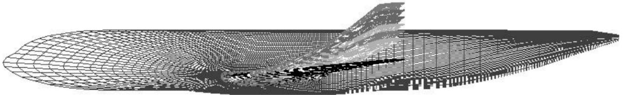
Figure 5 - Deformation of cantilever wing due to rib placement
