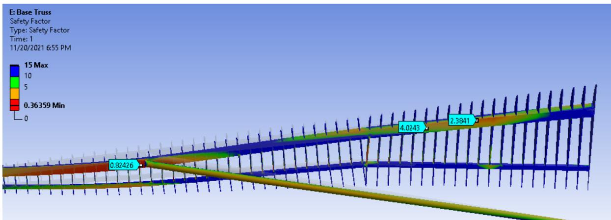
Figure 34 - Tensile stress has 0.82 FOS at strut joint while FOS at engine is 4
