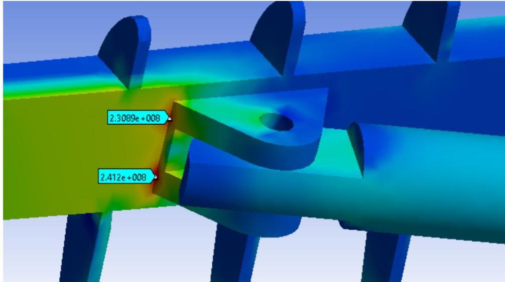
Figure 44 - Stress peaks seen at edges of pin bracket [pascals]
