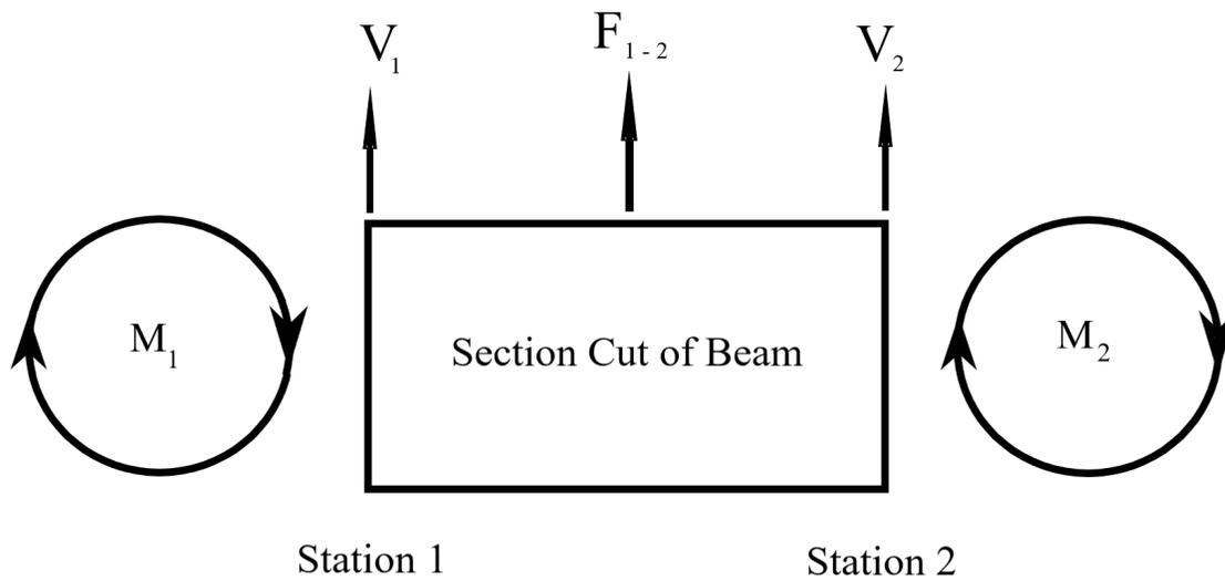
Figure 13 - Section cut of the beam with free body loads
