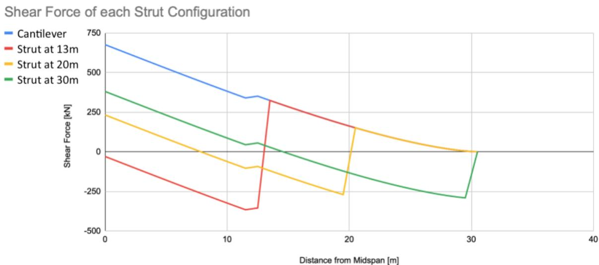
Figure 14 - Shear force results from strut position sweep
