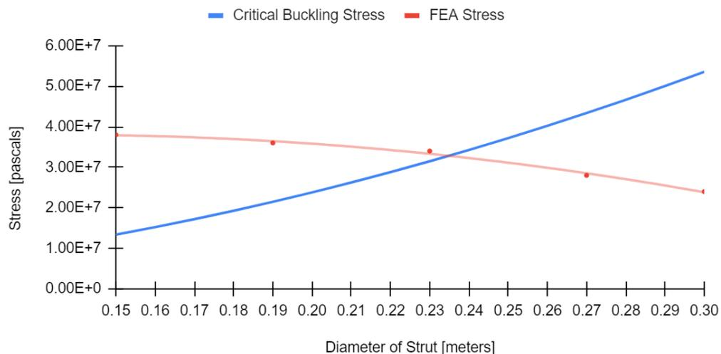
Figure 48 - Comparison between the calculated critical buckling stress compared to the FEA simulated maximum stress for each strut diameter
