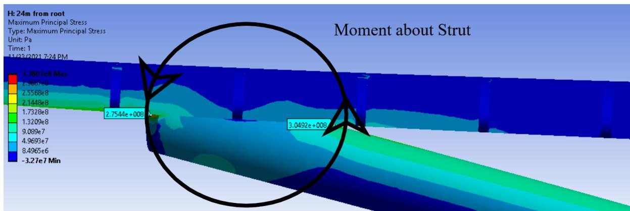
Figure 41 - Moment about strut connection causing high stress at edges
