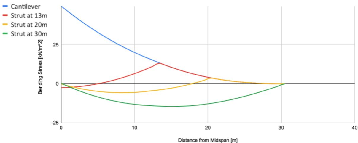
Figure 16 - Bending stress results from strut position sweep
