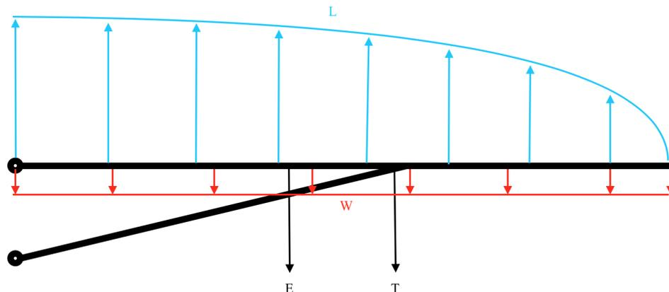
Figure 8 - Free body diagram of vertical loading on beam simplification
