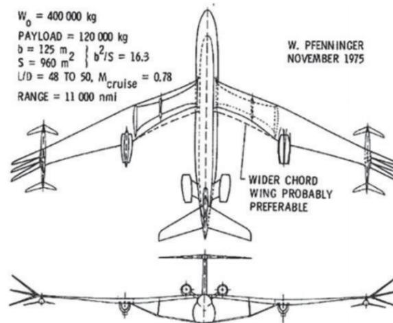
Figure 1 - Werner Pfenninger's concept of a more efficient high aspect ratio wing
