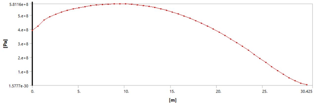
Figure 26 - Solid SUGAR wing main wing stress across span of wing
