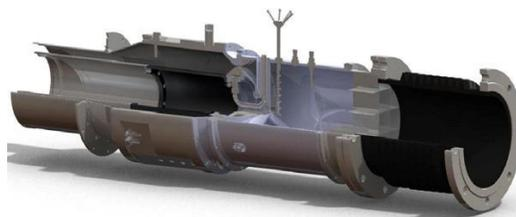
Figure 15: Continuous detonation wave combustor integrated into a GTD-350 turbojet <sup>3</sup>
