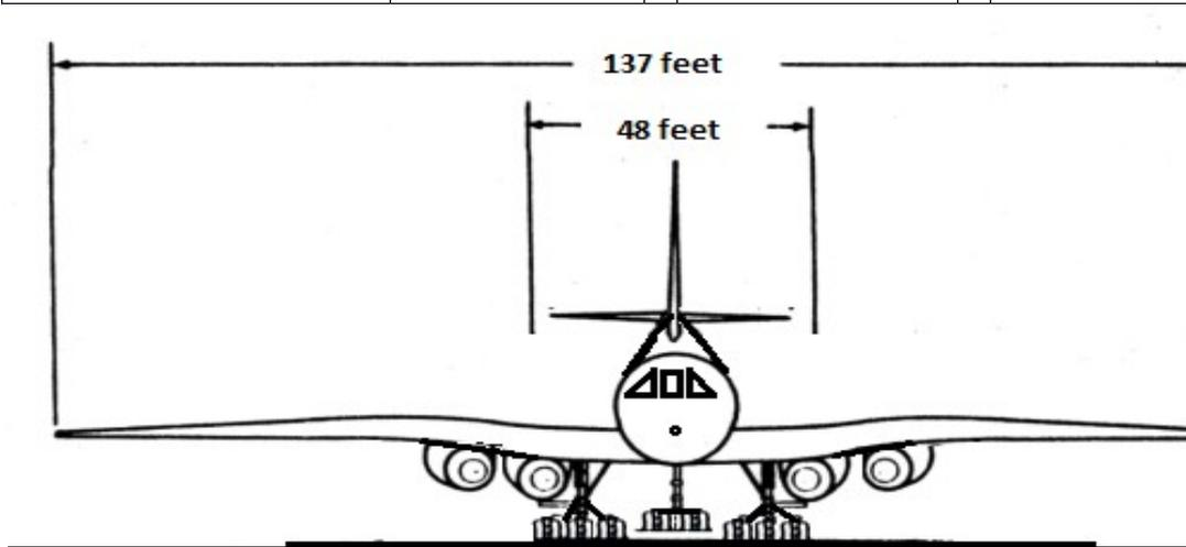
Figure 11 Front view of the SST
