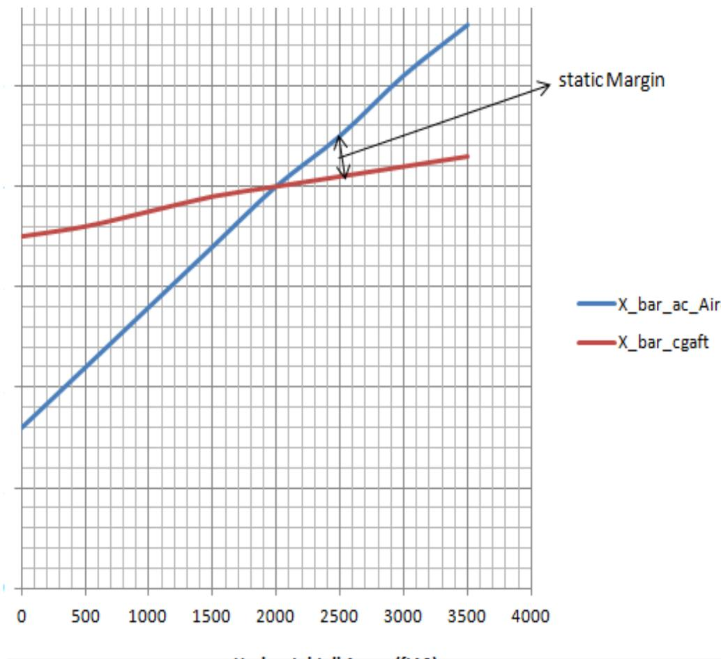
Figure 9 Static Longitudinal X-plot
