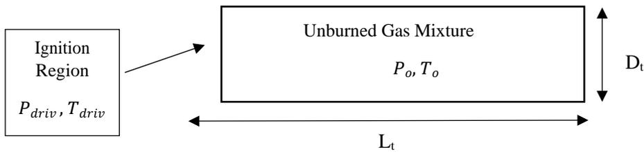
Figure 18 Schematic of 2-D Axisymmetric Ideal PDE tube
