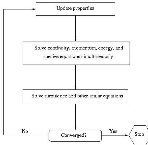
**Figure 17 Algorithm for Density Based solver in ANSYS Fluent**
