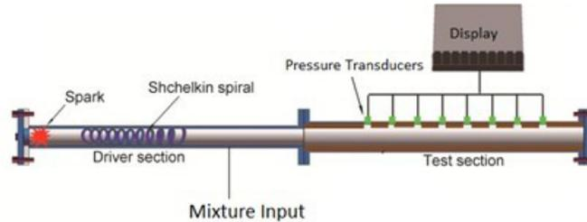
**Figure 11 General PDE experimental setup with Shchelkin spiral**
