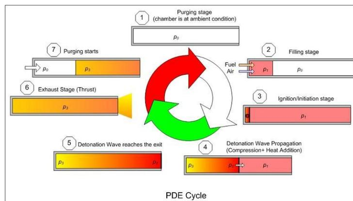
Figure 8 Pure PDE operating cycle
