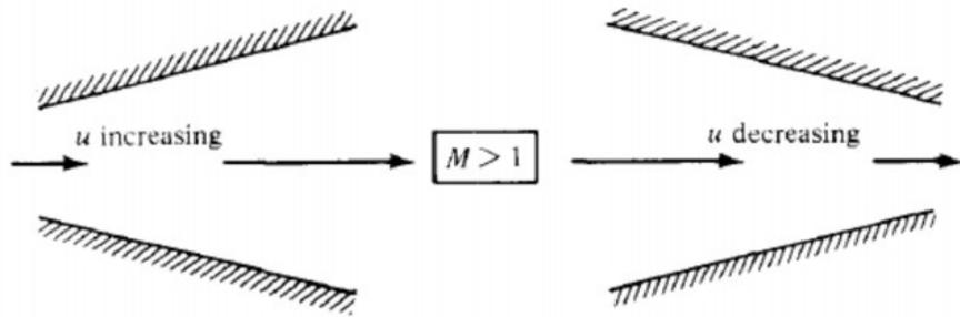
**Figure 16 Supersonic Flow in Converging -Diverging Section**
