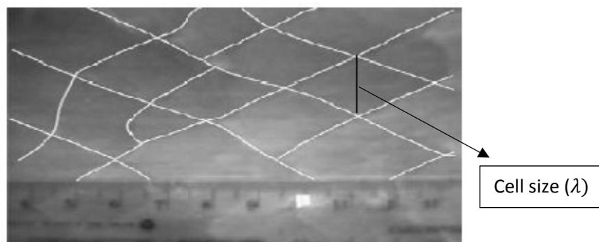
**Figure 6** "Fish scale" structure of the detonation wave (Valli & Jindal, April 2014)
