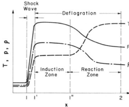
**Figure 4 Variation of physical properties for ZND conditions**
