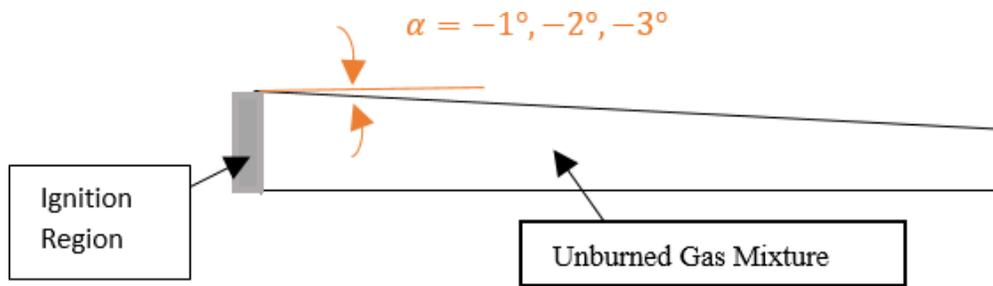
**Figure 22 PDE tube with negative angle of inclination ( $\alpha$ )**
