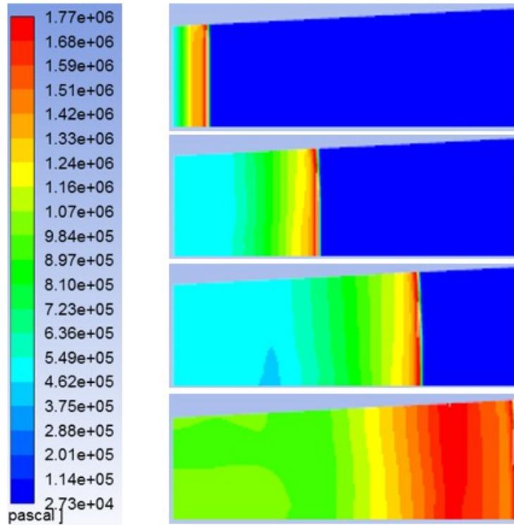
**Figure 28 Detonation wave propagation along the PDE tube with positive inclination showing pressure contours**
