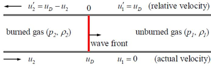
**Figure 2 Detonation wave in constant area tube**
