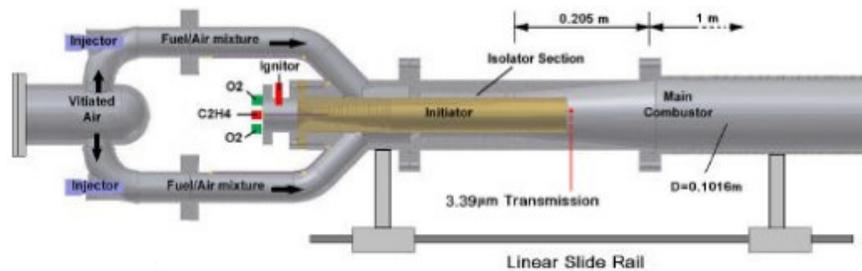
**Figure 15 Schematic of a Valve-less PDE setup**
