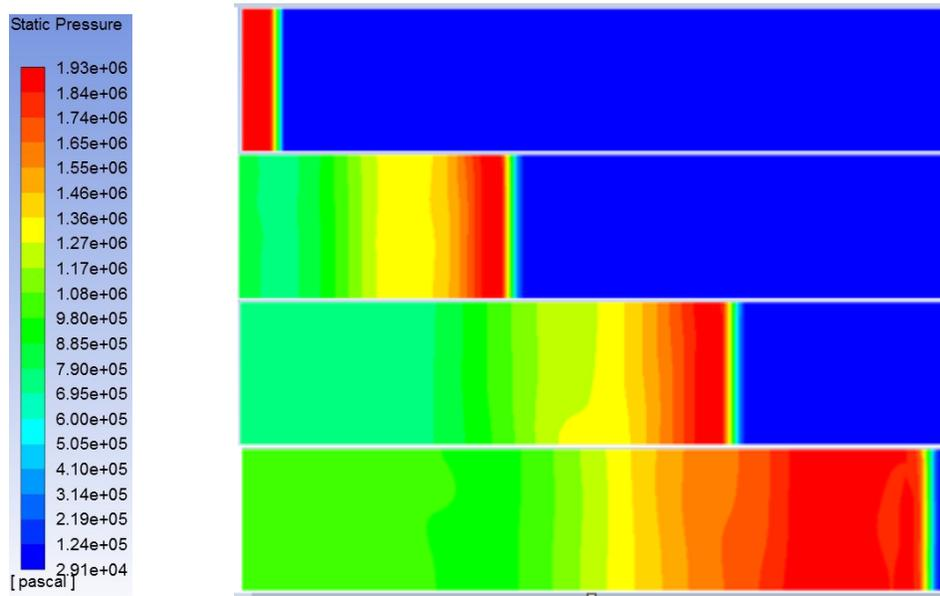
Figure 25 Detonation wave propagation along the ideal PDE tube with Pressure contours
