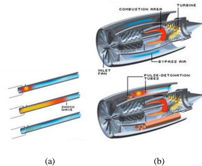
**Figure 10 PDE- hybrid gas turbine engine (a) detonation wave propagation in tube, (b) placement of detonation tubes**
