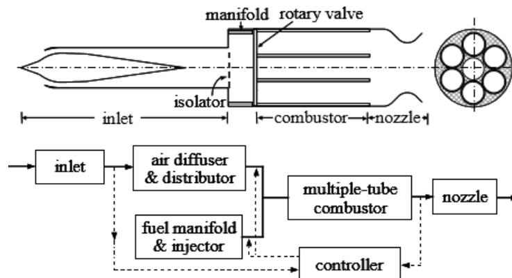
**Figure 13 Schematic of supersonic air-breathing PDE**
