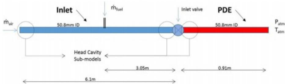
**Figure 14 Computational PDE model with dimensions (including choked inlet, intake tube, and constant fuel mass flow)**
