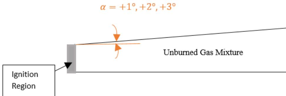
**Figure 21 PDE tube with positive angle of inclination ( $\alpha$ )**
