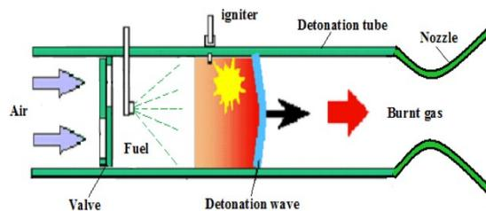
**Figure 9 Structure of PDE concept model**
