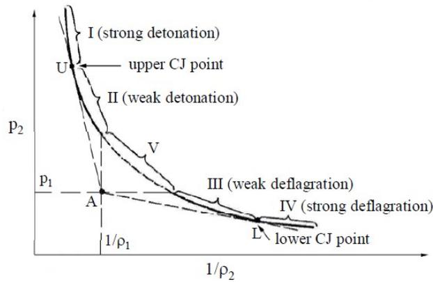
**Figure 3 Rayleigh line - Hugoniot curve PV diagram**
