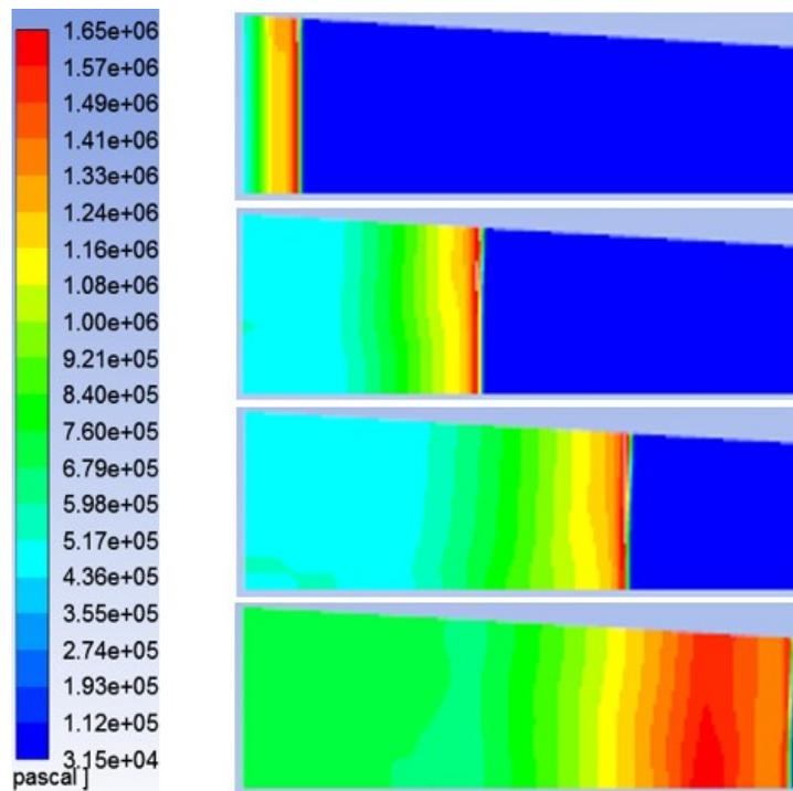
**Figure 29 Detonation wave propagation along the PDE tube with negative inclination showing pressure contours**
