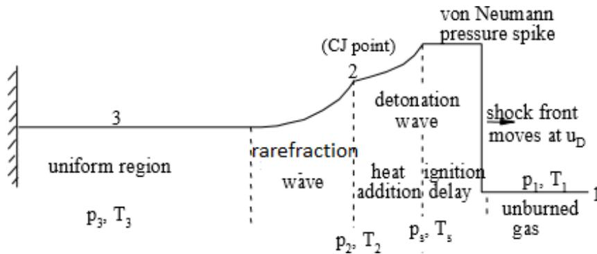
Figure 7 ZND Pressure Profile within the detonation tube
