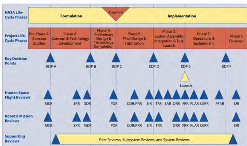
Figure 2.6: Systems engineering project lifecycle required reviews. For large projects, especially flagship-class, every review is required to be completed to ensure a continuation of the project [5].
