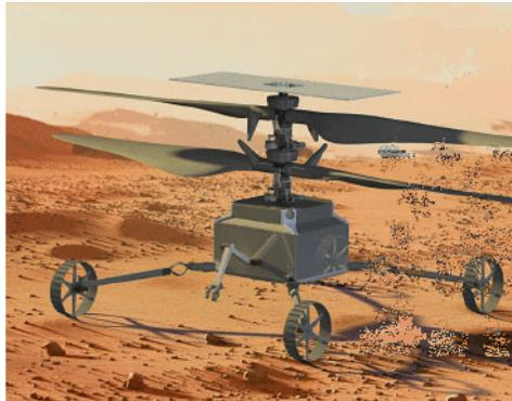
Figure 1.35: AeroVironment Sample Fetch Helicopter concept. Aside from the inclusion of a robotic arm and wheels, the helicopter design remains fairly similar.
