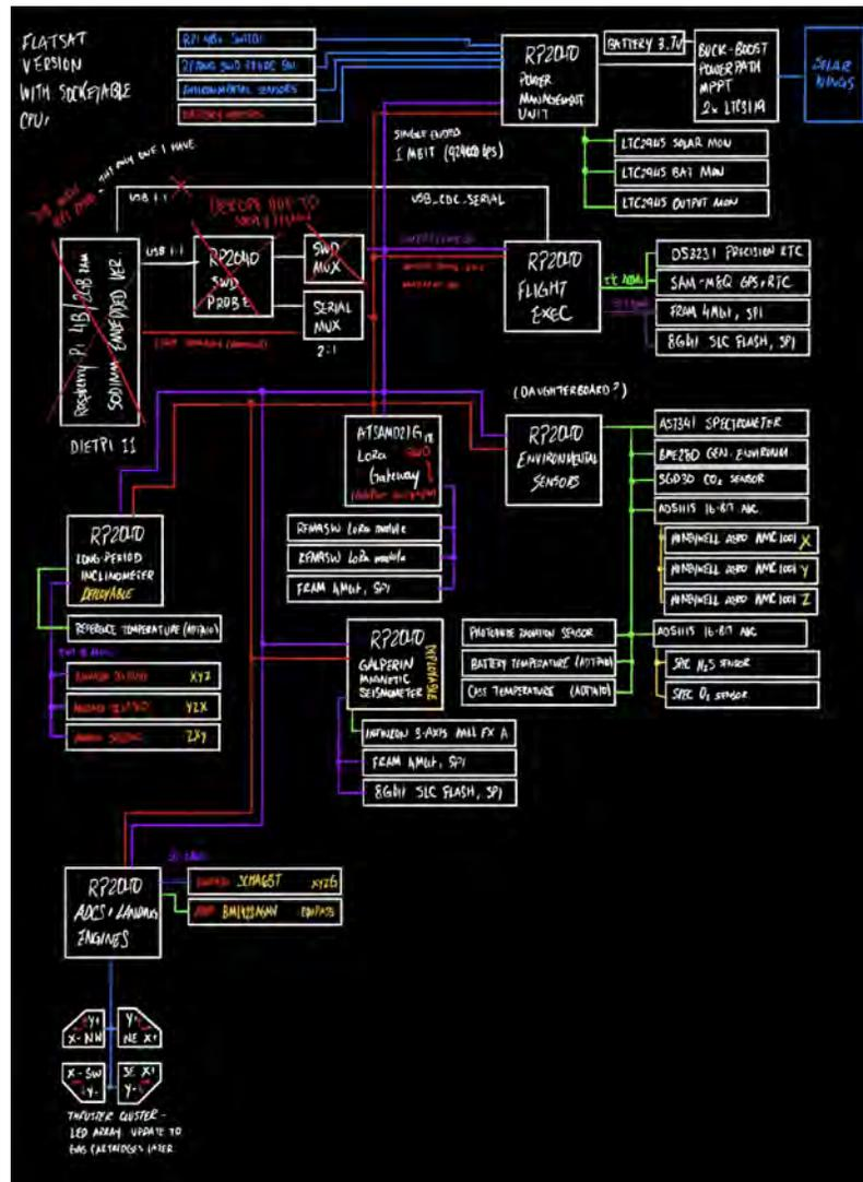
Figure 5.15: Wavefront R1 lander electronics. The prototype was meant to be breadboardable across several boards for prototyping. No propulsion system was to be a part of it; an LED quadrant simulates reaction control system thrusters.
