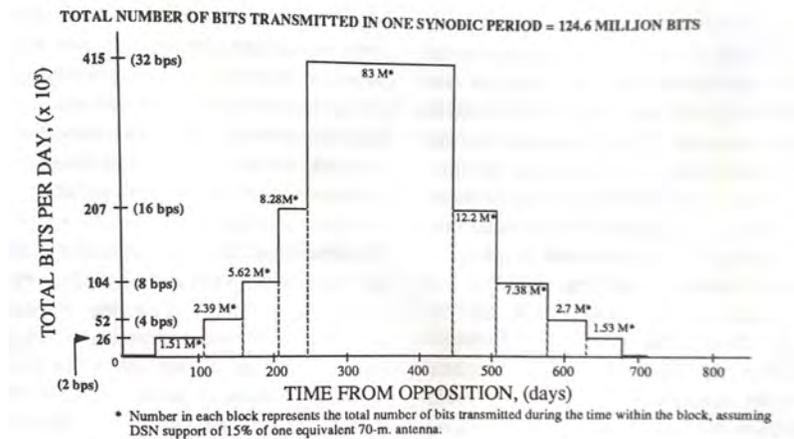
Figure 1.27: MESUR network data rate capability using 15% of one DSN 70m antenna.
