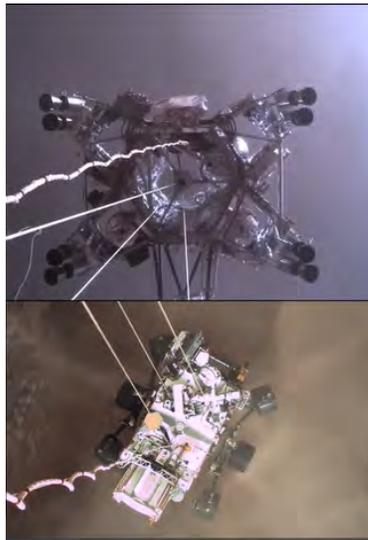
Figure 1.29: Screenshot of JPL video, replaying multiple angles of Mars 2020 while landing. The upper portion of the frame is a view from the rover looking up at the skycrane system, and the lower frame is the rover suspended from the skycrane.
