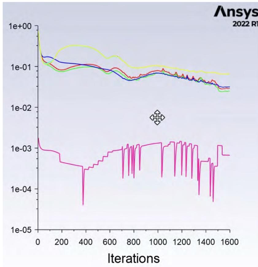
Figure 6.10: Convergence results after running the simulation with 2.997 million cells for 5 days. The stairstepping occurring in the  $\nu_t$  variable shows constant divergence protection, which is a symptom of very high gradients, poor meshing in shoulder flow, and a generally unsolved flow condition.
