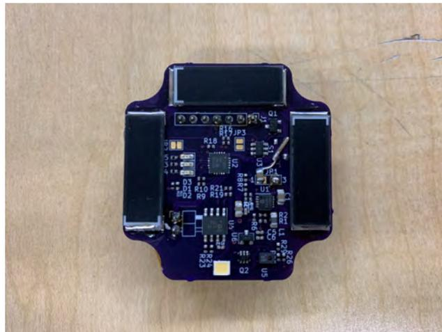
Figure 5.12: The upper stack contains the solar panels, power conditioning, and a light sensor.
