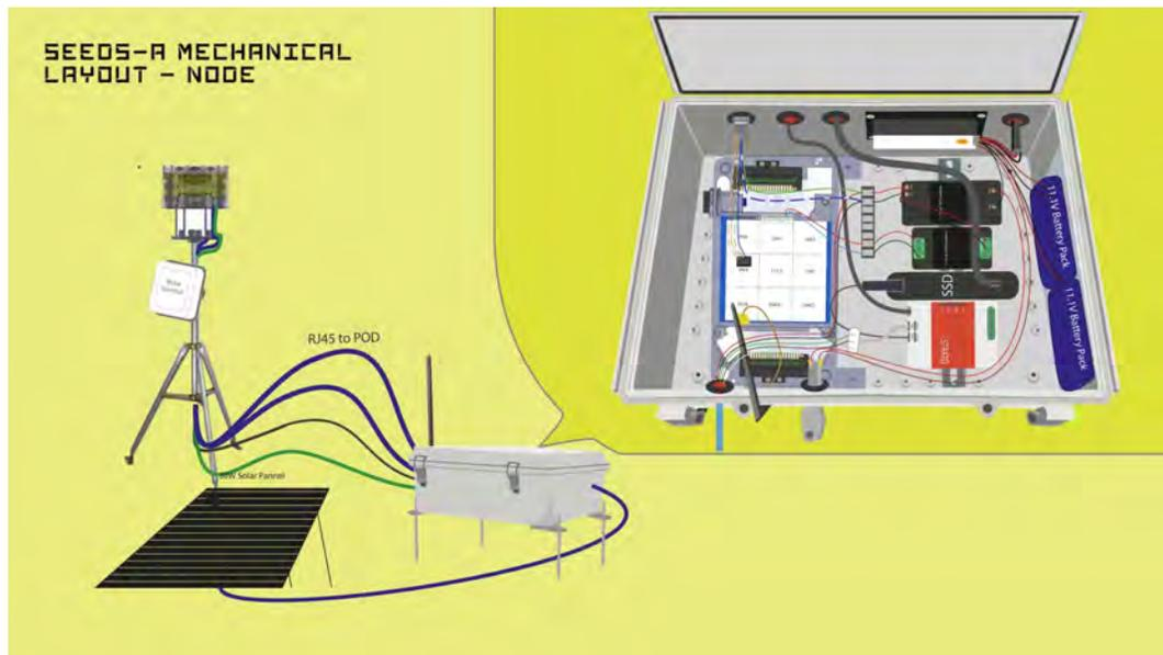
Figure 5.2: SEEDS-A mechanical configuration of *gateway*. The project used a different nomenclature that is incompatible with IoT terminology. A ground-mountable mast held the optical sensor head and Inmarsat(R) communications unit. A ground-staked polycarbonate enclosure held the electronics and mass storage. On the lower-left, a 30-watt monocrystalline solar panel powered the entire gateway. Credit: Christian Espinoza.
