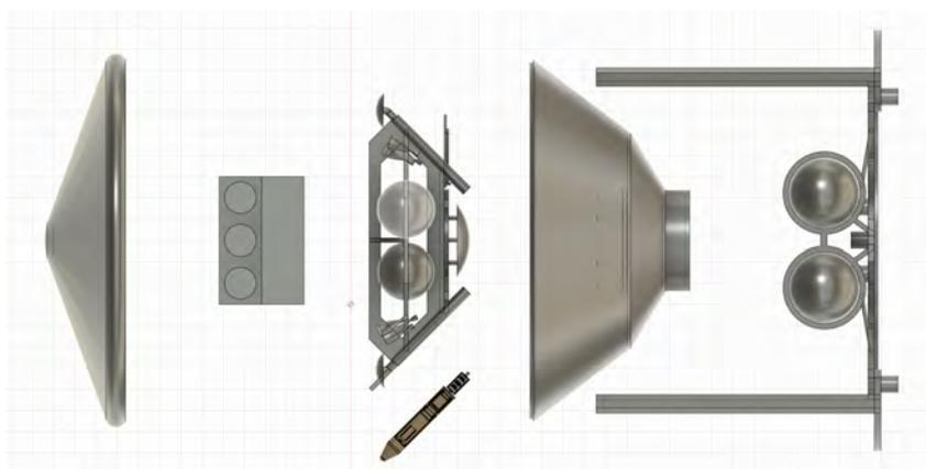
Figure 4.9: Notional, initial design for the Wavefront mission system. From left to right: 70 deg half-angle instrumented heatshield, 18U CubeSat form factor rover, ultra-light lander with base station and unrollable solar panels, Nines nanoprobes, instrumented backshell, cruise stage with stacking struts.
