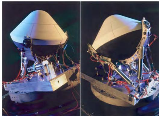
Figure 1.28: Deep Space 2 probes mounted to Mars Polar Lander bus. The heatshield was of a 45° design to accommodate its parachuteless crash landing.
