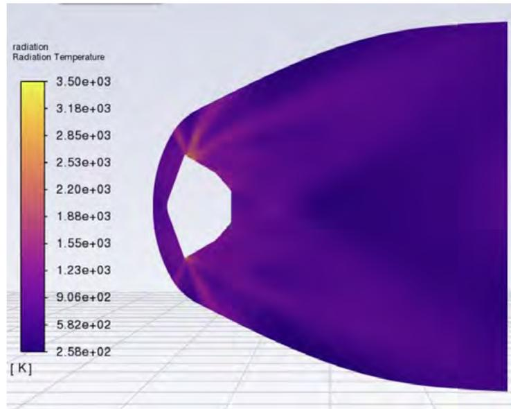
Figure 6.15: Radiation temperature response from the surface of the aeroshell.
