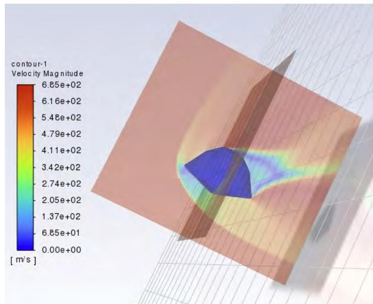
Figure 6.22: Oblique view of XZ and YZ planes of 3D flow around the aeroshell at over 40 deg AOA.
