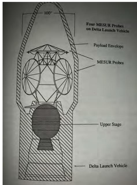
Figure 1.24: MESUR configuration inside a then-U.S. Air Force Delta II launch vehicle. Four MESUR probes are shown on a structure mounted to a solid rocket booster upper stage. The entire configuration would have fit within a 100-inch diameter. Credit: Stanley Krześniak.
