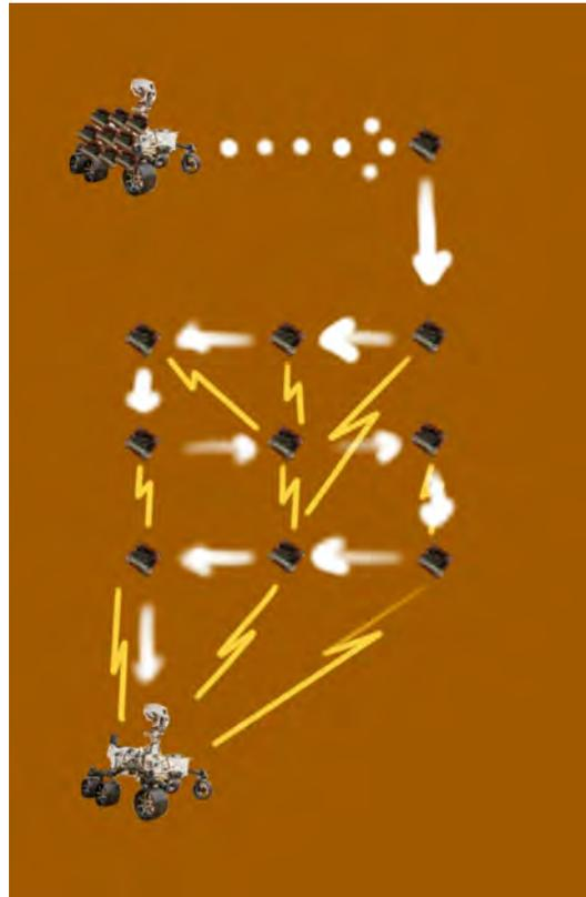
Figure 4.8: Concept of operations of Nines nodes being dropped off by a rover, one at a time. After all nanoprobes are deployed and activated, each communicate in a mesh network to eventually move the data to the rover when in range.
