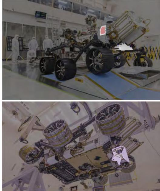
Figure 1.31: Location of RIMFAX data processing unit (top) and antenna (bottom).
