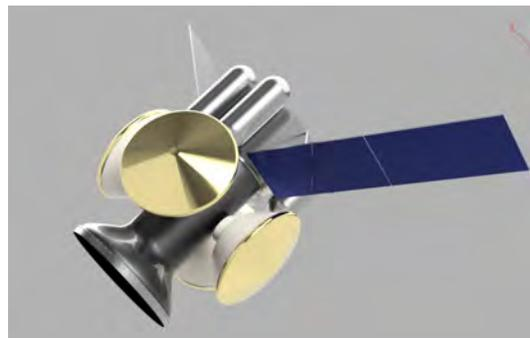
Figure 4.14: Notional, complete system design with orbital relay. Four nanoprobes landers surround the center tube, which serves as both a mounting point for all nanoprobes and relay, and extra internal space for communication equipment, including a high-gain antenna. Four external tanks surround a hexagonal prism-shaped main spacecraft body of the relay. All tanks will have a hypervelocity Whipple shield to mitigate catastrophic damage to the spacecraft during the orbital phase.
