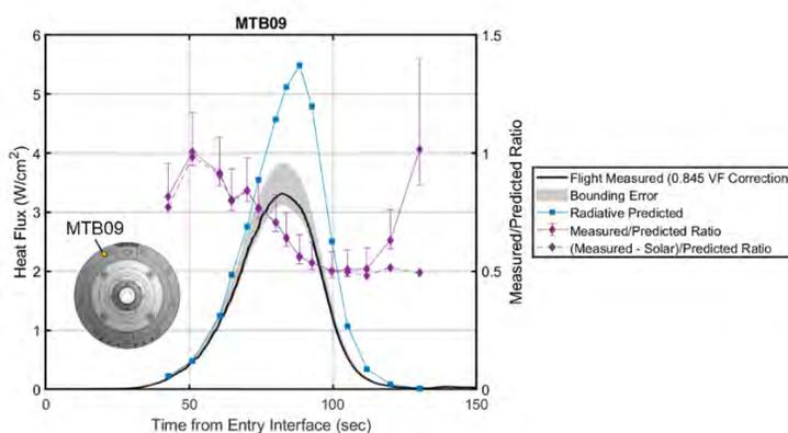
Figure 6.14: Radiative response of the surface of the MSL aeroshell.
