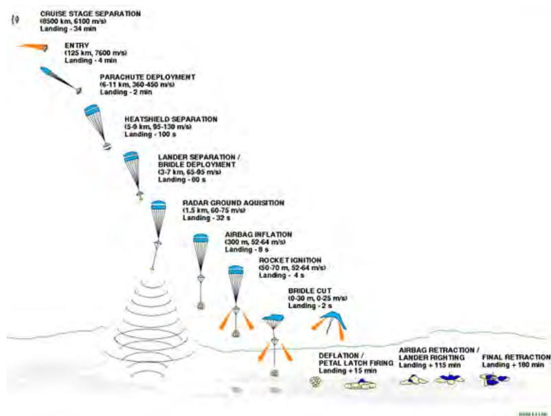
Figure 4.4: Concept of operations of Pathfinder rover mission. It is an accurate representation of a free-flyer version of Nines due to experiencing direct entry and due to the architecture being almost exactly the same. Credit: NASA JPL/Caltech/Lockheed Space Systems
