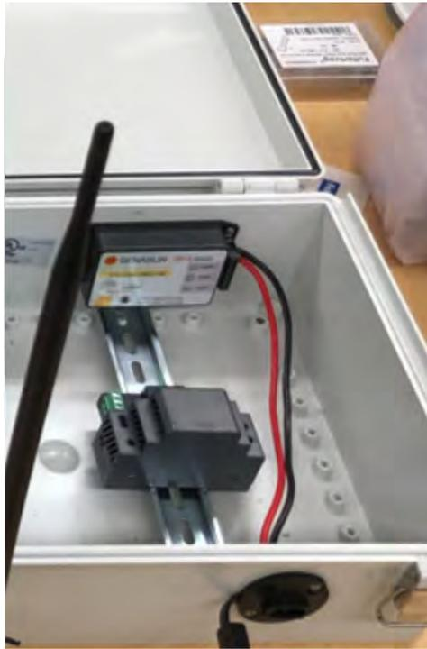
Figure 5.4: DIN rail mounting mechanism for power supplies and industrial Raspberry Pi. Credit: Stanley Krześniak
