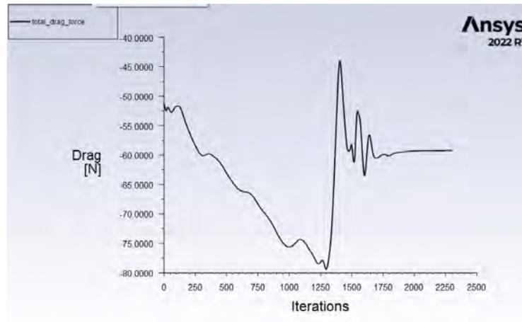
Figure 6.34: Plot of *lift* force in the XY plane. The plot is erroneously labeled as drag.
