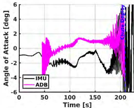
Figure 6.2: InSight reconstructed angle of attack, based on data from IMU and other factors. The black line is the direct data from the inertial measurement unit, and the pink line is from a ratio of normal and side accelerations for determination of angle of attack and sideslip, respectively. Credit: NASA JPL/Caltech.
