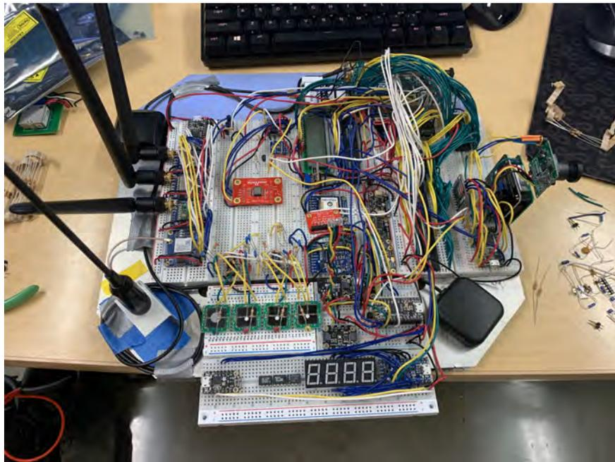
Figure 5.14: The complete gateway electronics mounted on an aluminum-2000 series honeycomb panel. The highly complex system is broken up into the following sub-systems: command and data handling, mass storage, radar evaluation and machine vision, environmental and gas sensing, debug, seismometry, and communications.
