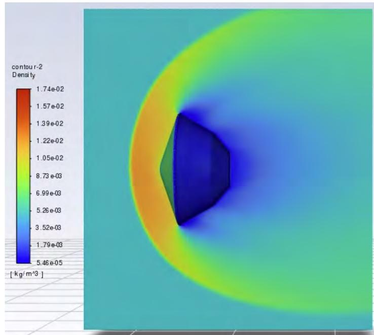
Figure 6.24: Density of flow on the YZ plane of flow around the aeroshell at over 40 deg AOA.
