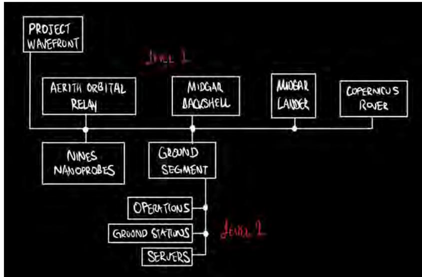
Figure 2.8: Level-1 with a single member node Level-2 product breakdown tree. Each box represents the system, subsystem, and so forth required to formulate the product. When these are fully defined, work can very easily be delegated because the chief engineer and project manager will be able to see the whole picture in terms of the project, and create an appropriately scoped WBS.
