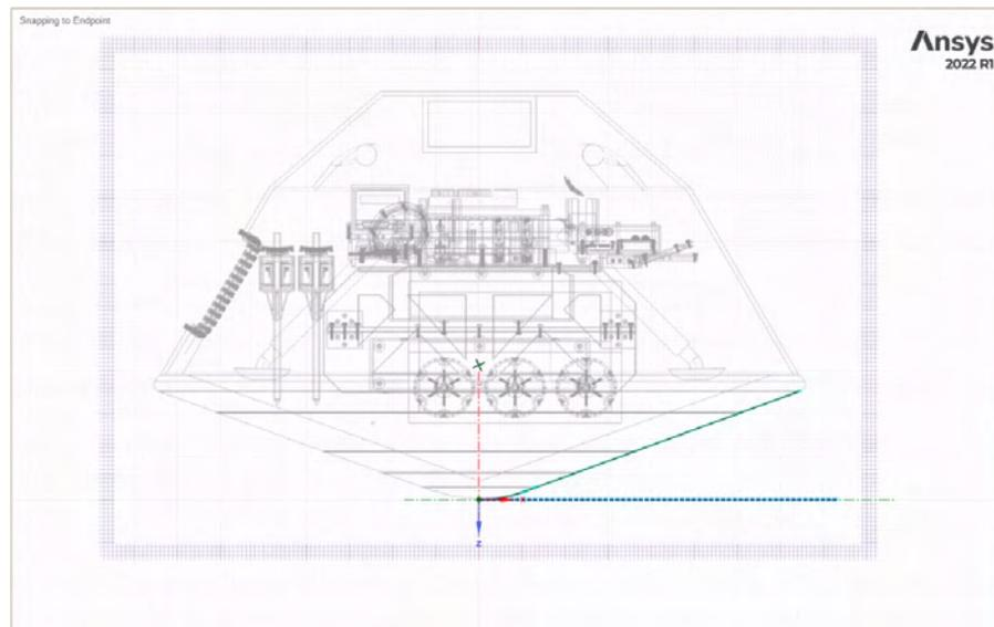
Figure 6.5: A screenshot of the SpaceClaim CAD program in sketch mode. The screenshot was scaled to the correct dimensions in order to prepare it for CFD analysis.
