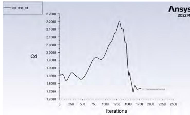
Figure 6.36: Total CD for the entire package. Convergence was observed at 1800 iterations, or roughly 3 days of wall-clock time.
