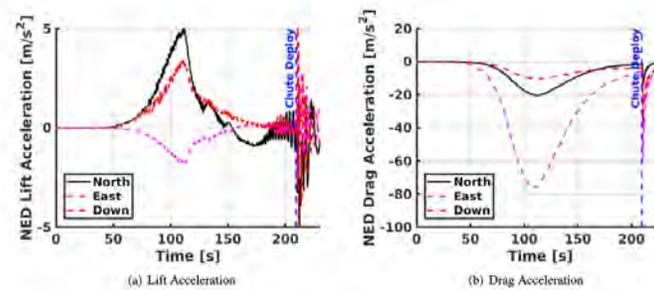
Fig. 14 Lift and Drag Acceleration Components
