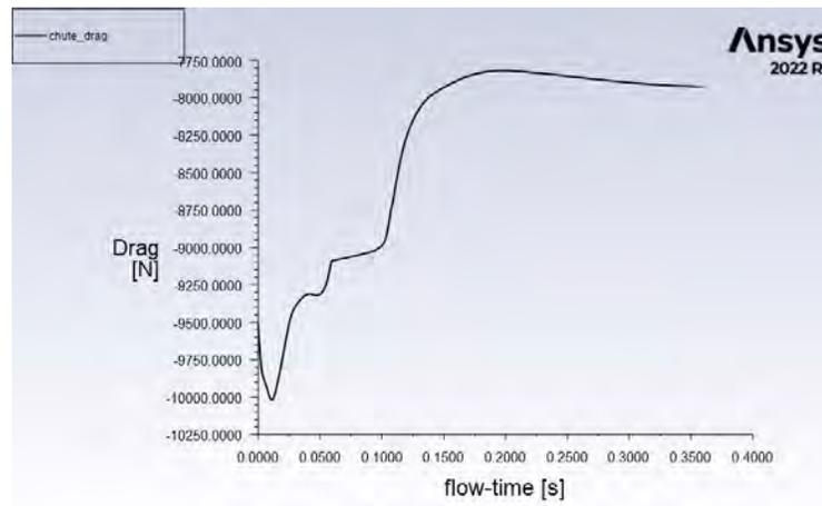
Figure 6.31: Drag in Newtons on the parachute.
