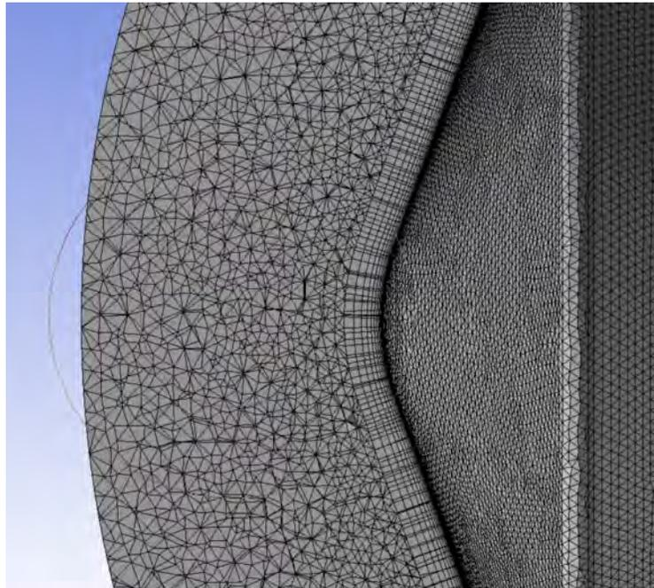
Figure 6.9: ANSYS DesignModeler (R) meshing software showing a cross-section of the blank 3D control volume for the Wavefront lander. After simulating flow, it was determined a loss of accuracy might have occurred due to part of the boundary condition intersecting the shoulders of the bow shock flow.
