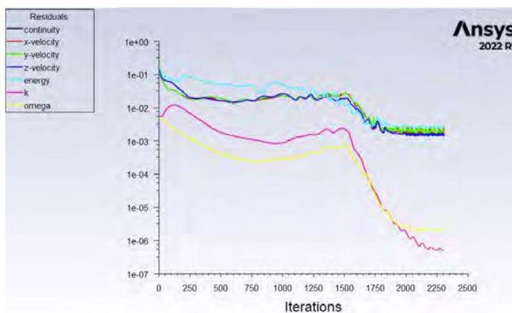
Figure 6.33: Residuals at Mach 0.16. The solution converges just above 0.1%, which is likely due to the boundary conditions being too close to the turbulent wake core of the parachute.
