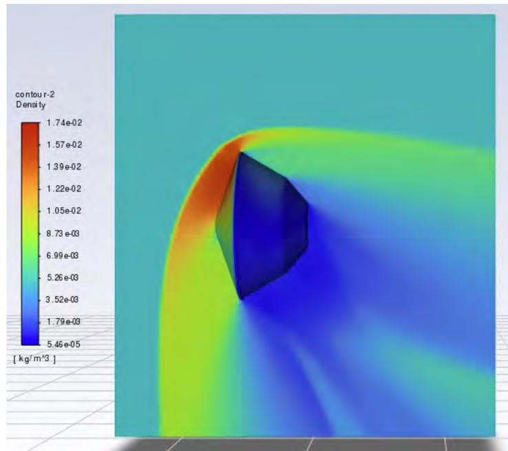
Figure 6.23: Density of flow on the XZ plane of flow around the aeroshell at over 40 deg AOA.
