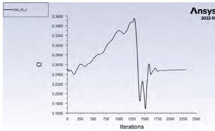
Figure 6.35: Plot of coefficient of lift in the XY plane. The initial estimate generated by FAS FMG was nearly spot-on with the final result.
