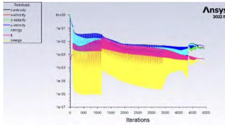
Figure 6.28: Residual plot of transient simulation. The first 100 iterations were performed at steady state to antialias the FMG solution, 150 timesteps were performed at 160 microseconds to converge the solution, and 251 timesteps were then performed at 1 millisecond once sufficiently converged.
