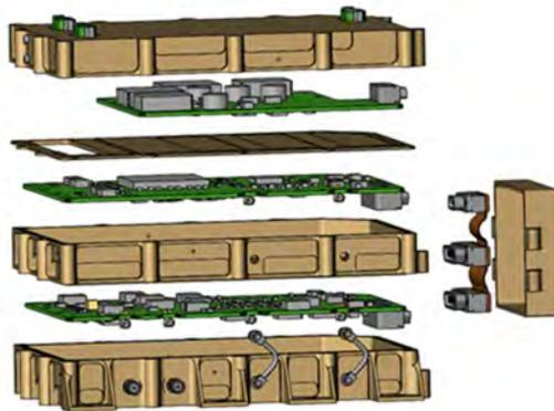
Figure 1.32: Internals and assembly of RIMFAX signal processing and conditioning.
