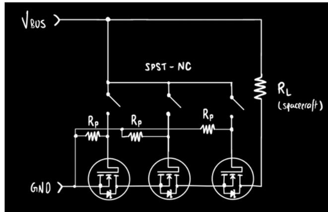
Figure 3.3: Electrical schematic for a dual-fault tolerant, electromechanical inhibit scheme. Resistor  $R_P$  is used to "pull-down" the voltage to zero, since MOSFETs behave like parallel plates - capacitors and must be discharged to properly signal. Resistor  $R_L$  is the entire spacecraft load. The switches are ahead of the spacecraft load in order to allow power to flow to the inhibit MOSFETs.
