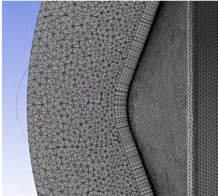
Figure 6.7: ANSYS DesignModeler (R) meshing software showing a cross-section of the 3D control volume for the Wavefront lander. This particular mesh has 2.9 million cells, with an O-type structured mesh and unstructured tetrahedral filler mesh. Note the semi-unstructured form of the O-type mesh - each layer is a hexahedral/triangular prism.
