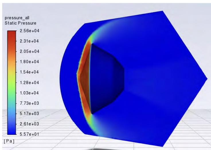
Figure 6.11: ANSYS DesignModeler (R) meshing software showing a cross-section of the blank 3D control volume for the Wavefront lander. After simulating flow, it was determined a loss of accuracy might have occurred due to part of the boundary condition intersecting the shoulders of the bow shock flow.
