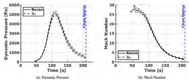
Fig. 15 Reconstructed Atmospheric-Relative Trajectory
