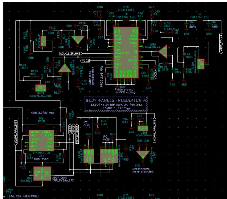
Figure 7.4: Solar wing power regulator subsystem schematic.
