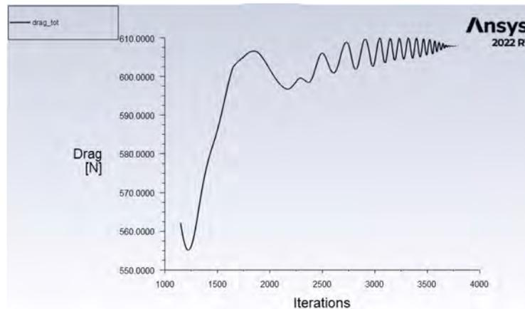
Figure 6.21: Aerodynamic convergence plot for Mach 2.1.
