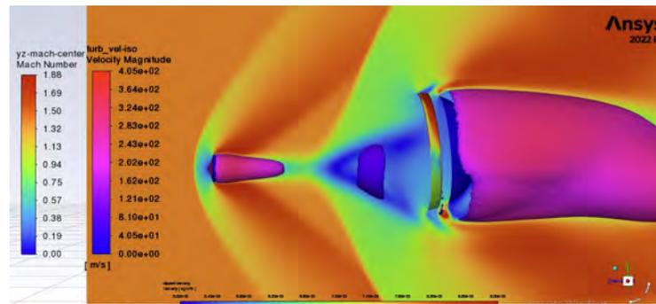
Figure 6.32: Mach 1.4 scene at 331.4ms flow time.
