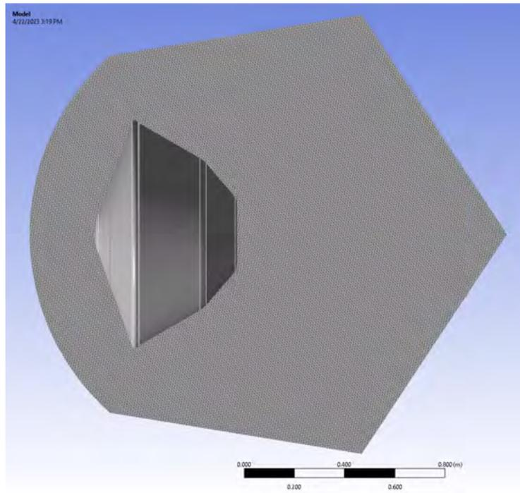
Figure 6.8: ANSYS DesignModeler (R) meshing software showing a cross-section of the blank 3D control volume for the Wavefront lander. After simulating flow, it was determined a loss of accuracy might have occurred due to part of the boundary condition intersecting the shoulders of the bow shock flow.
