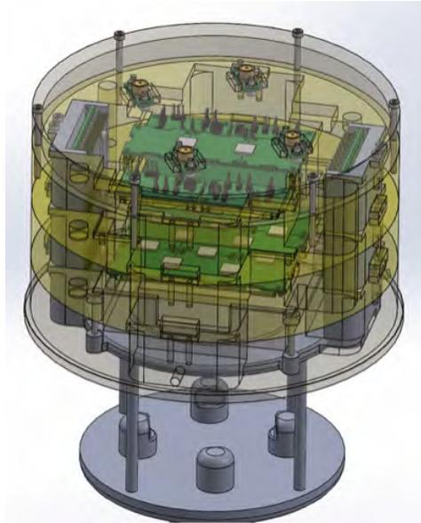
Figure 5.5: Sensor head CAD with internals shown. The optical sensor head was designed to be mounted on top of a Windsonic(R) ultrasonic wind sensor. Credit: Stanley Krzeńskiak
