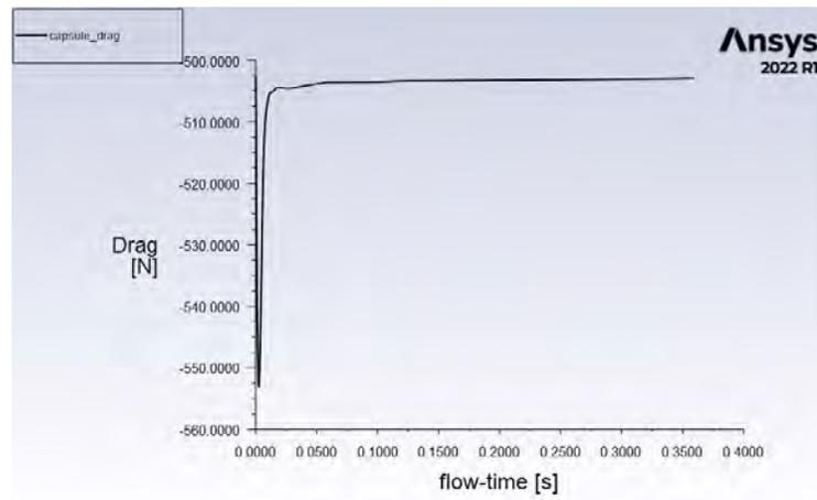
Figure 6.30: Drag in Newtons on the aeroshell.
