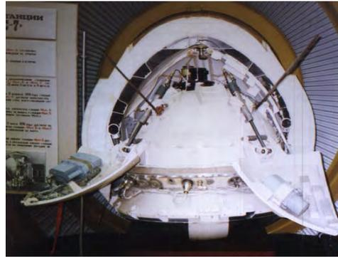
Figure 1.14: A cutaway of a full-scale model of the Mars 3 lander, on display at the NPO Lavochkin Museum. Credit: Alexander Chernov.
