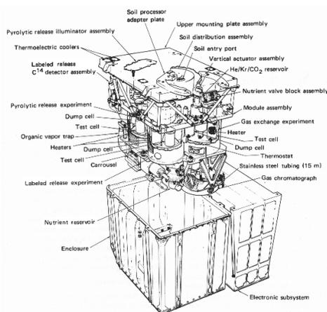
Figure 1.16: A detailed drawing of the Viking Biological Package, an experiment specifically designed to determine if life was present on Mars. Credit: NASA.
