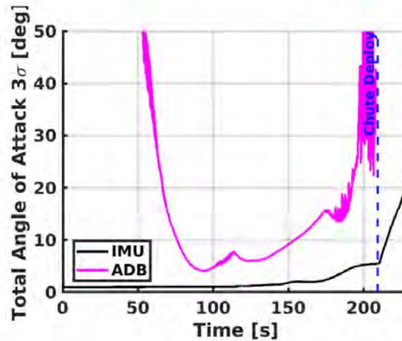
Figure 6.3: Reconstructed angle of attack, with 3-sigma error bounds. Credit: NASA JPL/Caltech.
