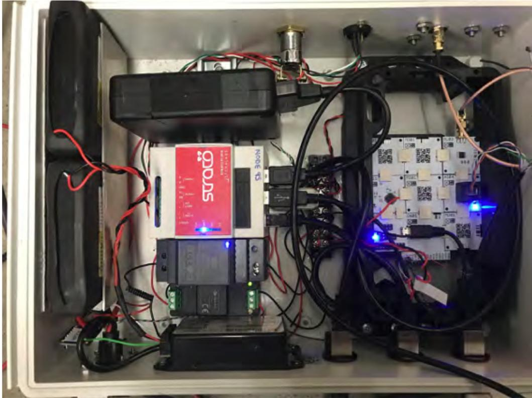
Figure 5.3: SEEDS-A internal mechanical configuration of *gateway*. From left to right: 3S2P, lithium-ion, 200 watt-hour; 128 GB SLC SSD; Raspberry Pi 3B+; 12V buck regulator; 3.3V buck regulator; 27V MPPT solar to battery charger; terminal block; modular central computer. Credit: Stanley Krzeńskiak
