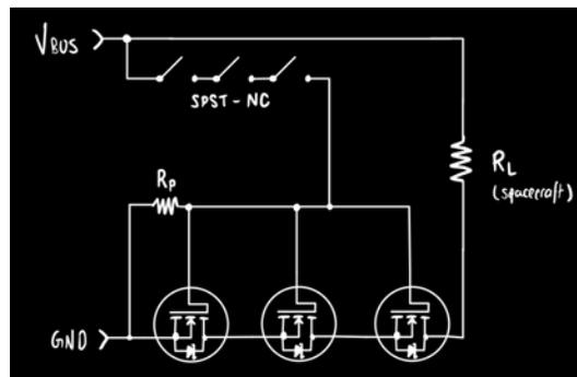
Figure 3.1: Electrical schematic for a dual-fault tolerant inhibit scheme.
