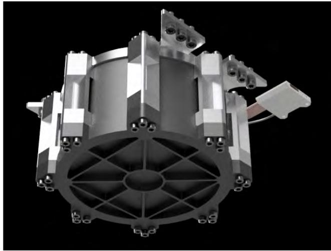
Figure 4.11: Shinra Radioisotope Thermoelectric Generator for nuclear lander option, which was ultimately not selected.
