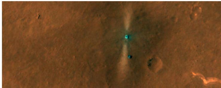
Figure 1.39: The Zhurong rover and lander system on the surface, imaged by NASA JPL's Mars Reconnaissance Orbiter. The blast pattern from the descent engines of the lander are shown. To the right of the lower blast pattern is the Zhurong rover. Credit: NASA/JPL-Caltech/Arizona LPL.
