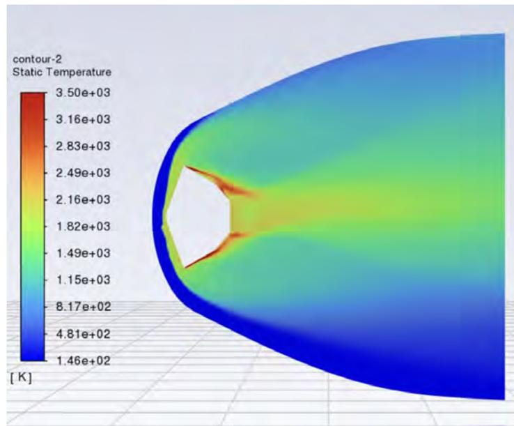
Figure 6.16: Radiative response of the surface of the MSL aeroshell.
