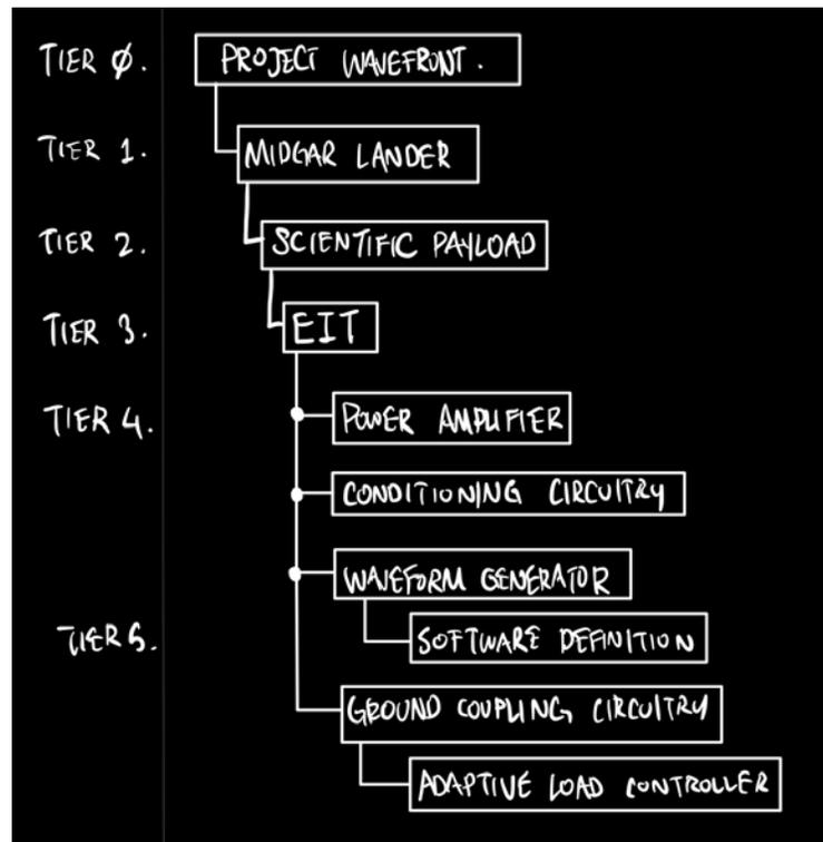
Figure 2.9: Representative Level-5 product breakdown for impedance transmitter on electrical impedance tomography instrument of individual Midgar lander. Because of the distributed nature of this instrument, this is not a complete PBS of the EIT instrument. Aside that, the very high tier numbering shows how much engineering would have to be considered as part of the system, which significantly increases the number of engineers required for this stage of the project.
