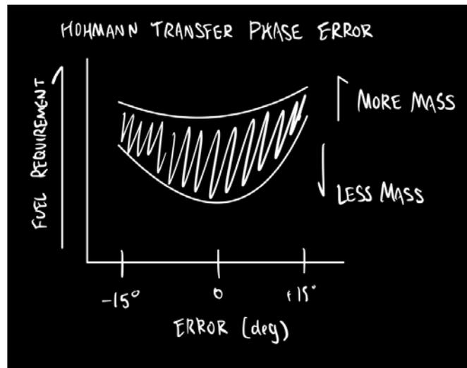
Figure 3.4: A basic tradeoff of the phase error between an ideal Hohmann transfer and the fuel requirement. The space in between the upper and lower lines represent an acceptable mission. In orbital dynamics, derivatives of this plot are called "porkchop plots", due to the shape of the area within the curves forming a porkchop.
