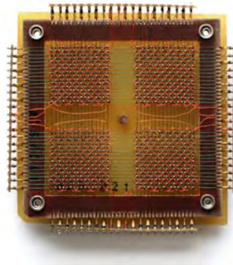
Figure 1.2: Core rope memory module storing 1024 bits. Credit: Wikimedia Foundation.
