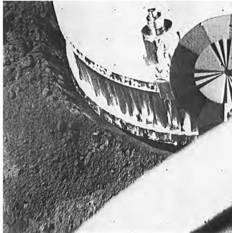
Figure 1.6: A picture of Surveyor 1's foot pad from its zoomable television camera. The softness of the regolith is visible. Credit: NASA/Jet Propulsion Laboratory.
