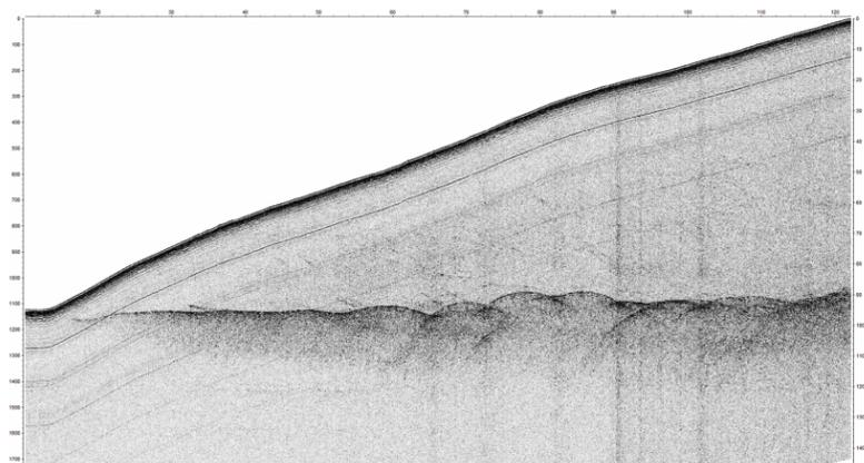
Figure 1.33: RIMFAX instrument test results at the Midtre Lovenbreen glacier in Svalbard, Norway. The solid, near-diagonal line is the surface, and features under it show different properties of the ice and water below the glacier. The strong, horizontal return is the "grounding line", where the ice meets rock. Credit: University of Oslo.
