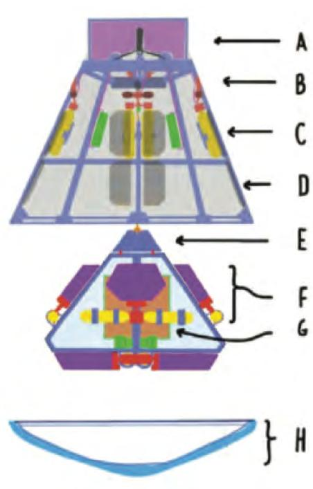
Figure 4.3: 2D drawing of the full Nines concept. The backshell (A-D) contains propellant (C), batteries (D), the parachute (A), and high speed deceleration devices (B). The tetrahedron (E-G) contains the actual lander hardware (G) and self-righting lander petals (E), as well as airbags and airbag inflators (F). The heatshield (H) is at the bottom, which would be 3D printed using ablator and PAEK-based thermoplastics.
