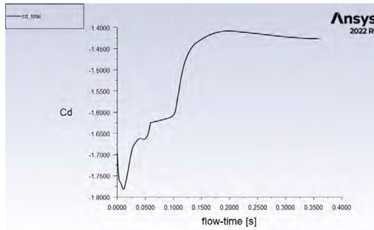
Figure 6.29: Total coefficient of drag on the capsule-parachute system.
