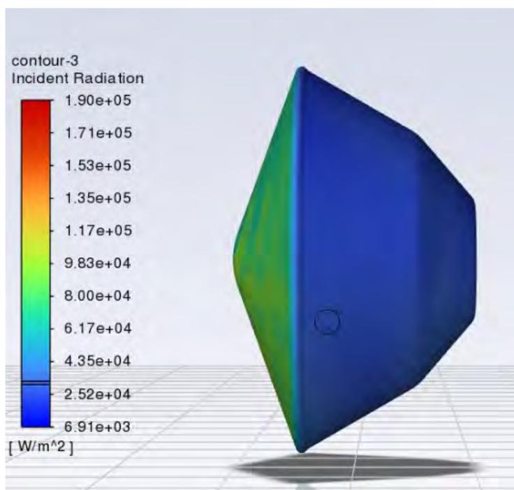
Figure 6.13: Radiative response of the surface of the aeroshell. The circle (reticle) on the backshell corresponds to Figure 6.13's MTB09 radiometer response.
