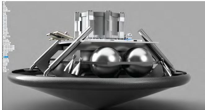
Figure 4.12: Shinra RTG mounted on lander, showing the extensive amount of volume it occupies.
