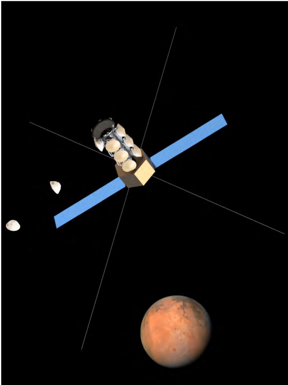
Figure 4.15: Aerith releasing two Midgar landers at apoapsis. By releasing the landers at apoapsis, fine-tuning the landing site by the lander's limited fuel supply is maximized.
