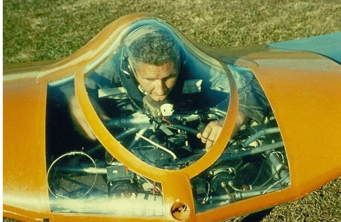
**Fig. 4 Picture of Horten IV aircraft and pilot position [6].**
