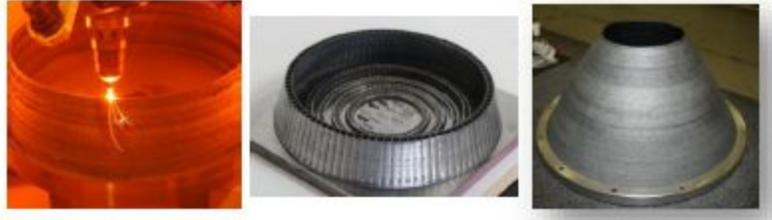
Figure 1.3 - Blown powder deposition [4]
