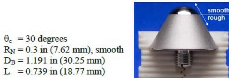
Figure 1.15 - Base geometry parameters from Reda [15]
