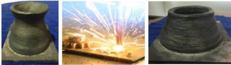
Figure 1.5 - Arc-based deposition [4]
