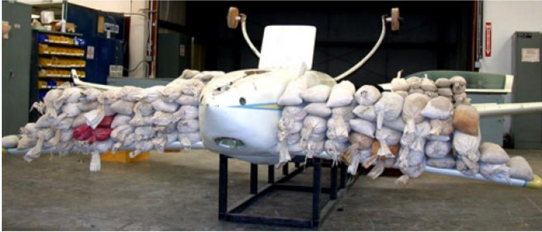
Figure 3-3: Applying Sandbags
