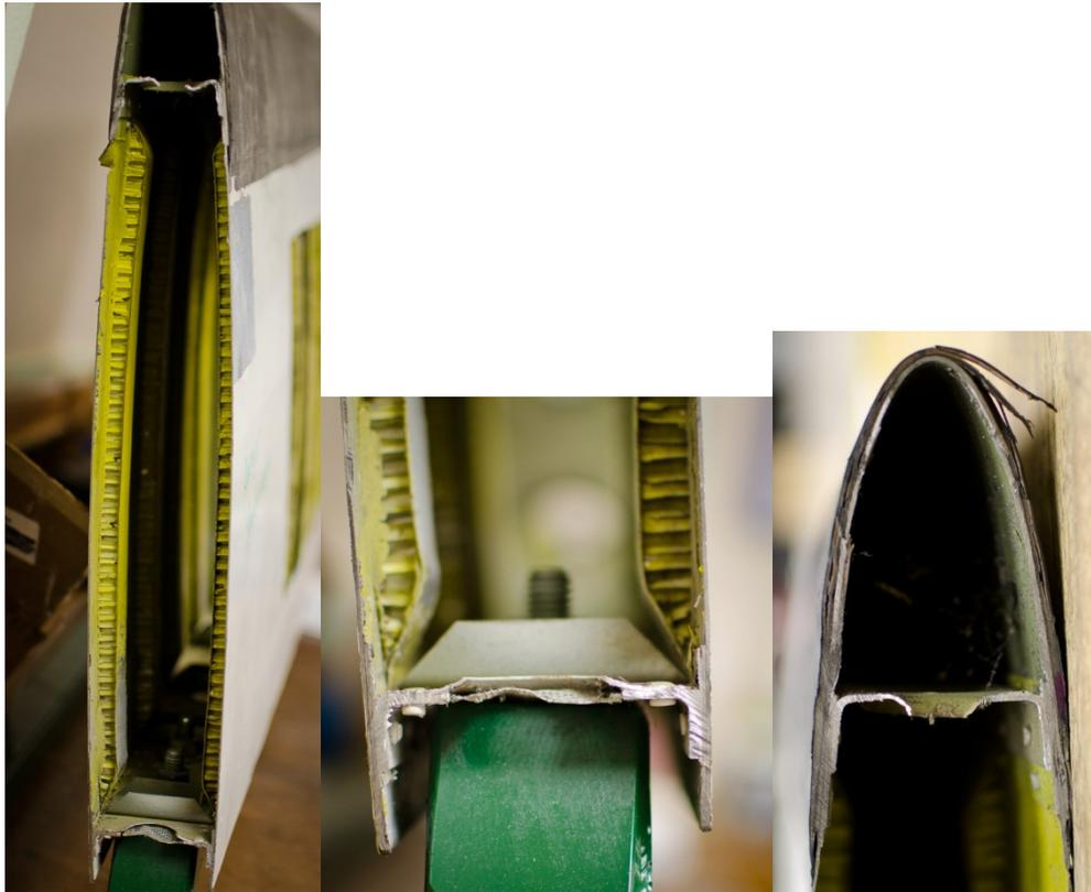
Figure 3-13: (a) (b) (c) Observed Cross Section of the Tail Section
