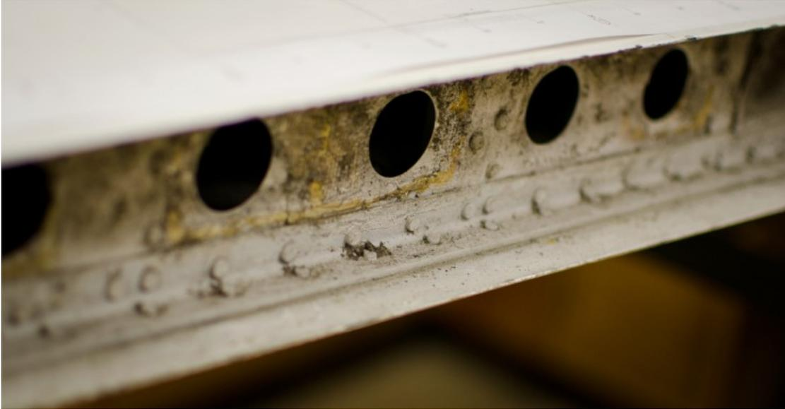
Figure 3-14: Stringers along the wing and the Backing Support with Cutout Holes
