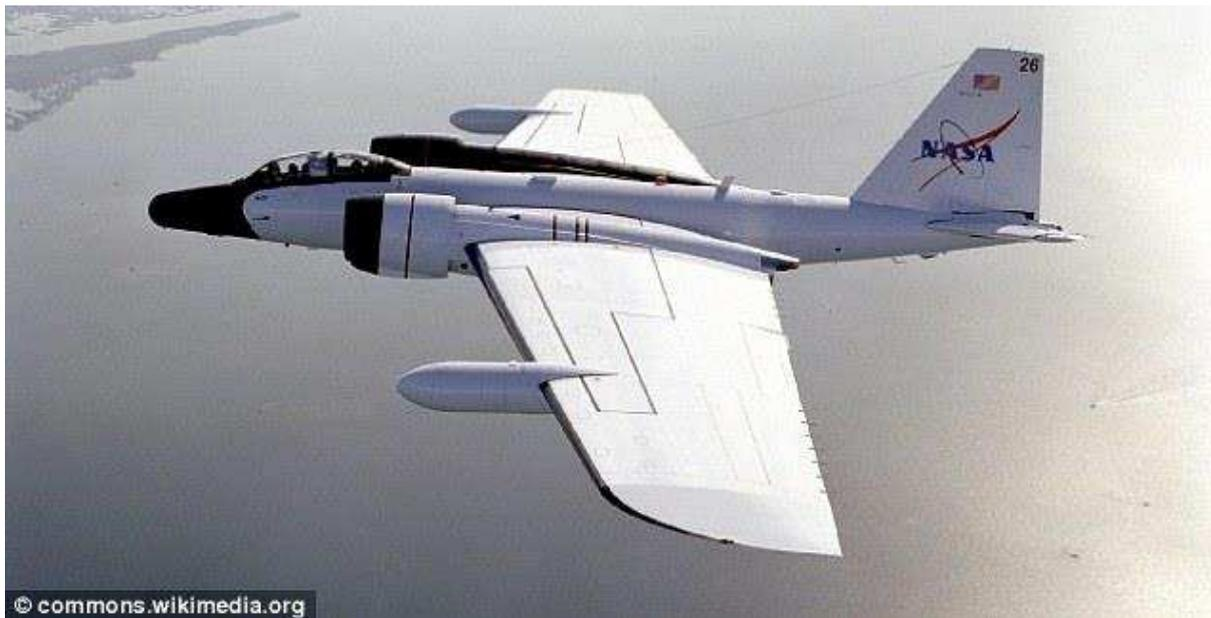
*Figure 145: Mid Wing Configuration -NASA Research Plane*
