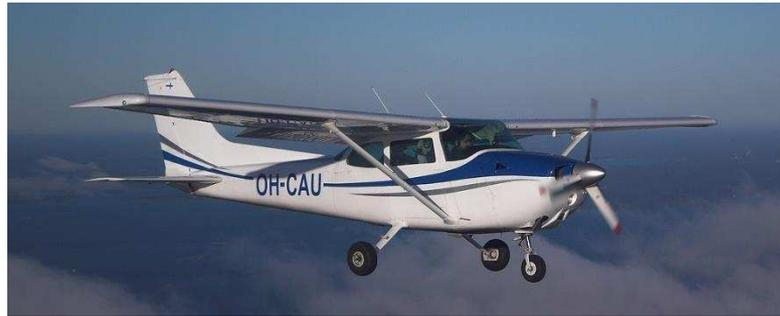
*Figure 143:High Wing Configuration - Cessna 172*
