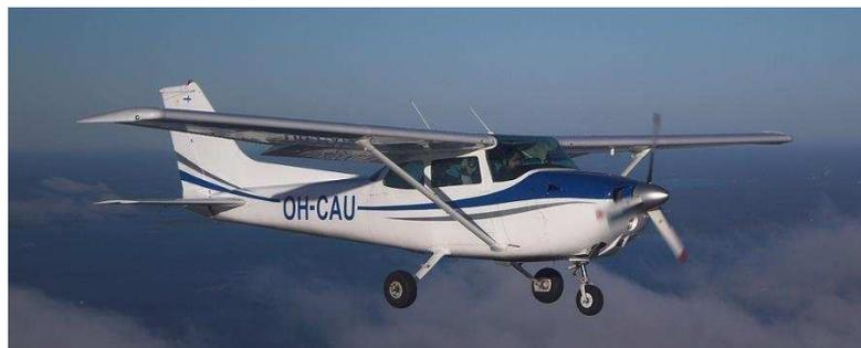
*Figure 13:High Wing Configuration - Cessna 172*
