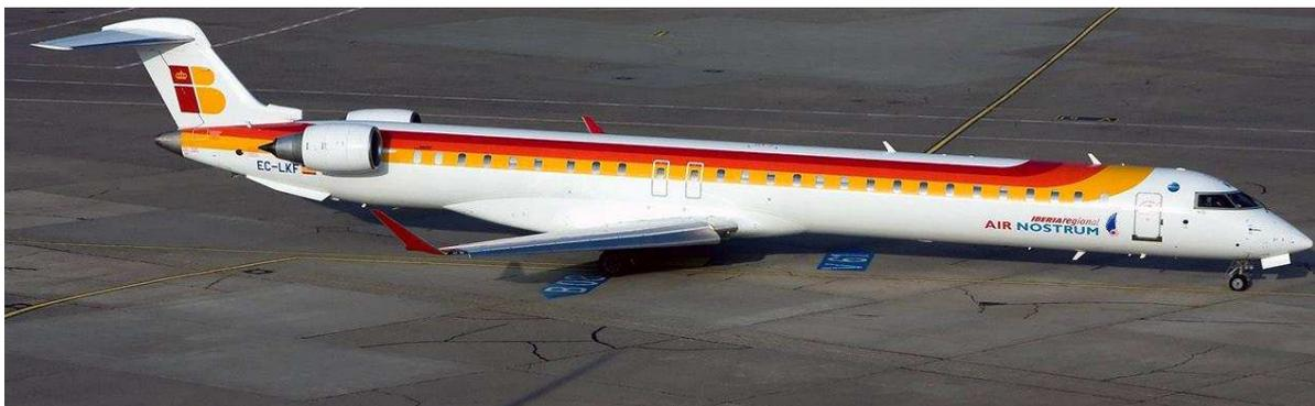
*Figure 144: Low Wing Configuration -CRJ1000*
