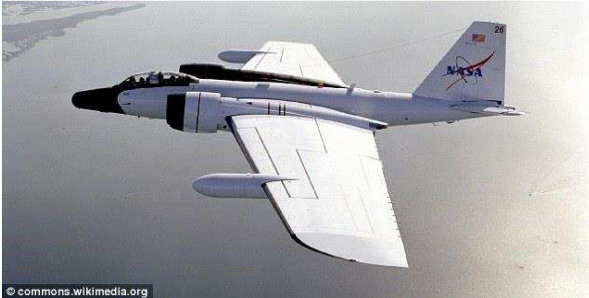
*Figure 15: Mid Wing Configuration -NASA Research Plane*
