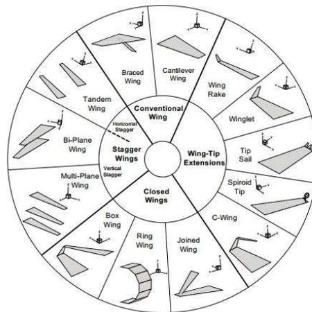
*Figure 7: Conventional/Unconventional Wing Structures*
