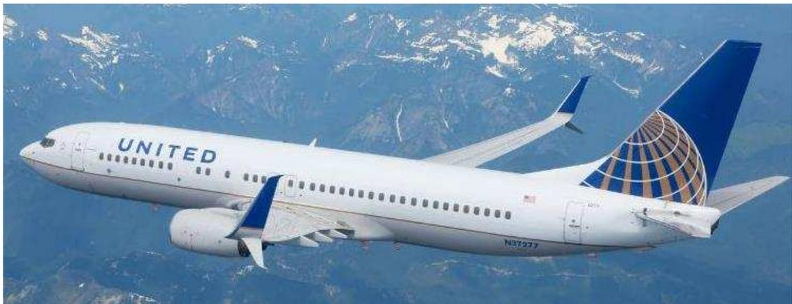
*Figure 157: United Airlines Boeing737 Winglets located at Wing tips*
