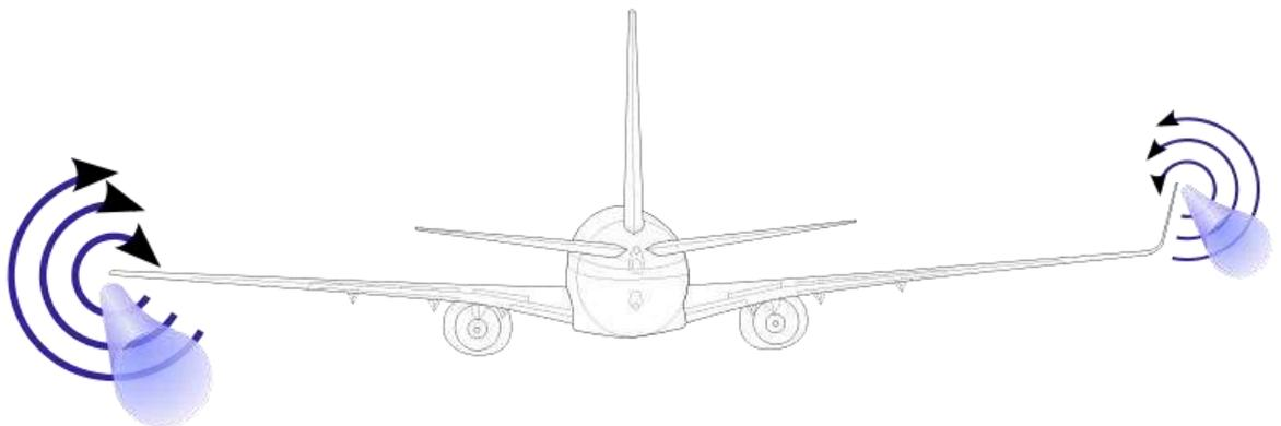
*Figure 158: Wing Tips with and Without Winglets*
