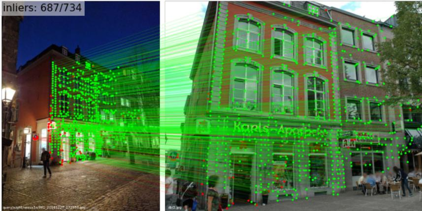
Figure 5.5 – Keypoint feature matching between two images [29].
