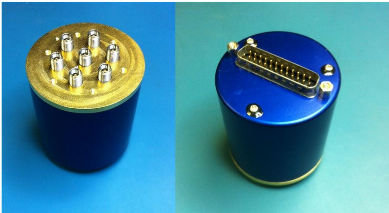
**Figure 4.1-1: Radiall R583833250 Switch**
